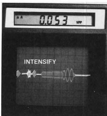
Fig. 16 — Intensify the color burst with the Delta PPV function. Notice, it is 53 mV which is outside the recommended tolerance.
