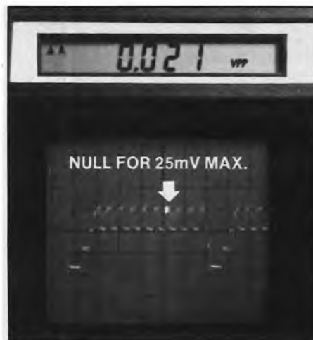
Fig. 9 Null the trap until the SC61 reads under 25 mV. Job done!
