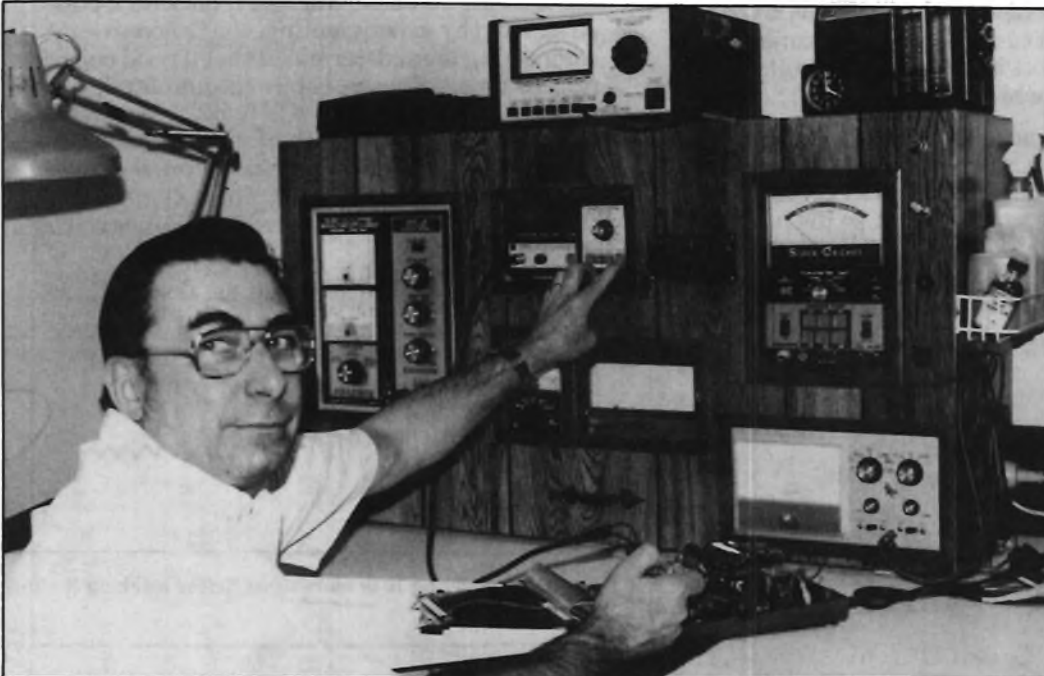
The Sencore leakage and dielectric absorption test finds defective capacitors in the power supplies and eliminates digital glitches.
