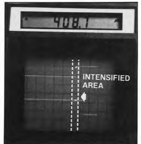
Fig. 12 — Now adjust the bar for less than a 440 uS readout, as we've done here.
