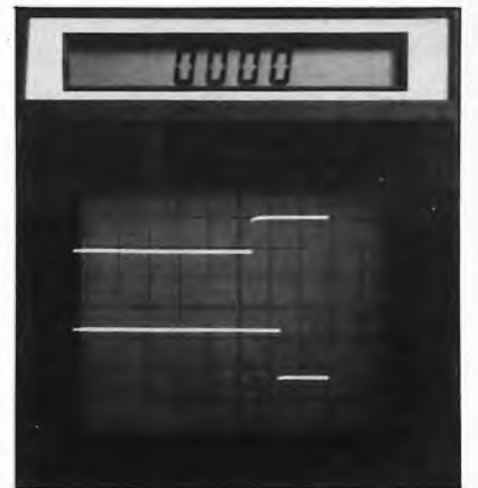
Fig. 10 — Use the CRT to view the two servo waveforms as shown in the service literature.
