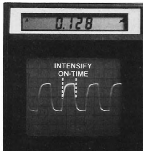
Fig. 19 — Use the digital display to confirm the setting is correct by measuring the on-time with the Delta Time function.
