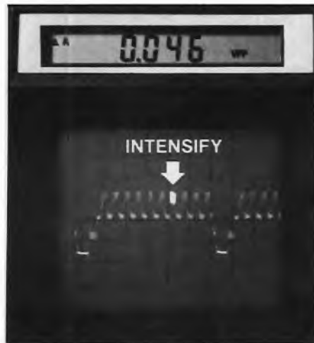
Fig. 8 — Intensify the top of one color bar to measure the amount of color signal at the trap output. Here, the signal is 46 mV which is above the 25 mV limit.
