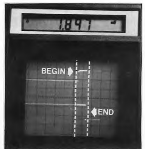
Fig. 11 — Adjust the Delta Time bar until it fills the delay between the two signals that we want to measure and we see the signals are 1.897 mS apart, which is outside the 440 uS limit.
