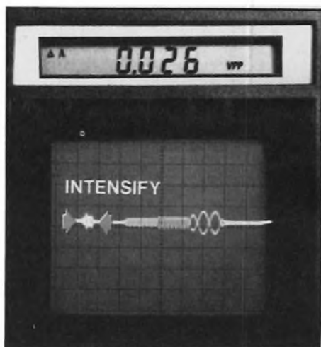
Fig. 17 — Adjust the circuits until the digital readout shows the correct amplitude of 25 to 30 mV.
