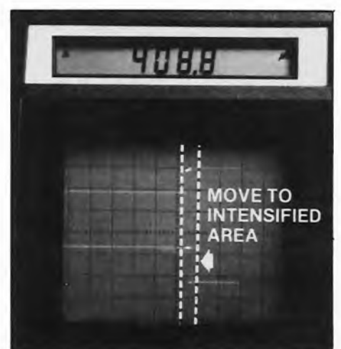
Fig. 13 — Simply adjust the control until the two signals fall inside the Delta bar. The entire operation takes only seconds.
