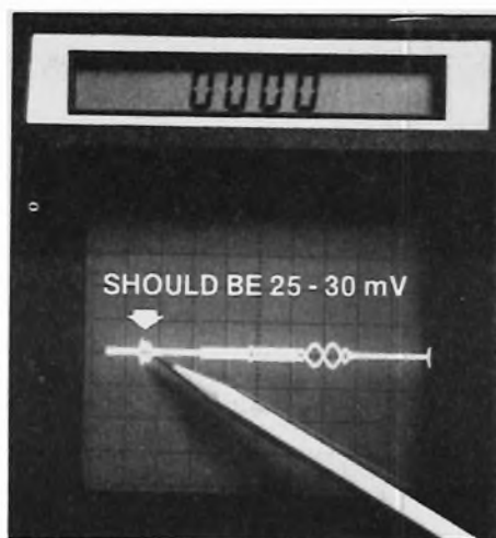
Fig. 15 — The chroma record current adjustment requires the color burst to be between 25 and 30 mV, according to the RCA procedures.
