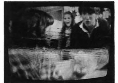
Fig. 3 — Timing errors in the servo circuits cause increased video noise or tearing in the picture during playback.
