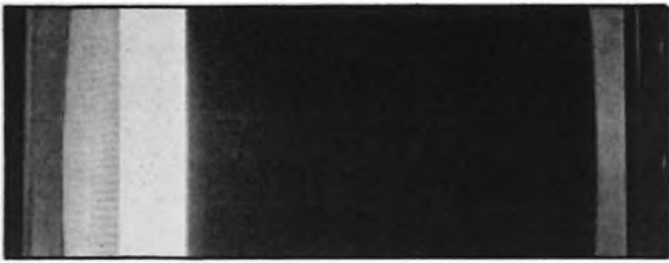
Fig. 17—You can set the screen and drive controls dynamically with the grey scale portion of the Bar Sweep pattern.
