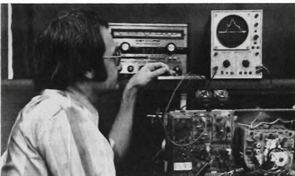
Fig. 3—The bias supply must be used because a sweep and marker signal is totally unnatural to the keyed AGC circuits. The bias supply setting will affect the response curve.
