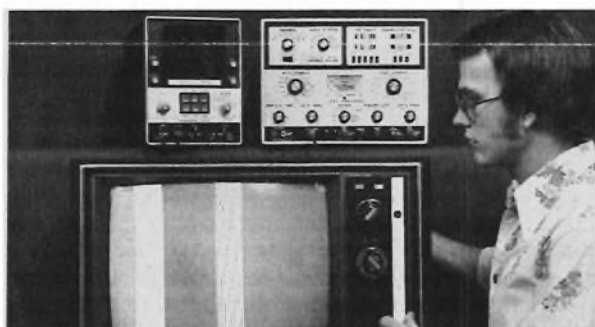
Fig. 8—Use your VA48 for "spot alignment" by selecting the one bar whose frequency is closest to the frequency called out in the alignment instructions and adjusting for maximum.
