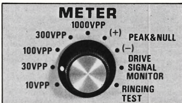
Fig. 31—The Drive Signal monitor position of the meter lets you set the level of drive signal to match the circuit.
