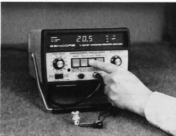
Fig. 17 — The "Z METER" provides an automatic inductance value test and Ringing "Q" test to locate problems in coils and transformers.
