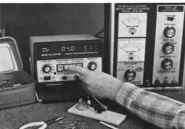
Fig. 6 — Ceramic capacitors that change value due to thermal stress can cause real headaches for circuit designers. This one changed from 19 pF to 4 pF during a standard temperature test.
