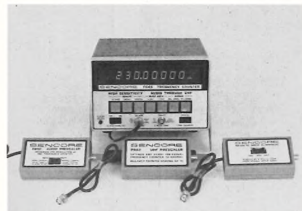
Fig. 1 — The FC45 counting system allows you to update your counting capabilities at any time with two optional prescalers and a digital noise filter for use in PLL troubleshooting.
