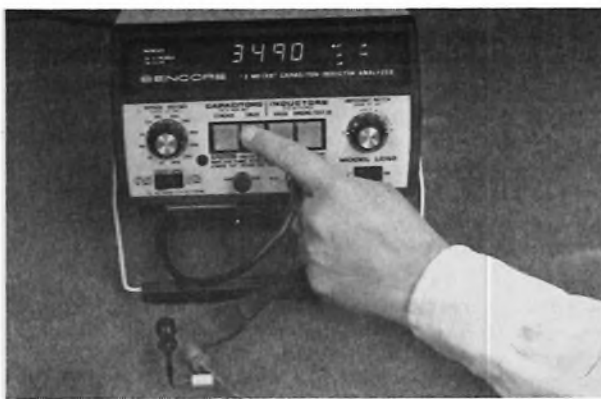
Fig. 3 — The "Z METER" is so simple to operate, just connect the capacitor and push the button to get the capacity value in pF or uF on the digital readout. Its all automatic, no range switches to select.
