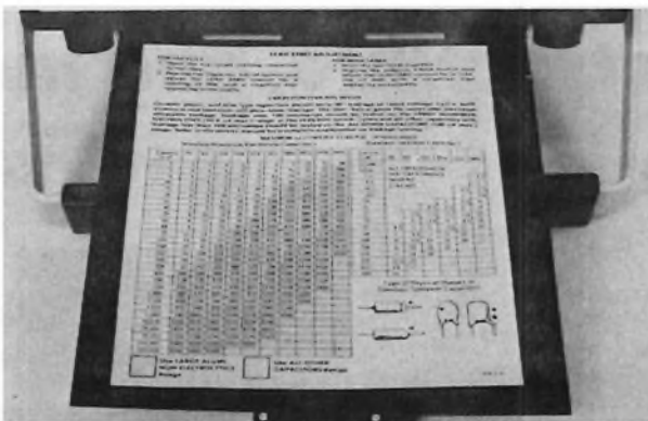
Fig. 4 — The EIA maximum allowable leakage for aluminum and tantalum capacitors are shown on the handy pull-out chart on the bottom of the unit.
