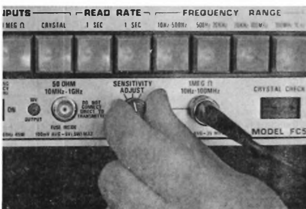
Fig. 13 — The FC51 attenuator allows noisy digital signals to be measured which will cause most other frequency counters to give an incorrect reading.
