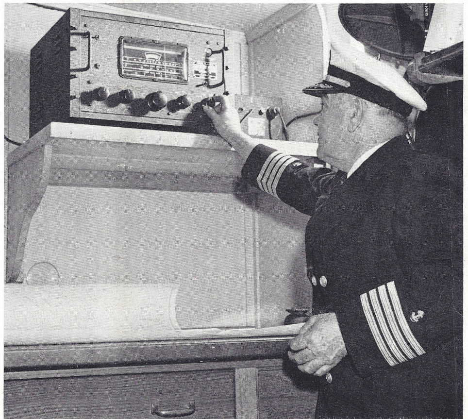
Capt. R. K. Sawyer of liberty ship Charles Carroll tunes Scott low radiation receiver installed in chart room to bring his men news and entertainment through speakers installed in mess rooms.
