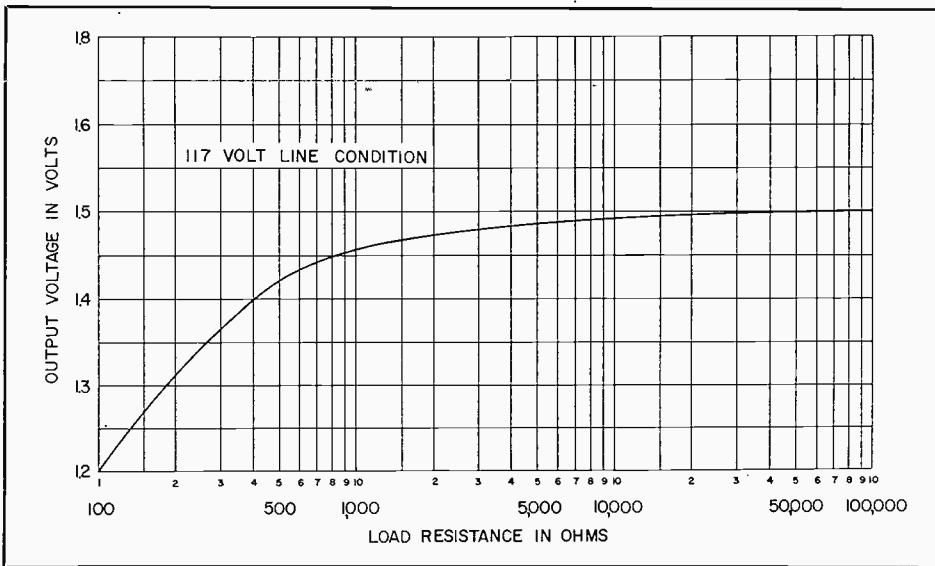
Figure 3—This curve, which was obtained under average line conditions, illustrates the minute change in output voltage over a wide range of load resistance.
