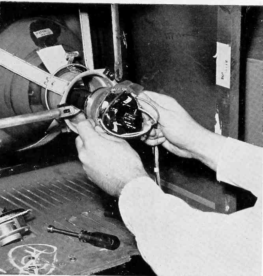
Figure 1 Removing yoke from neck of a cabinet-mounted tube.
