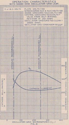
ditions specified in the figure. Oscillator-grid currents less than this minimum value will result in decreased valve life and low mixer-stage gain. The maximum oscillator-grid current recommended for this condition is 500 microamperes. Experience has shown that this current can be obtained without any of the undesirable effects mentioned previously.
