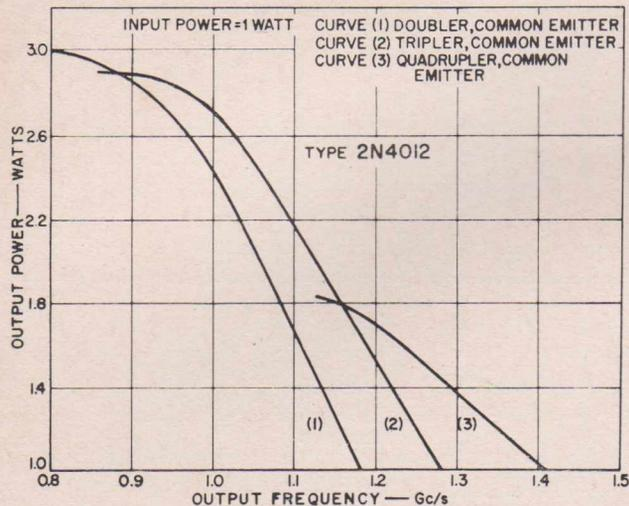
FIG. 5.—Power-output capabilities of the RCA-2N4012 overlay transistor as a function of frequency when operated in common-emitter doubler, tripler, and quadrupler circuits.
