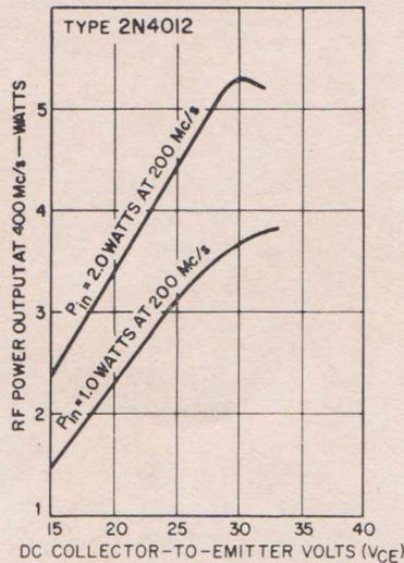
FIG. 15.—Power output as a function of collector supply voltage for the 200-to-400-Mc/s frequency doubler.
