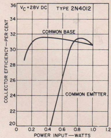
FIG. 20.—Collector efficiency as a function of input power for common-base and common-emitter circuit configurations of a 340-to-1020-Mc/s transistor frequency tripler.
