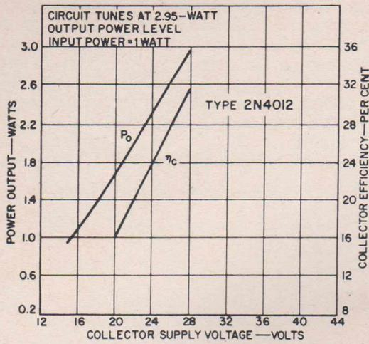
FIG. 11.—Power output as a function of the collector voltage for the 340-to-1020-Mc/s frequency tripler.
