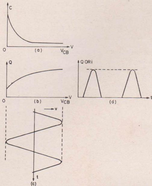
FIG. 2.—Energy transfer relationships for an overlay transistor in a frequency-multiplier circuit: (a) Capacitance-voltage curve for the collector-to-base junction; (b) Charge-voltage curve of the collector-to-base junction; (c) Sinusoidal voltage developed by the amplifier section of the transistor to drive the nonlinear collector-to-base capacitance; (d) Distorted charge, or current, waveform produced by the nonlinear collector-to-base capacitance in the generation of harmonic power.
