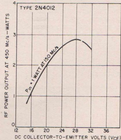
FIG. 18.—Power output as a function of the collector voltage for the 150-to-450-Mc/s frequency tripler.
