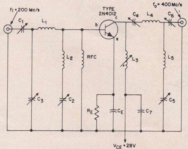
FIG. 13.—200-to-400-Mc/s, common-emitter transistor frequency doubler.
