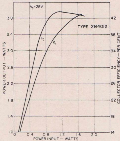
FIG. 7.—Output power and collector efficiency as a function of the input power for the 400-to-800-Mc/s frequency doubler.
