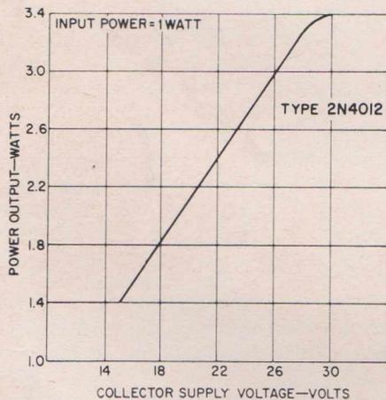
FIG. 8.—Power output as a function of the collector supply voltage for the 400-to-800-Mc/s frequency multiplier.
