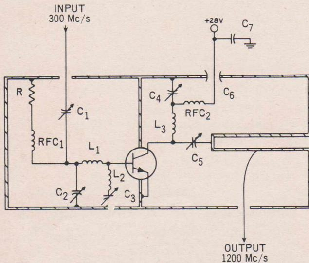
FIG. 12.—300-to-1200-Mc/s, common-emitter frequency quadrupler.
