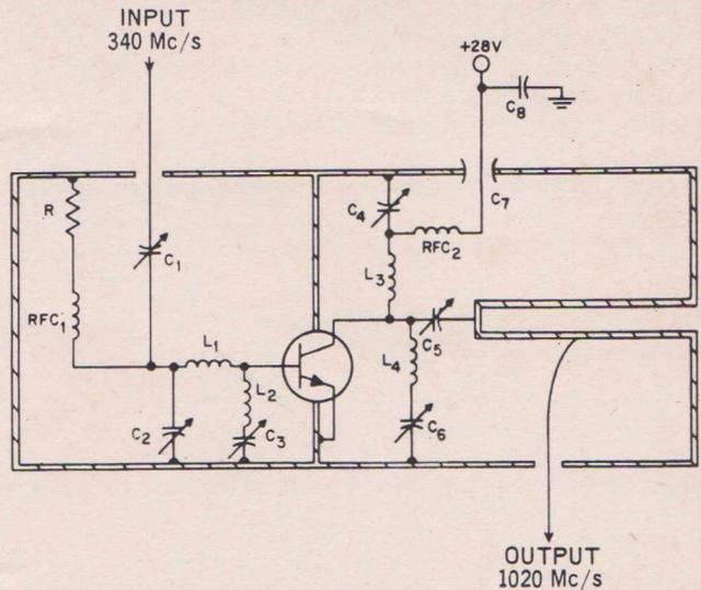
FIG. 9.—340-to-1020-Mc/s, common-emitter transistor frequency tripler.
