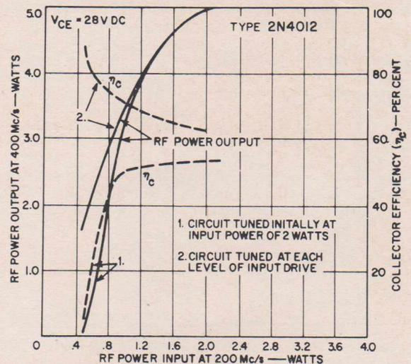
FIG. 14.—Power output and collector efficiency as a function of input power for the 200-to-400-Mc/s frequency doubler.
