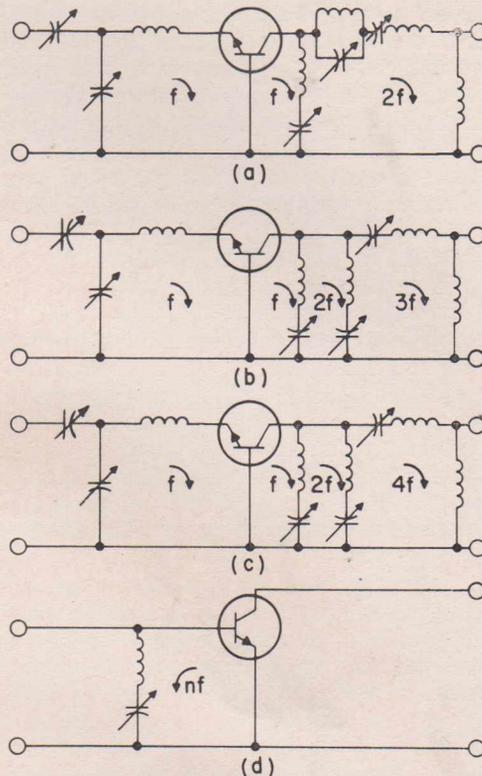
FIG. 3.—Basic circuit configurations of overlay-transistor frequency multipliers: (a) Common-base frequency doubler; (b) Common-base frequency tripler; (c) Common-base frequency quadrupler; (d) Input-circuit arrangement for a common-emitter frequency multiplier.
