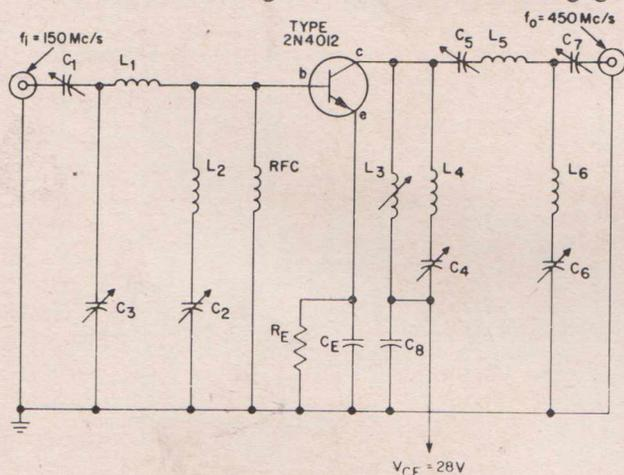
FIG. 16.—150-to-450-Mc/s, common-emitter transistor frequency tripler.
