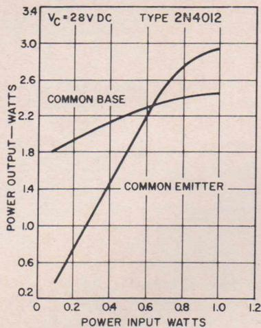
FIG. 19.—Power output as a function of power input for common-base and common-emitter circuit configurations of a 340-to-1020-Mc/s transistor frequency tripler.
