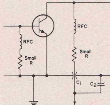
FIG. 4—Circuit showing the biasing arrangement and bypass capacitances that are used to eliminate instabilities in common-emitter frequency multipliers.
