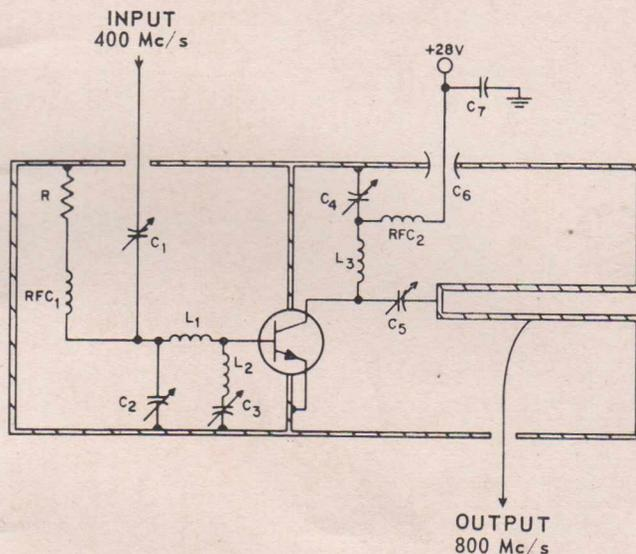
FIG. 6.—400-to-800-Mc/s, common-emitter transistor frequency doubler.
