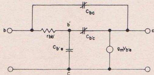
FIG. 1.—Equivalent circuit of an overlay-transistor frequency multiplier.
