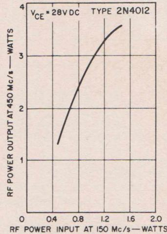
FIG. 17.—Power output as a function of power input for the 150-to-450-Mc/s frequency tripler.
