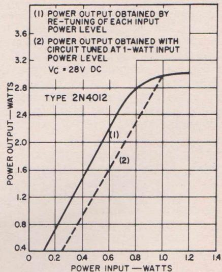
FIG. 10.—Power output as a function of power input for the 340-to-1020-Mc/s frequency tripler.
