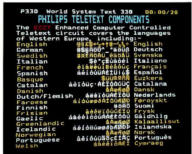
Fig.12 All the characters required for the major languages of Western Europe can be displayed using the ECCT
