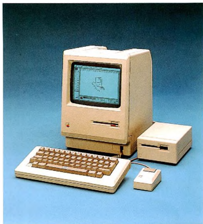
The 68000 is the foundation for one of the most sophisticated personal computers — Apple's Macintosh.
