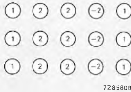
Fig.6 Stacked Bessel arrays. When the three panels are driven in parallel their radiation is omnidirectional in the horizontal plane but concentrated vertically at the level of the arrays
