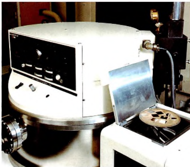
Fig.9 R.F. sputtering apparatus. The apparatus contains individual targets of gold, titanium, platinum, etc. The sputtering operation is carried out under argon at a controlled pressure of 10^{-2} to 10^{-3} torr
