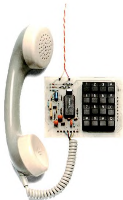
Experimental printed-circuit board with the TEA1046, its peripheral components, keyboard and handset. The basic functions of the IC are dialling tone generation, speech amplification, four to two-wire conversion, dialling/speech switching and line adaptation
