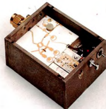
Fig.15 The ceramic disk resonator in a balanced downconverter based on alumina. The downconverter shown here operates in the 11.4 to 11.7 GHz band
