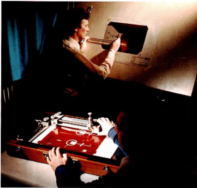
Fig.7 In the initial design phase of a system or function, the studnite pattern is produced manually to allow a fast turn-around. The apparatus in the foreground can do this job very accurately. It is, however, limited to relatively simple shapes; more complicated shapes must be cut by hand as shown in the background
