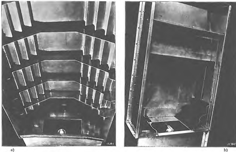
Fig. 1. Models for examining the "useful" intensity of sound in a hall. The source of sound is represented by a small lamp, shown at the bottom of the photograph. The walls of the model are made of aluminium which reflects about 50 per cent of the light-rays falling on it, so that, in accordance with the definition of the "useful" intensity, a ray after only a few reflections can just contribute to the illumination of the opal glass representing the audience. (In the pictures this glass has been removed in order to show the interior; in the upper half of fig. 1b, however, the opal glass representing the seating on the balcony is visible. Sound-absorbing surfaces in the hall are blackened in the model, e.g. the right-hand wall in fig. 1b. The brightness of the opal glass (see figs. 4, 8 and 11) represents the distribution of the useful intensity of sound.
