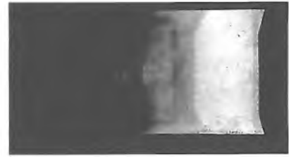
Fig. 4. Photograph of the opal glass in the model of the old hall (fig. 1a). The stage is on the right-hand side. The rapid diminution in illumination intensity towards the left may be noted; at the rear of the hall the useful sound intensity was far too small. The bright trapezoidal spot near the stage is due to reflection at the forepart of the ceiling which was not screened by the transverse roof trusses.
