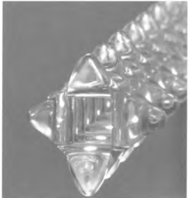
Fig. 7. Model of a stationary field distribution for a guided beam of rays inside a fibre core. The bounding surface of the field distribution is so defined that about 95% of the radiant energy is contained within it. In the direction of the optical axis it can be seen that the bounding surface has a row of maxima in both the vertical plane and the horizontal plane, and also on both sides (the maxima are the zones where the surface is furthest from the axis). Alternating with the maxima are minima — hence the guiding effect. The minima are barely visible in the photograph. The distance of the minima from the axis can however be estimated from the vertical ellipse at the front of the model. Half the minor axis of the ellipse is approximately equal to this minimum distance ( w_{min} in fig. 6). Half the major axis of the ellipse is of course equal to the maximum distance ( w_{max} in fig. 6). In this model the ratio w_{max}/w_{min} is about half the value of that used in fig. 6. Although there is this difference, the two ellipses in the group of three beam cross-sections shown in fig. 6 ( BC ) can easily be traced in this photograph.
