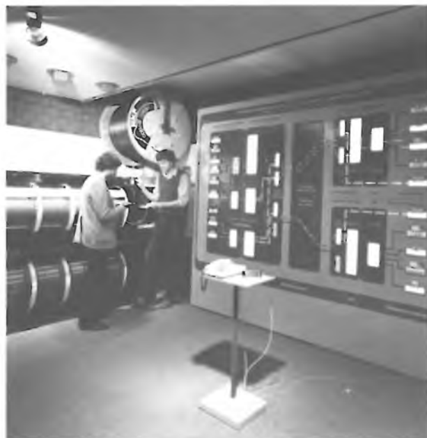
Fig. 3. Part of the experimental system in the laboratory. The reels of optical-fibre cable are on the left, and a demonstration display for the signal transfer can be seen on the right.
