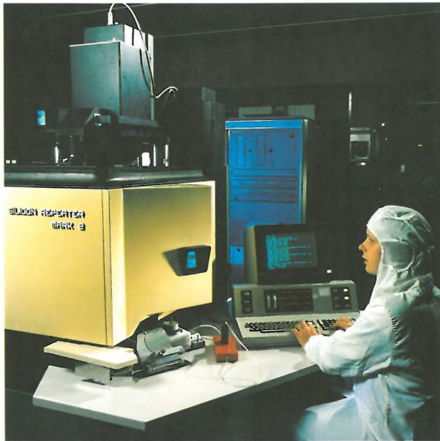
Fig. 1. The Mark 2 Silicon Repeater, an improved version of the earlier Silicon Repeater designed at Philips Research Laboratories and described in this journal [1*]. The improved Silicon Repeater can expose sixty 4-inch silicon integrated-circuit wafers per hour.
