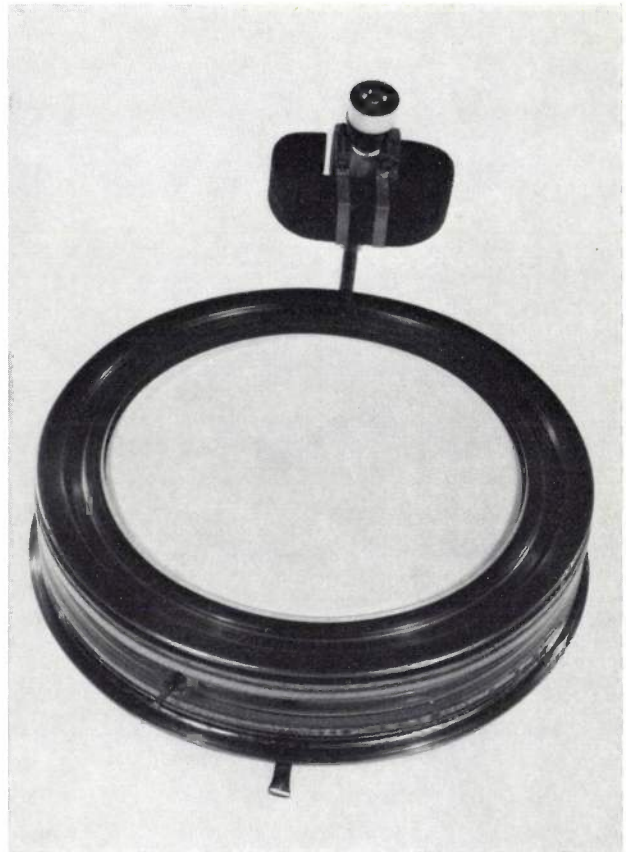
Fig. 6. An X-ray image intensifier with metal conversion foil and electron-intensity amplification by means of a channel plate. The photograph shows the glass output window with the fluorescent layer. The getter-ion pump, which remains permanently connected, removes the residual gases released from the channel plate during operation. In this construction there is no room to incorporate a conventional absorption getter of sufficiently large capacity.
