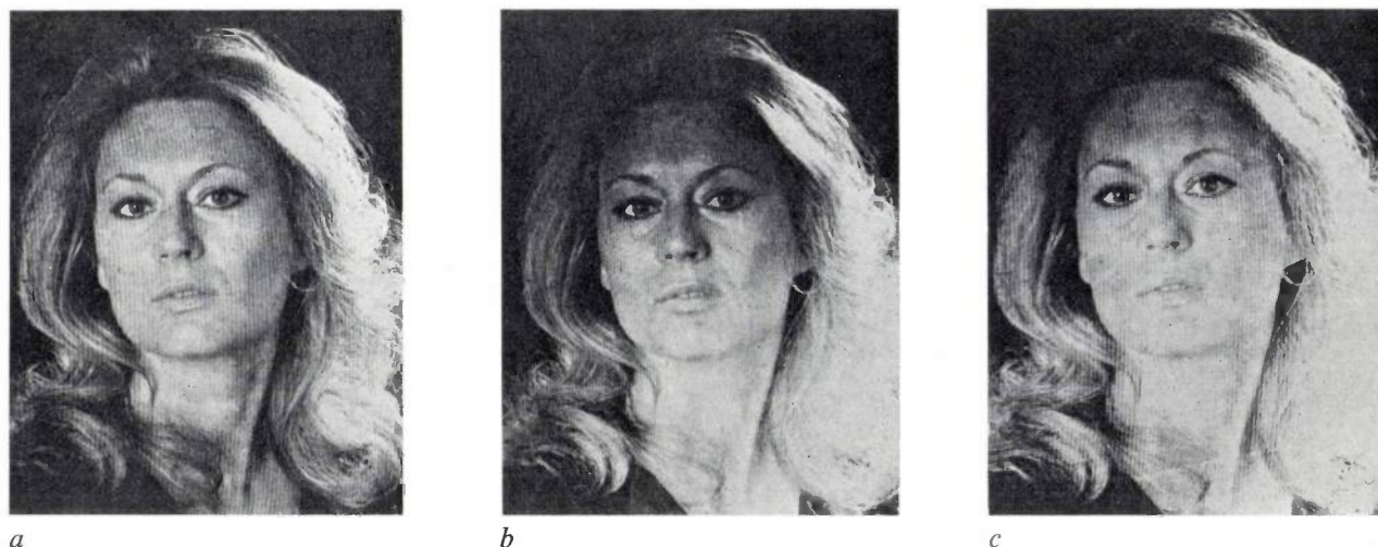
Fig. 7. Reconstruction of holograms during the various stages of thermal fixing. a ) Direct image of the object, seen through the crystal. b ) Reconstruction during recording at 150 °C. c ) Reconstruction after fixing.
