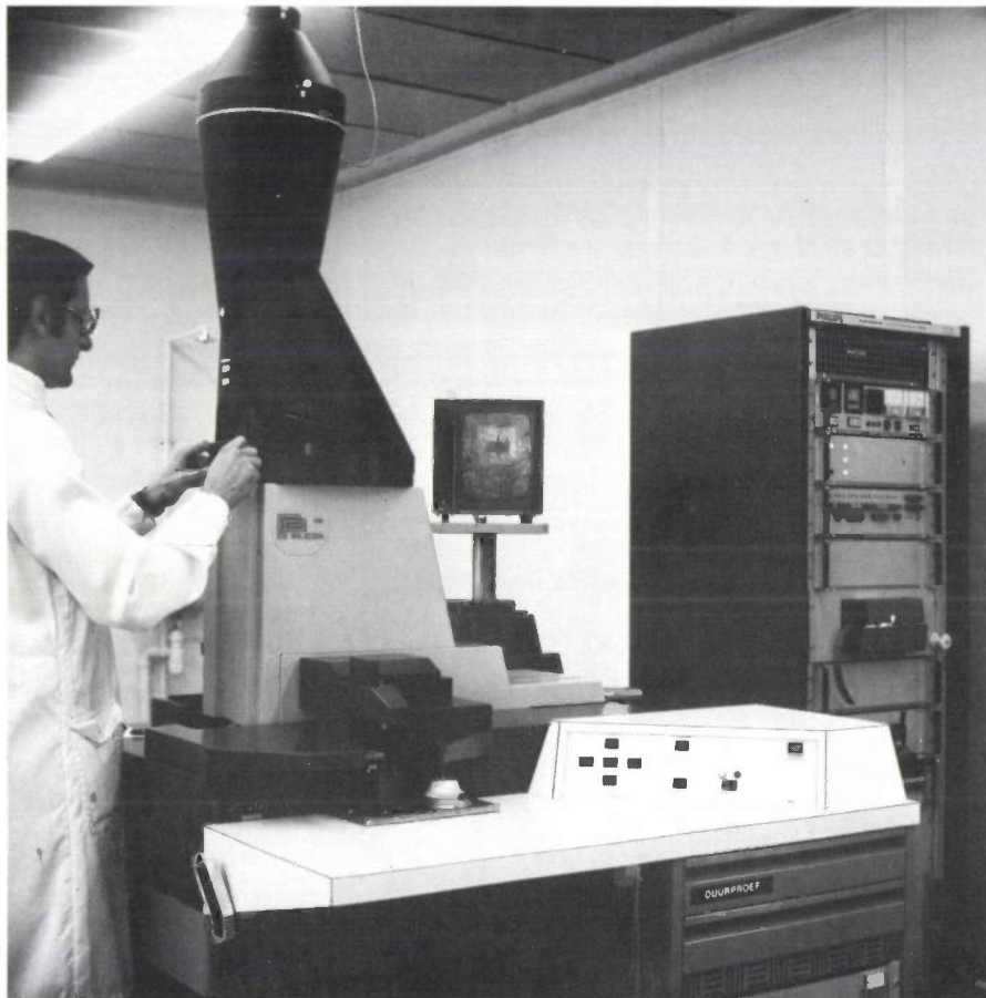
Fig. 1. The Silicon Repeater. The black column contains the illumination system. The cylindrical drum at the base of this column contains the turntable for the masks; the lighter-coloured unit underneath it accommodates the projection optics and the alignment system. All these are situated on one of the two carriages mounted on hydraulic bearings and driven by hydraulic motors. The other carriage, not shown in the photograph, carries the wafer table with the silicon wafer to be exposed. To change the wafers the table can be slid out of the equipment at the front. The monitor in the background shows the alignment marks on wafer and mask, which are used for the coarse alignment, set manually by the knobs on the control panel in the foreground. After this initial coarse alignment, the accurate alignment is carried out automatically by the computer in the background.
