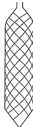
Fig. 9. Diagram of a cracked crystal. Cracks are usually formed at 45° to the axis.
