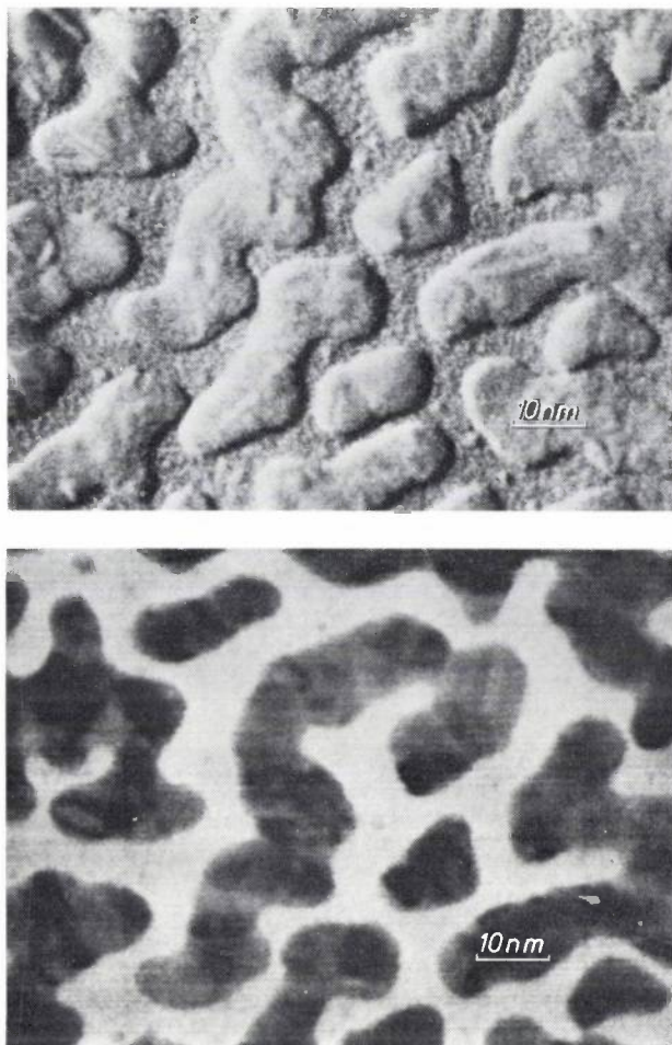
Fig. 6. Photographs of gold islands on a collodion film. The lower photograph was taken with the sum signal and the upper one with the difference signal, which means that they show an amplitude image and a differentiated phase image respectively. The direction of differentiation is from left to right. Since the collodion film behaves as a weak phase object, it remains practically invisible in the amplitude image, thus greatly enhancing the observability of the islands.
