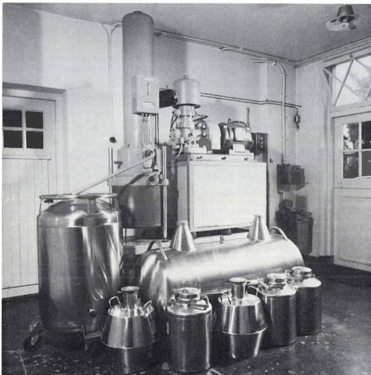
Fig. 12. Equipment for the production and storage of liquid nitrogen. The Philips PLN 106 liquid-nitrogen unit can be seen in the background; it consists of the PW 7160 refrigerating machine (right) and the PW 7170 air fractionating column (left). In the foreground are two large containers for liquid nitrogen alongside containers for the storage of bovine semen.
