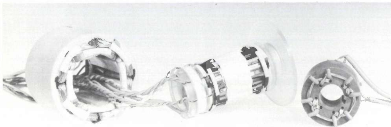
Fig. 6. The focus coil ( centre ), the coils for correcting astigmatism (the stigmators, left ) and a coil for scanning the substrate (when the column is used as an SEM). Each stigmator consists of four vertically wound coils forming a magnetic quadrupole. One unit is aligned with the x - and y -axes, the other is at 45^\circ to them. The focus coil is a simple solenoid, with compensating coils placed around it to improve the symmetry of the field. In reality it is mounted inside the stigmators.
