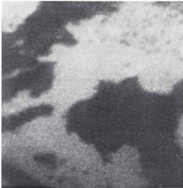
Fig. 11. An example of a magnetic-contrast image made with an SEM. The darker and lighter regions represent ferromagnetic domain structure on the basal surface of a single crystal of magnetoplumbite. Because of Lorentz forces, the fringing fields deflect the secondary electrons emitted from the sample. These deflections produce the contrast in the image.
