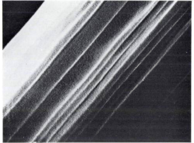
Fig. 2. Domain structure of an uncoated cleavage surface of a single crystal of \text{BaTiO}_3 . The polarization vectors in adjacent domains are perpendicular to each other. The image was made with a scanning electron microscope (SEM), using voltage contrast.
