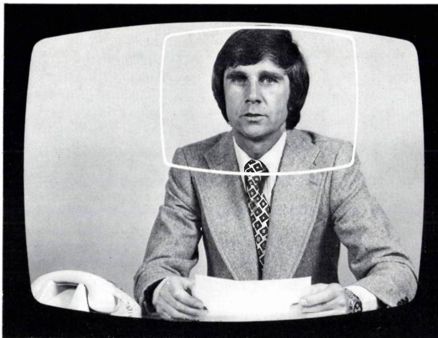
Fig. 3. A picture of about 300 lines, as used for the video telephone, is equivalent to one-quarter of the picture used for broadcast television.
