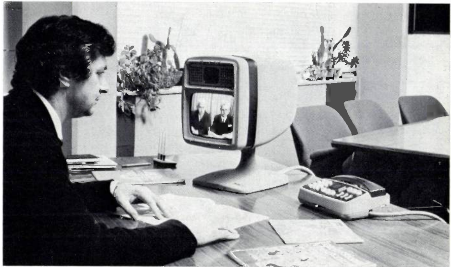
Fig. 5. Video-telephone station set designed by Philips Telecommunication Industries (PTI) for use in the national experimental network. Like the set developed at Philips Research Laboratories (fig. 4) it consists of three units. The technical differences are only minor.
