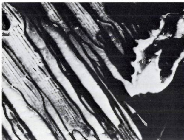
Fig. 6. Photomicrograph of a single crystal of TGS, showing 'beam writing' produced by an SEM. The 'writing' consists of a row of dashes formed in non-adjacent domains of the same polarization. The dashes represent local reversals brought about by individual scans. The beam current was 10^{-9} A.
