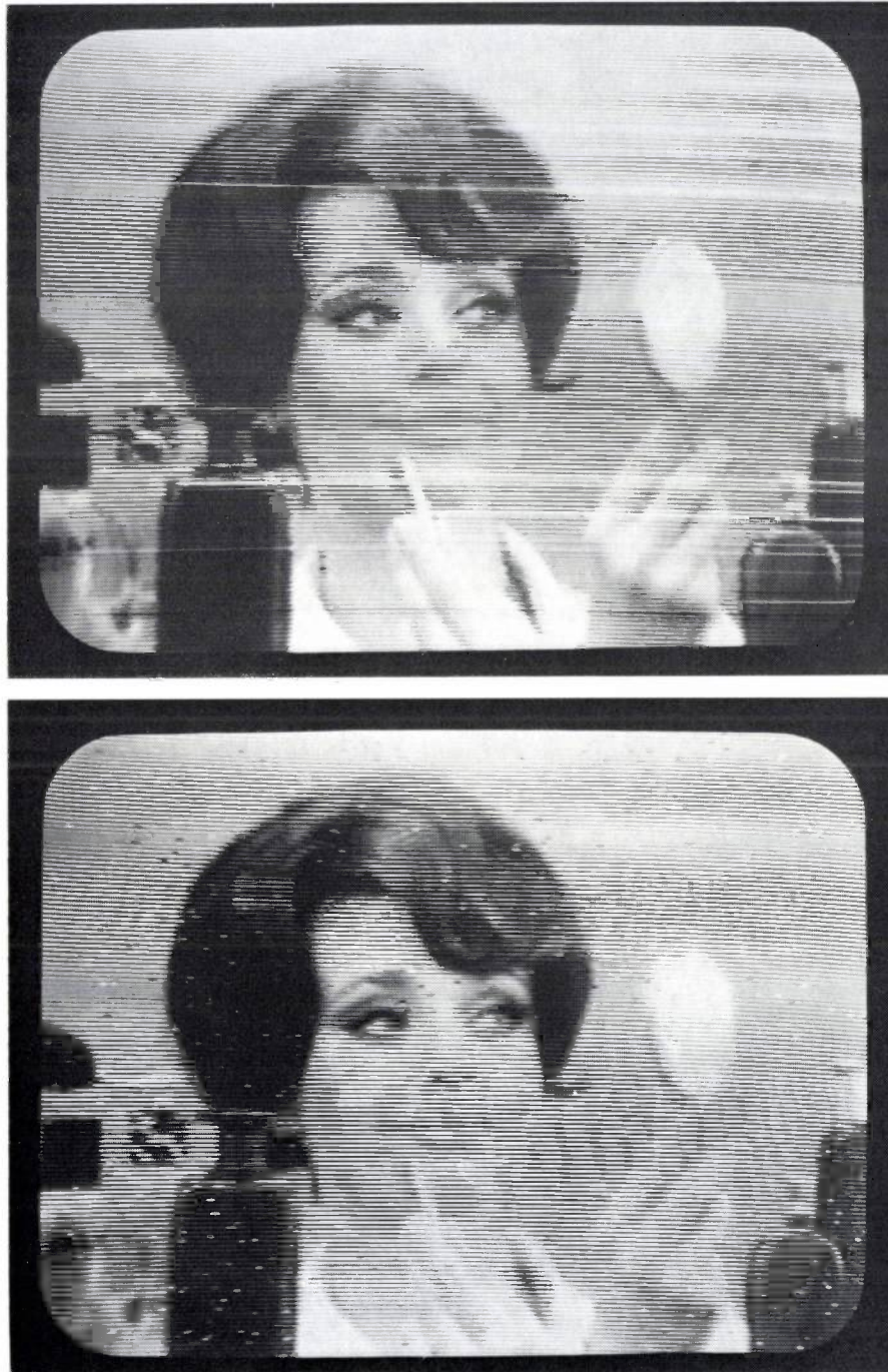
Fig. 64. Television-picture degradation due to bit errors in transmission, above : with DPCM ( P_e = 3.3 \times 10^{-4} ), below : with PCM ( P_e = 10^{-2} ). The probabilities P_e of a bit error for the two cases have been chosen so as to give about the same degradation. DPCM is thus about 30 times more sensitive to bit errors than PCM.
