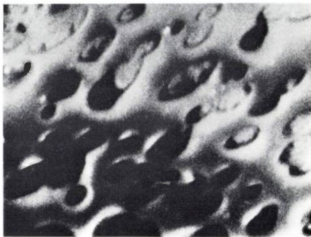
Fig. 5. An intermediate stage in the charge-compensation process (see fig. 4 c ). The areas inside the domain walls are still partly black, indicating that charge compensation is not yet complete.
