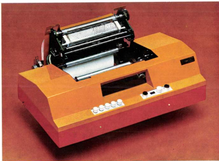
Fig. 1. An electrostatic printer used for the real-time presentation of acoustic spectra. The printer has been opened for loading with paper.
