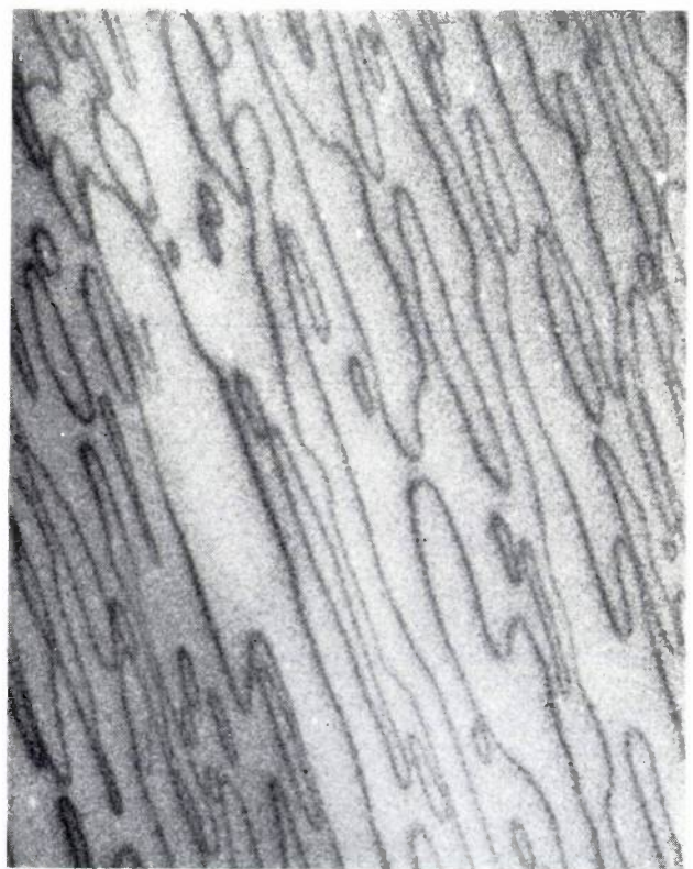
Fig. 1. The surface of a single crystal of the ferroelectric TGS (triglycine sulfate). Adjacent domains have opposite polarizations. The image, obtained with a scanning electron microscope, is produced by the effect of the electric field from the various domains on the secondary electrons emitted by the surface ('voltage contrast'). The surface of the sample was optically flat and uncoated. The small whitespots denote the build-up of surface charge.
