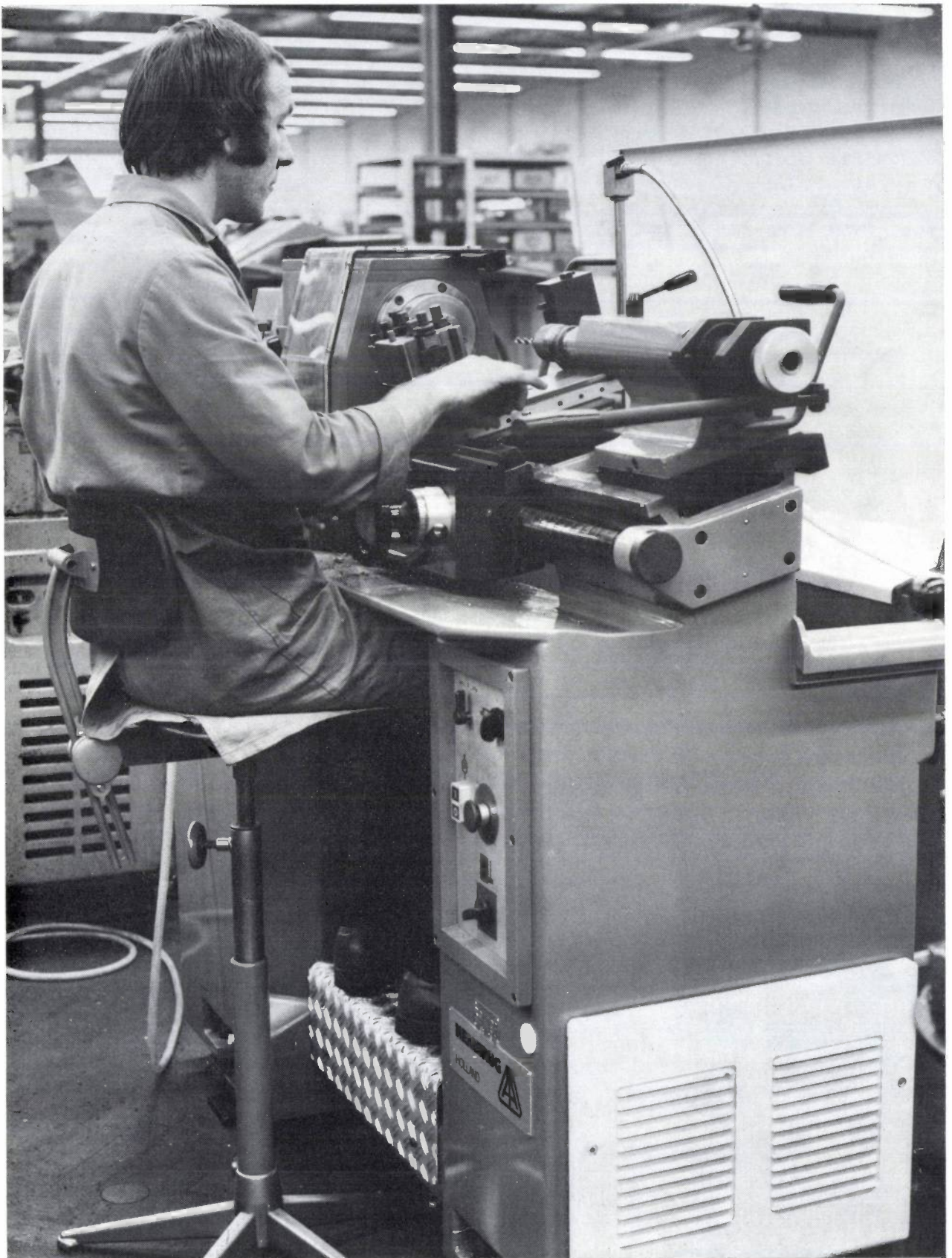
The 'Ergonomic', an ergonomically designed lathe, the result of cooperation with N.V. Hembrug. The operator can work comfortably at this lathe either seated or standing.
