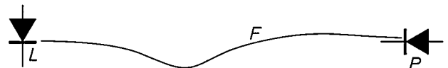
Fig. 1. Schematic representation of an optical telecommunication channel with a glass fibre F , a GaAs laser diode L and an avalanche photodiode P . The laser emits a beam of infrared radiation whose axis is in line with the junction of the laser diode. The avalanche photodiode detects radiation incident at right angles to the P-N junction.
