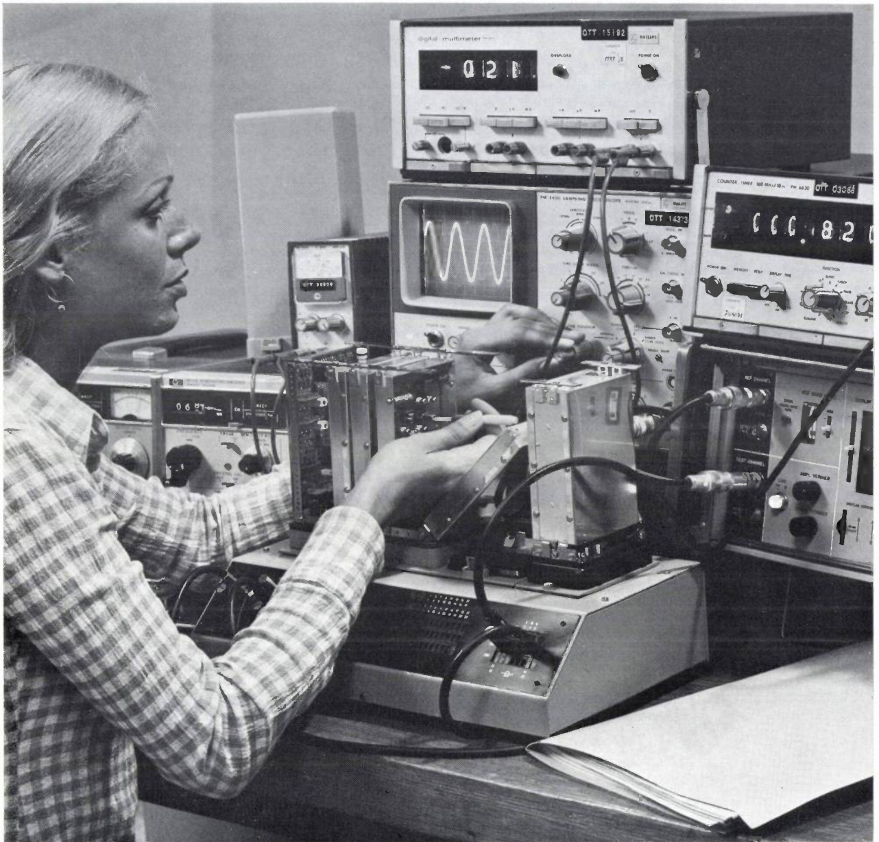
Adjustment of a 60-MHz modulator for carrier telephony. The 60-MHz carrier can be modulated by 10 800 speech channels in frequency-division multiplex (FDM); single-sideband modulation is used.
