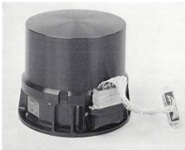
Fig. 4. The reaction wheel. The whole structure is 150 mm in height and in diameter, and weighs 2795 g. The connector block has an extension cord (the 'pin-saver'), which is used during pre-flight testing to protect the connector pins in the wheel from being damaged by repeated plugging and unplugging.
