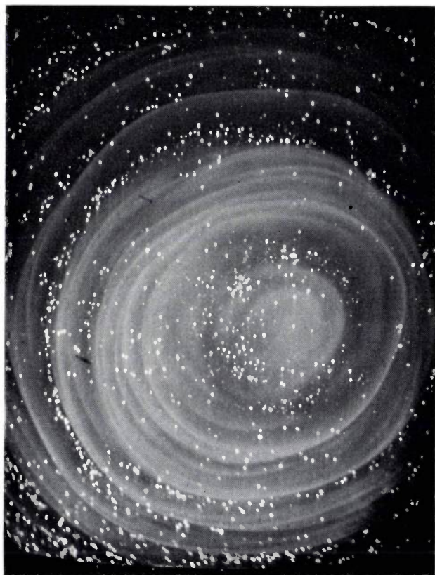
Fig. 1. Monitor picture from a silicon vidicon [31] with a target of dislocation-free silicon (cross-section 25 mm) operating in darkness. The bright spots are leaky diodes; they are distributed in a spiral pattern. The continuous spiral pattern is background leakage, probably due to impurities. Magnification 9\times .
