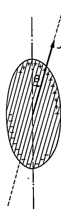
Fig. 5. A magnetized ellipsoid of revolution of a ferromagnetic material, where the polarization vector J makes a small angle \theta with the major axis. The demagnetizing field inside the ellipsoid is homogeneous.
