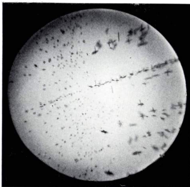
Fig. 3. Infrared micrograph of a region at the edge of a silicon crystal grown in the \langle 111 \rangle direction. The microdefects have been made visible by 'decorating' with copper. Magnification 170 \times .
