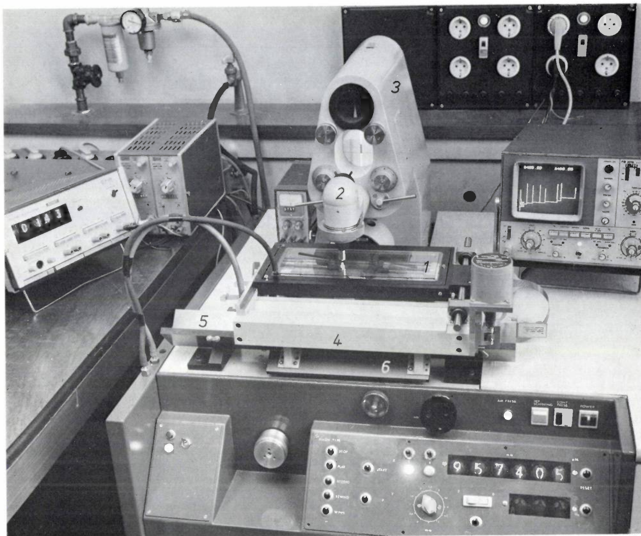
Fig. 1. Automatic microphotometer. A stationary beam of light passes upward through the photographic plate 1 (glass, 10 \times 25 cm) and via the reading head 2 to a photosensitive cell in the housing 3. A spectrum is scanned by moving the plate in the x -direction along the reading head by means of an electric motor. The slide 4, on which the photographic plate is held by suction to a glass plate, travels on a cushion of air in a V-shaped guideway 5 (see fig. 2). The position is measured with an optical system, using a reflection phase grating mounted under the slide (6). To change from one spectrum to another the plate is moved in the y -direction. Both movements can be controlled by a computer as well as by hand. A digital reading of the position in the x -direction is given to an accuracy of 1.25 \mu\text{m} . Any part of the spectrum can be displayed on an oscilloscope screen. The measured blackening can be read at all times on the digital meter on the left. Parts of the 'Schnellphotometer' made by the Jenoptik company of Jena were used in the construction of this equipment.
