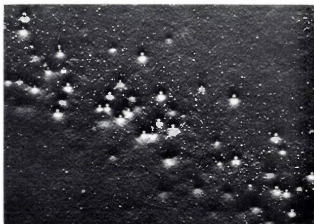
Fig. 8. Preferentially etched silicon with etch pits of various sizes. The etch pits have been made more clearly visible by using interference contrast (Nomarski's method, magnification 150\times ).
