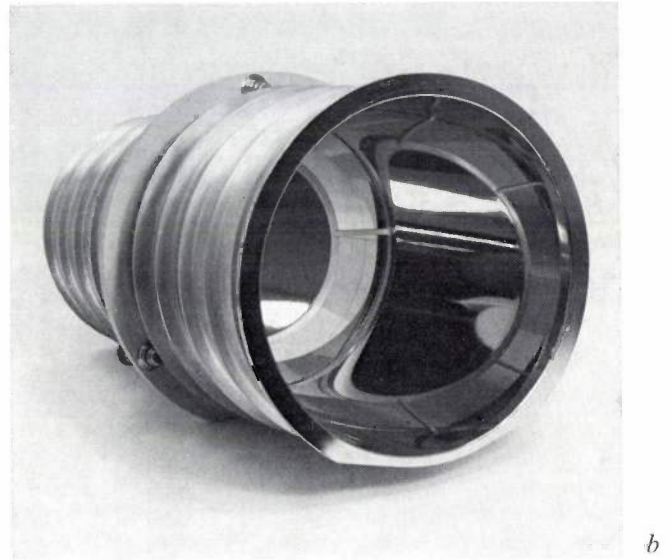
Fig. 17. a) The parabolic reflector for radiation with a wavelength greater than 45 Å. S screen. T vignetting tube. The paths of three rays are shown. If the tube T were not there, ray 1 originating from the cosmic background, or from some source or other, would reach the detector without being reflected from the mirror. Ray 2, which would reach the mirror without being reflected, is blocked by the screen. Ray 3 belongs to a beam originating from the region of the sky within the desired field of view. The parabolic reflector directs this beam on to the detector. The left-hand part of the paraboloid does not contribute to the reflection. The angle of incidence here is greater than the critical angle. b) Photograph of the paraboloid. The reflector was designed by the Space Research Laboratory at Utrecht and made by Philips Research Laboratories in Eindhoven. Typical of the dimensional accuracy is the size of the focus for paraxial radiation. The overall half-width of this focus is 0.18 mm. The focal length is 80 cm. The geometric surface is 140 cm 2 . The weight is 3.3 kg.
