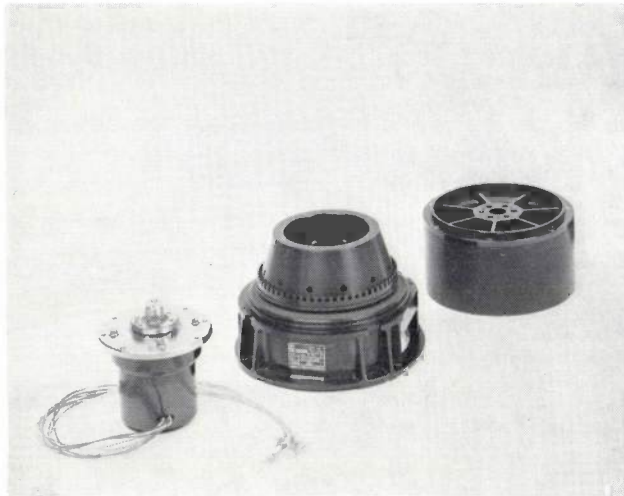
Fig. 3. Components of the reaction wheel; from left to right: the motor with bearing, the housing and the inertia wheel.
