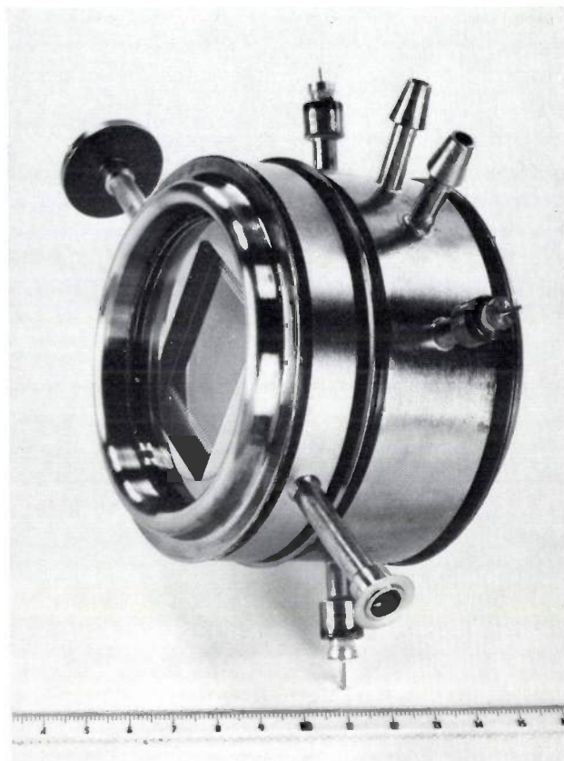
Fig. 3. Experimental model of Phototitus. The multilayer structure is mounted in an evacuated container; the selenium layer can be seen through the window. Two Peltier elements are also mounted in the container; these cool the system to -50^\circ\text{C} .
