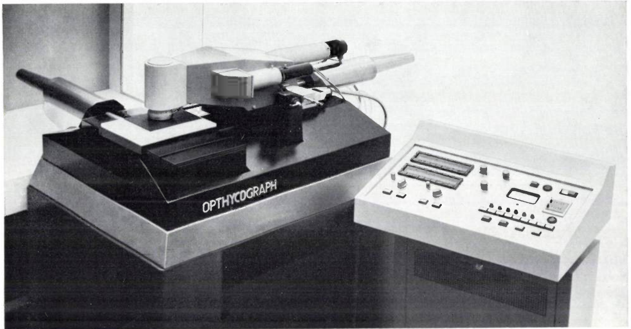
Fig. 1. The Opthycograph, with the control desk on the right and the actual pattern-drawing part on the left. The slide with the photographic plate can be seen on the left-hand side of the drawing machine and behind it the linear hydraulic motor that drives the slide. Situated on the right of this slide is the slide with the optical column, containing separate projection systems for line drawing and for the flashing-in of frequently recurring details. The drive for this slide is on the far right. The carriage slideways are located under the dark cover bearing the name of the machine. Telescopically sliding parts in this cover ensure that the slideways, which are entirely covered with oil from the slide bearings, always remain completely enclosed. During the drawing operations the photographic plate lies on its carriage unshielded, and the machine is therefore operated in a completely dark and dust-free room.
