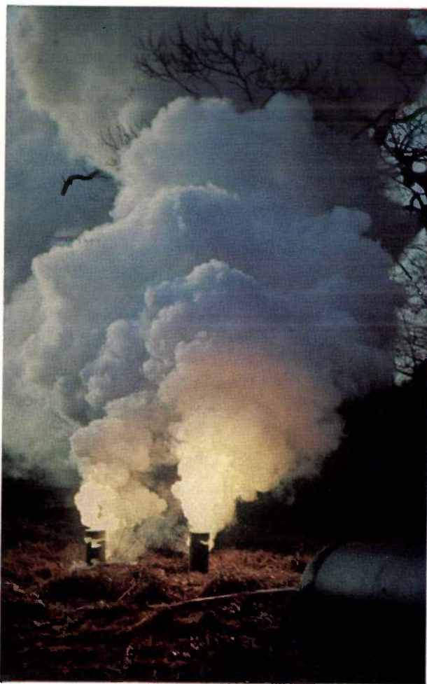
Fig. 1. Reaction between powdered aluminium and red phosphorus, resulting in the formation of aluminium phosphide.
