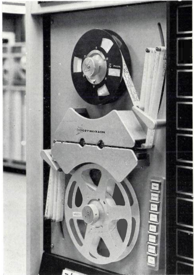
Fig. 12. Commercially available punched tape reader with a reading speed of about 1,000 characters per second, in use in Philips' Computer Centre, Eindhoven.
