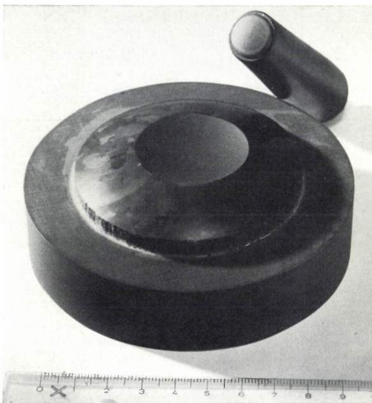
Fig. 2. A mortar of silicon carbide in a plastic base. The relatively large single crystals of which the mortar is built up can be seen at the left-hand edge. The pestle is also of silicon carbide (with a plastic handle).
