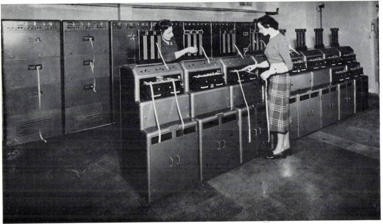
Fig. 2. Photograph of a torn-tape exchange based on the principle of fig. 1. The reperforators are in the background, with the transmitters and waiting bays in front.
