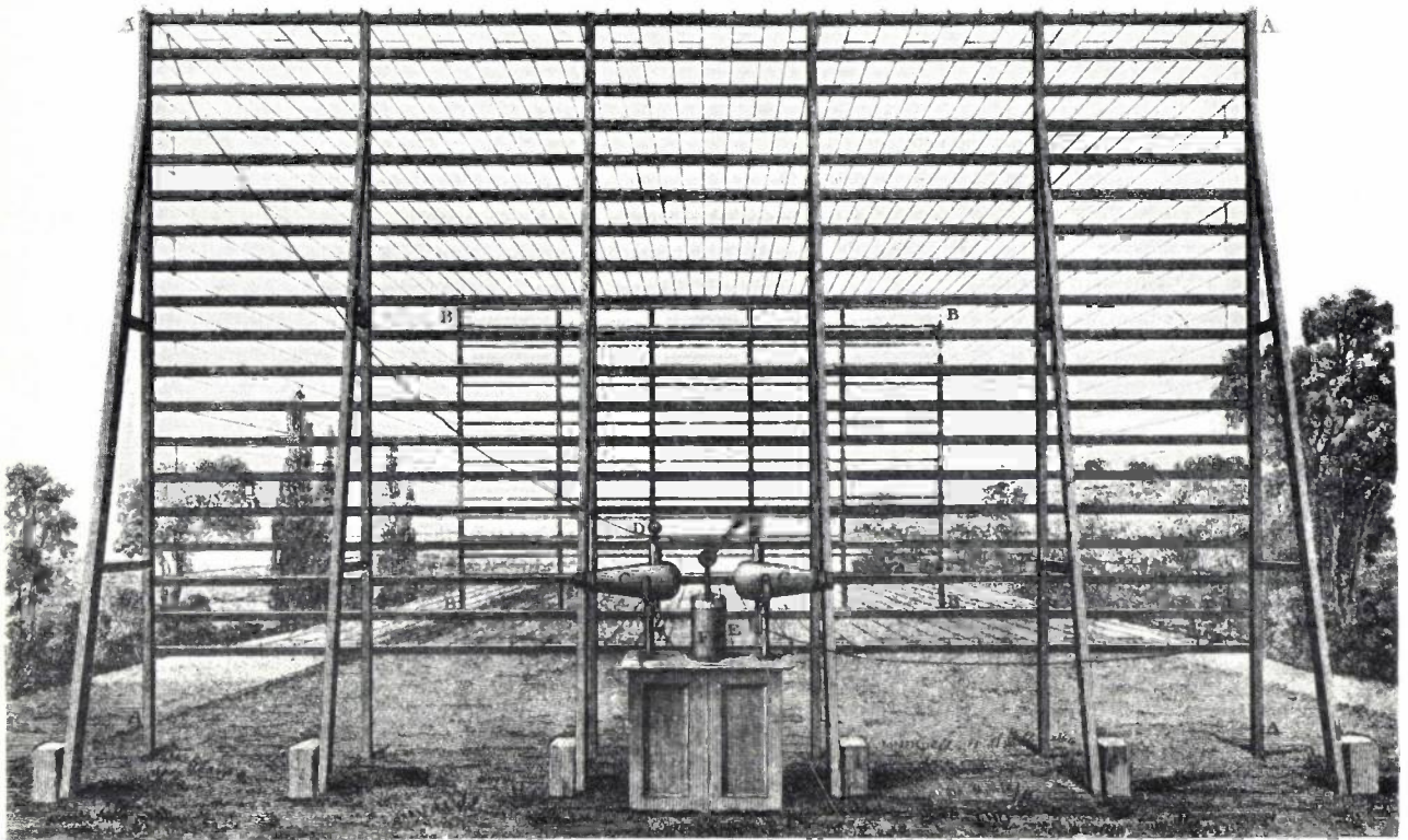
Fig. 6. Experimental arrangement of Ronalds' electrostatic telegraph in the garden of his house at Hammersmith, London. Between the large frames, Ronalds had suspended 8 miles of wire.
