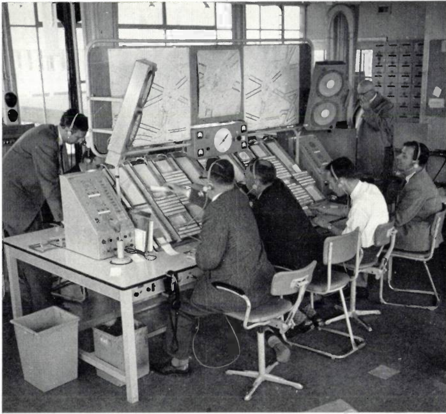
Fig. 1. The air traffic control room before the introduction of the new equipment. The stand on the table is divided into a number of sections, each of which corresponds with one of the reporting positions in the Flight Information Region. Each section contains a flight progress strip for every aircraft that is shortly to pass over the reporting position. By comparing the progress strips for each reporting position the control officer can evaluate the risk of possible conflict situations.
