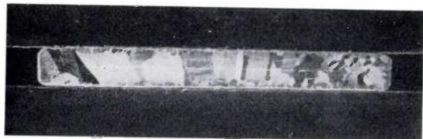
Fig. 16. Ag with 1.5 weight % Mn, 48 h on 800 °C in air; etched \text{NH}_4\text{OH} + \text{H}_2\text{O} . Magnification 10 \times . Although oxidation is completed, a "middle-line", poor in oxide, persists.
