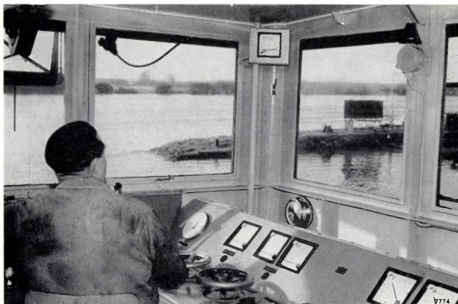
Fig. 10. Control cabin of the sand dredger. The meter near the ceiling gives a continuous indication of the sand concentration in the pumped mixture of sand and water.
