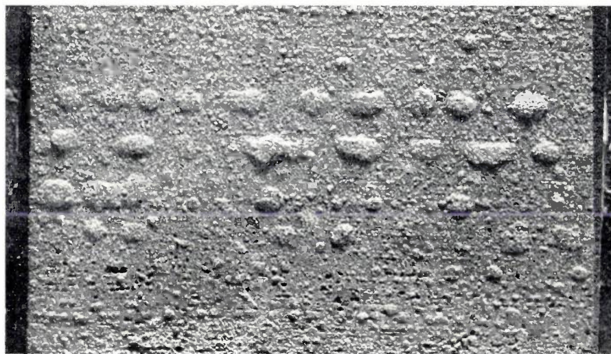
Fig. 10. Blisters formed during pickling of steel. In the pickling process atomic hydrogen is produced which diffuses inwards and forms molecular hydrogen at inclusions in the steel. The blisters appear where these inclusions are immediately below the surface. Magnification 10×. The regular pattern of the blisters indicates a regularity of the inclusions, brought about during the rolling of the steel.
