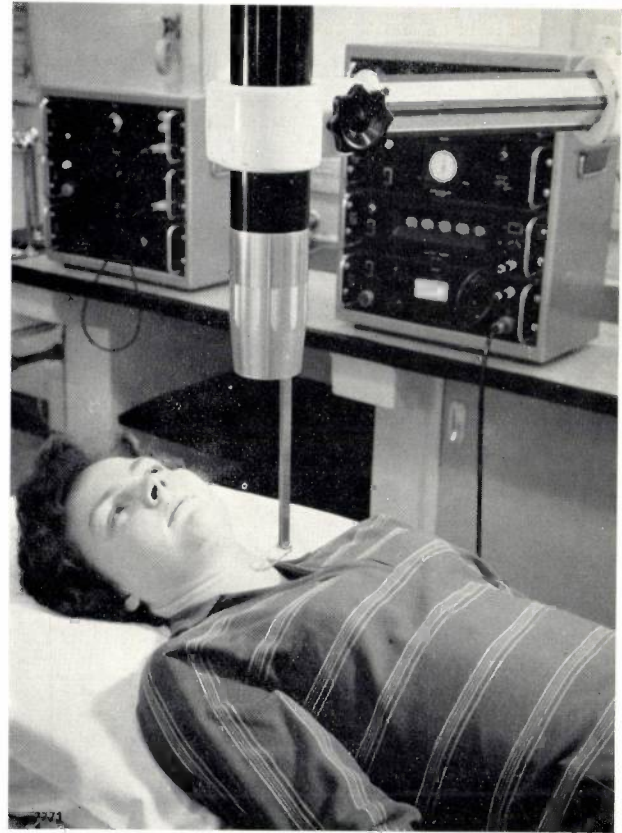
Fig. 6. Investigating the activity of the thyroid gland by means of a radioactive tracer, iodine-131, orally administered to the patient some time beforehand. The radiation pick-up (a scintillation detector) above the patient is shielded in such a way that only the gamma rays from the thyroid are measured. (Photograph by courtesy of St. Annadal Hospital, Maastricht.)
