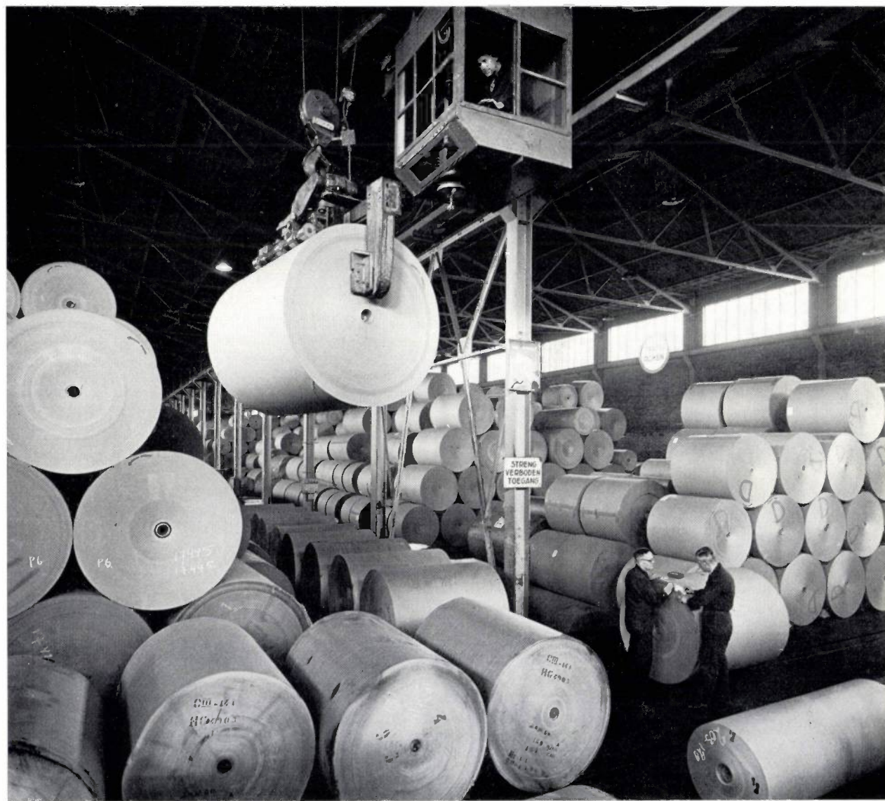
Fig. 1. The roll stores of Philips' corrugated-cardboard factory at Eindhoven. Every year these stores handle 36 000 metric tons of paper, which are processed into corrugated cardboard.
