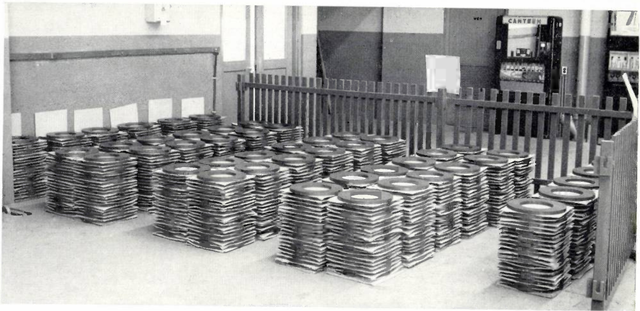
Fig. 9. Ferrite rings for the 12 accelerator stations of the 33-BeV proton synchrotron at Brookhaven. (Photograph by courtesy of Brookhaven National Laboratory.)
