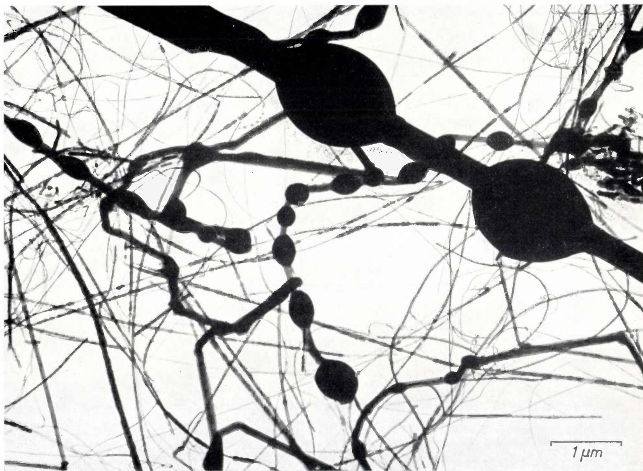
Fig. 1. Electron-photomicrograph of whiskers of various types produced in the reaction between carbon and quartz sand when heated for several hours at 1500 °C in an argon atmosphere. The whiskers are formed principally on the carbon particles. They were removed by placing against the particles a piece of copper-wire gauze, made sticky by immersion in a very dilute solution of polyester resin in amyl acetate. If the heating takes place at higher temperatures the crystals quickly grow long and thick enough to be seen with the naked eye.
