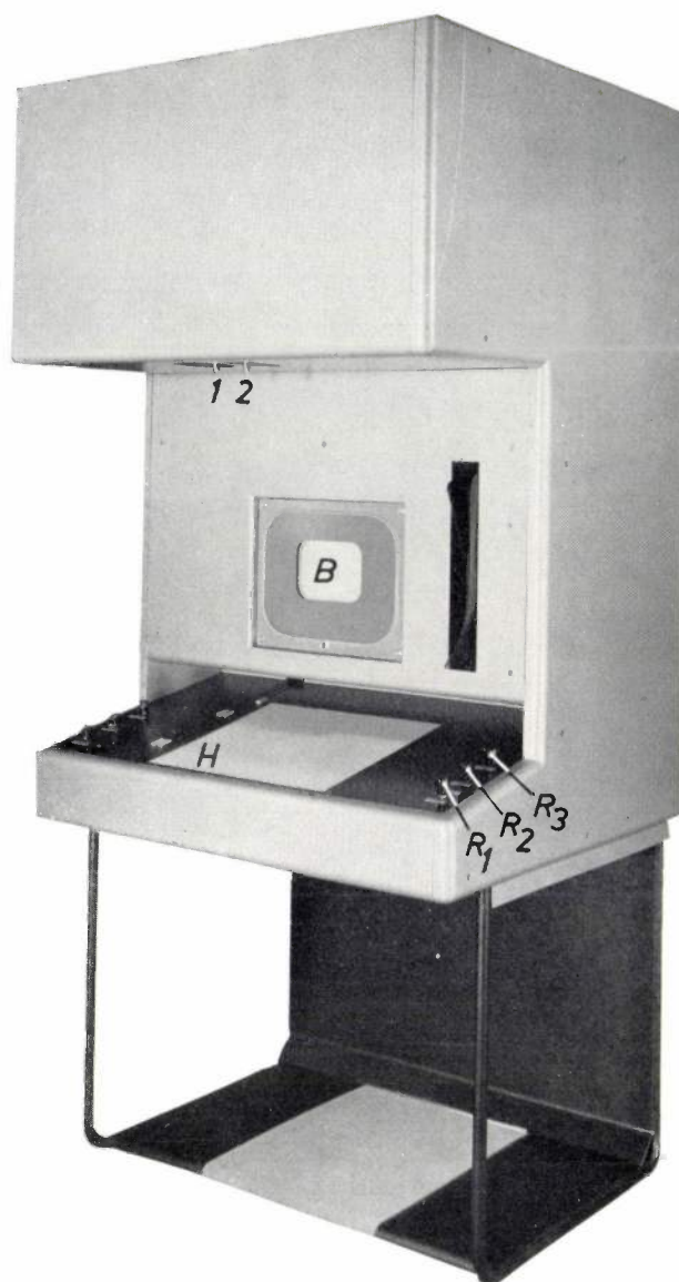
Fig. 6. Experimental model of the Ampliscope. H glass plate on which is placed the X-ray negative to be examined. B screen of the television tube on which the harmonized picture appears. 1 and 2 controls of the optics of the two television cameras. The degree of harmonization can be varied by means of the knob R_1 . (The picture shown on the screen can be changed from a negative to a positive by simply reversing the signals; see e.g. the article cited in ref. 4.) The knob R_2 controls the contrast amplification, and R_3 the mean brightness of the picture. To the left of H , the main switch, a switch for the light source which illuminates the photo to be inspected, and a switch for the lighting of the room are to be seen.
