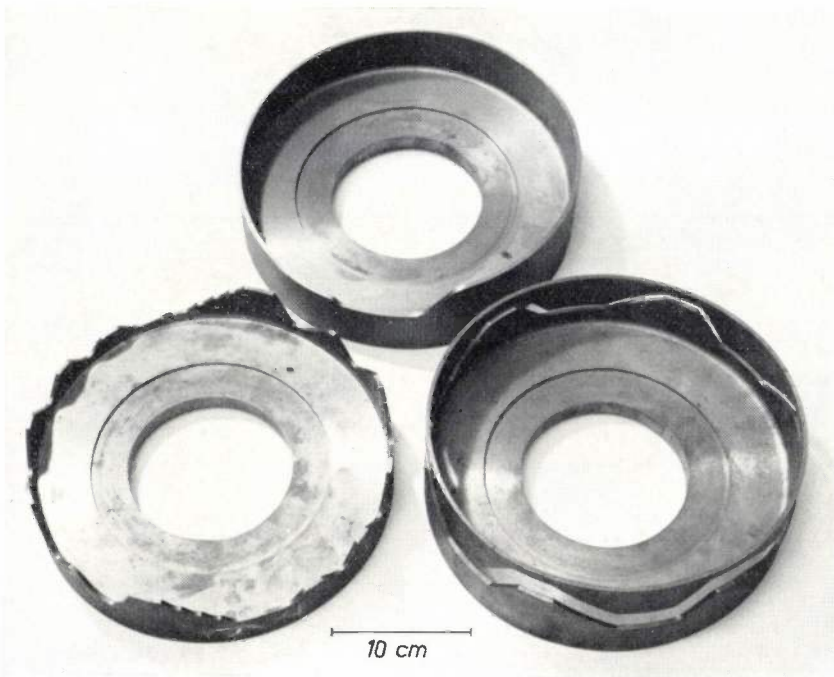
Fig. 3. Some surface cams made with the numerically controlled milling machine. The upper one is similar in shape to those used for grid-winding machines, while the two others were made to test the accuracy of the numerical controlled milling machine. The edge which was cut away during milling has been placed above the right-hand one.
