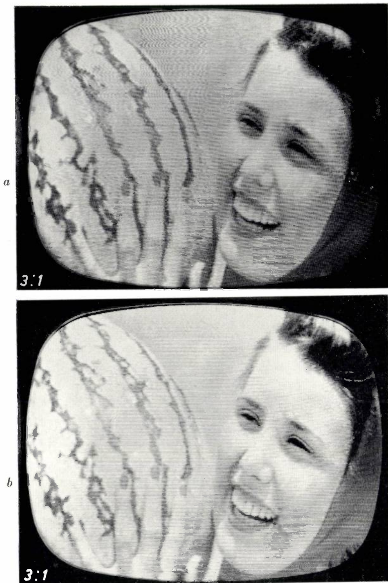
Fig. 5. Television picture recorded and played back with the apparatus described. In a ) the line-synchronizing pulses were out of alignment (fig. 4 a ); in b ) the situation was as in fig. 4 b . In both cases deliberate steps were taken to produce strong crosstalk, i.e. a ratio of 3 : 1 between the desired and the interference signal in the playback head.
