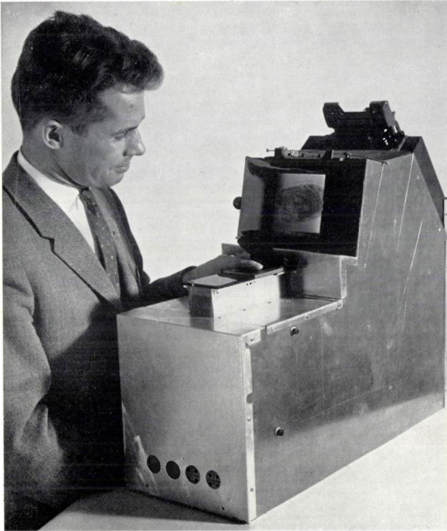
Fig. 1. Fingerprint recording apparatus. The finger is pressed on a face of a glass prism. On the ground-glass viewing screen an image of the surface relief of the finger at magnification 4\times is produced. No ink is used. At the back of the apparatus a plate camera is mounted by which either negatives or instant prints using Polaroid film can be made. (Another apparatus has been built using a 35 mm camera.)
