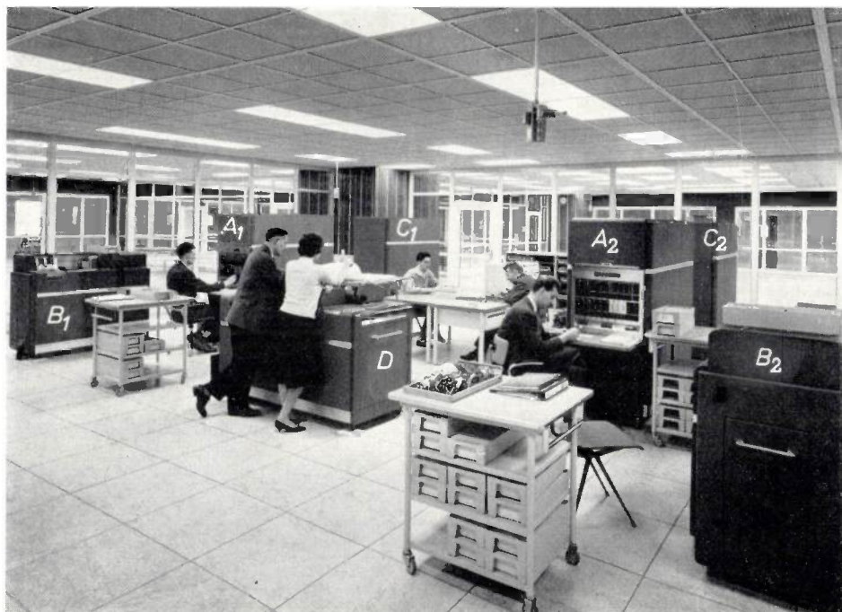
Fig. 1. Two IBM 650 electronic computers in Philips Computing Centre at Eindhoven. A_1 and A_2 are the actual computers, B_1 and B_2 the punched-card machines, and C_1 and C_2 the power units. The line printer D serves for both installations.
