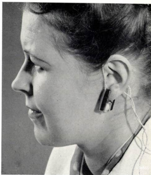
Fig. 3. Showing how the clip is attached to the ear and how the wires are arranged so that they will not cause undue interference by communicating their movements to the clip. The clip itself weighs about 2\frac{1}{2} grams; the spring tension should not exceed 20 to 30 grams.
