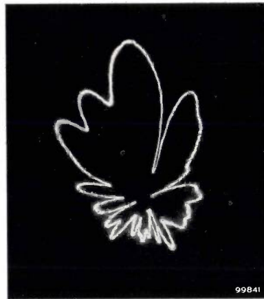
Fig. 11. Directivity patterns recorded at different frequencies on a double-cone loudspeaker, type 9710 M (outer diameter 216 mm), without cabinet or baffle.
