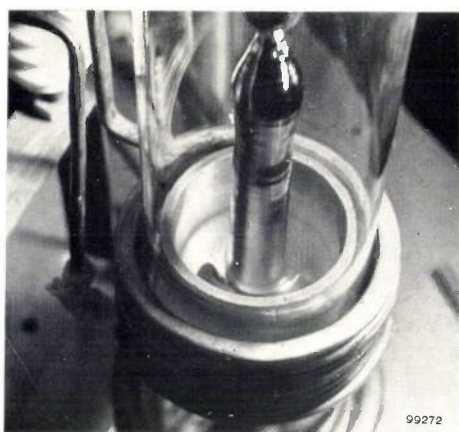
Fig. 6. Pulling a single crystal from the melt. The operation is almost complete. The photograph shows clearly the shape of the crystal obtained.
