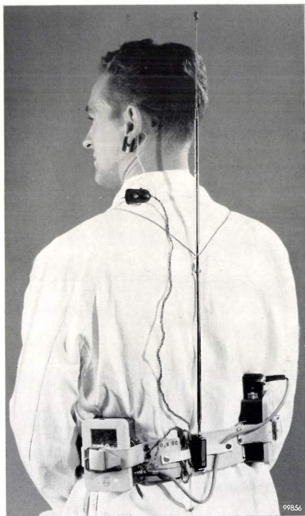
Fig. 1. The part of the apparatus worn by the subject. The subject is not obstructed in his movements.
