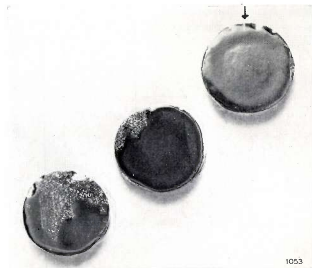
Fig. 4. Etched surface of three discs cut from an originally dislocation-free germanium crystal which, during the pulling process, came into contact with a piece of graphite on the melt. The disc on the right was cut at the point of collision; the two others were cut successively 5 mm further in the subsequently solidified part of the crystal. At the point of collision (see arrow) dislocation sources were evidently produced, from which stems a growing network of dislocations.
