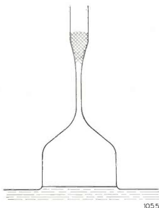
Fig. 2. In the necked portion of the crystal the dislocations as they grow with the crystal are bound to intersect the surface, where they must necessarily end; new dislocations cannot form because the thermal stresses are too small. In the lower portion, of large diameter, the thermal stresses are considerable, but now they create no dislocations because there are no longer any dislocation sources present.
