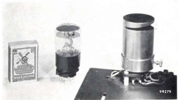
Fig. 4. Photoresistor, type ORP 30, mounted in a can with wedge-shaped aperture (diaphragm), seen from the light source. The light enters the aperture, where it is diffusely reflected so that every part of the horizontal photosensitive surface inside is equally illuminated. The illumination of the photoresistor can be varied by turning the can, which varies the effective width of the aperture. Left: the photoresistor shown separately.
