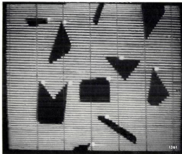
Fig. 4. Scanning of idealized particles, displayed on a monitor tube. Direction of scanning; right to left. The white dots are marker tags to indicate when a count has been made (see below). It will be noted that the indented particle (lower left) has been counted twice.
