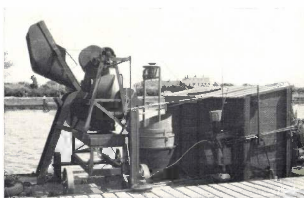
Fig. 10. Plant installed on a barge for preparing the tracer material 10 ). An ampoule containing radioactive ^{46}\text{Sc} , prepared in a nuclear reactor, is broken open and the contents dissolved in nitric acid in a vessel (not visible in the photograph). The solution is neutralized and diluted with water, after which it is conveyed by compressed air to the mixer shown on the left, which contains the appropriate quantity of "Ionac C 50". After some hours of mixing the ^{46}\text{Sc} is distributed uniformly enough amongst the grains. The contents of the mixer are emptied into the container on the right of the mixer, in which the tracer material is conveyed to the dumping site. The large bunker on the extreme right is filled with sand to protect workers on the barge against radiation. The whole installation is remotely controlled from behind this bunker.
