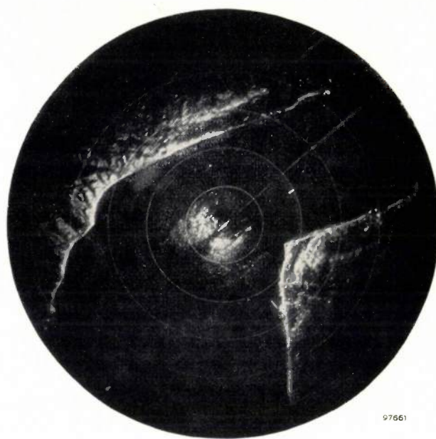
Fig. 16. Radar display of Straits of Messina, taken with the 8 GR 250; screen coverage set to approximately 5 km diameter ( \sim 2.7 nautical miles).
