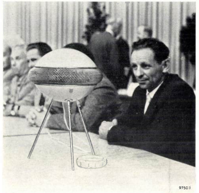
Fig. 19. One of the small omnidirectional loudspeakers ( A in fig. 17 ) that are placed on tables occupied by management, works council and press.
