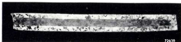
Fig. 4. Internally oxidized silver strip with 1.2 at. % magnesium. The strip was heated for 50 minutes in air at 800 °C and afterwards sectioned, polished and etched. The oxidation proceeding from the outside to the inside may be clearly seen: a "rim" covering about \frac{1}{4} of the thickness of the strip is oxidized, the interior is untransformed.
