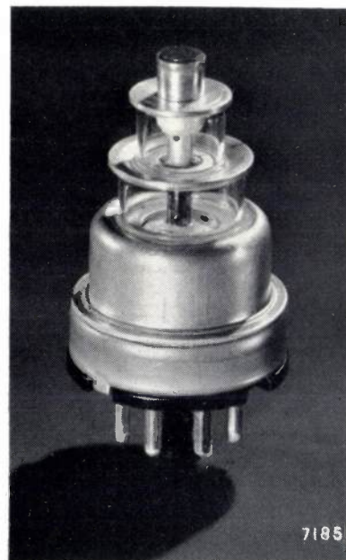
Fig. 9. "Disc-seal triode" type EC 56. Grid and anode are carried by metal discs sealed laterally into the glass wall; the outer part of the discs forms part of the resonant circuit.
