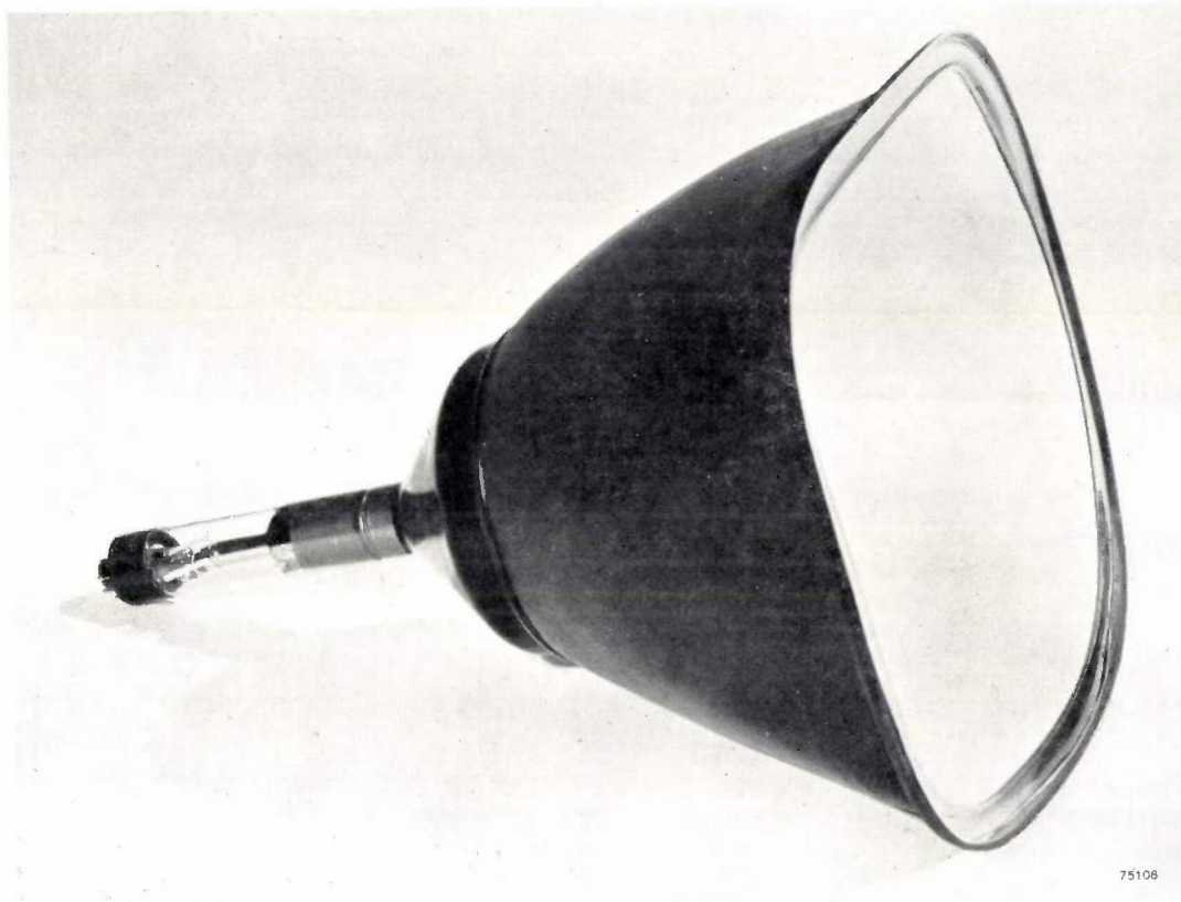
Fig. 4. Picture tube type MW 43-43 with rectangular window (diagonal 43 cm) and metal cone. During the course of 1953 the production will change over from chrome-iron to chromised steel as cone material.
