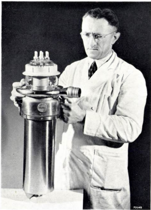
Fig. 8. Water-cooled transmitting tube for 100 kW output, with its anode water-cooling jacket.
