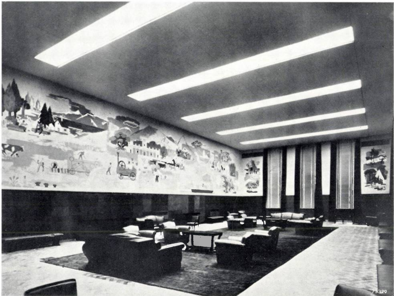
Fig. 3. Lobby of the Automobile Club of Argentine, Buenos Aires. The faces of the guests will constitute a horizontal zone of interest, whilst for relaxation a second horizontal zone of interest is found in the great mural. The concentration on this zone of interest is enhanced by the dark panelling underneath and the dark ceiling.
