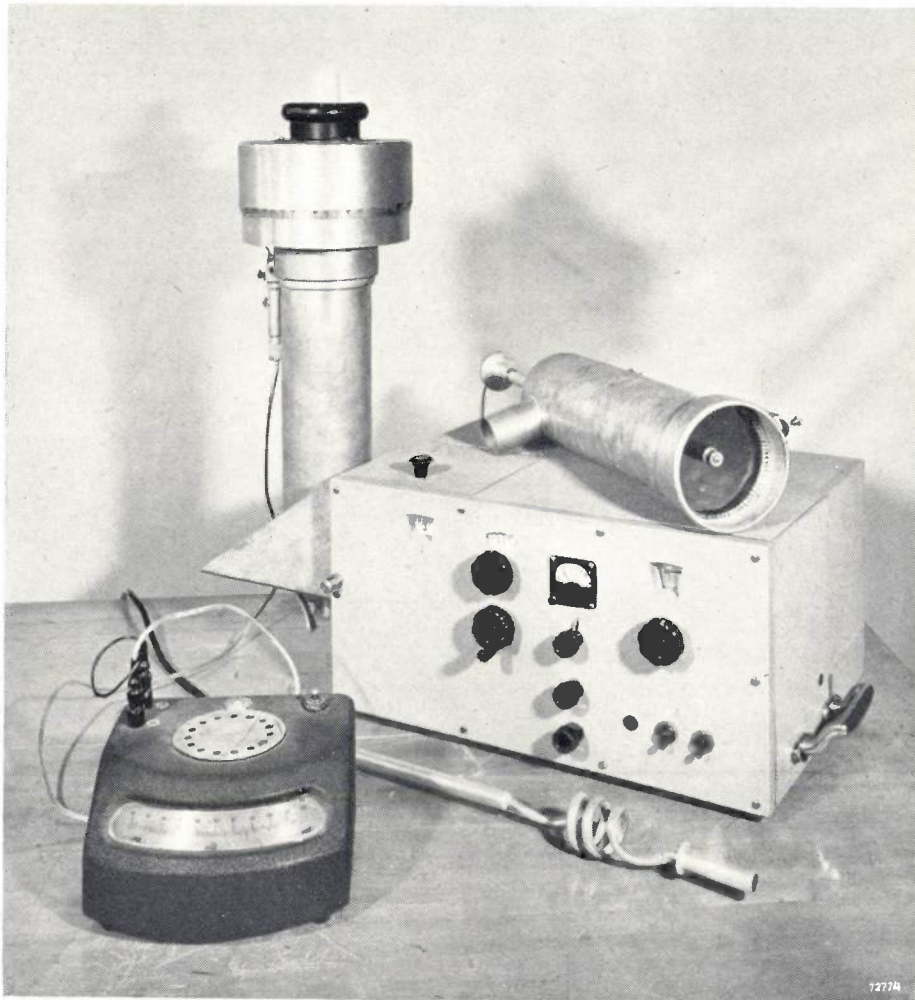
Fig. 6. Photograph of the equipment shown diagrammatically in fig. 5. At the right, the oscillator, on which is lying an open coaxial \lambda/4 line which is used in the range of 250-1000 Mc/s. At the end of the central conductor the electrically coupled detector can be seen. Standing at the left, a coaxial line with variable top capacitance, for frequencies of 5-100 Mc/s. To the left of this line is the electrically coupled detector. The helix in the foreground is the inner conductor of a line, in which the helix serves as lumped inductance (see text).
