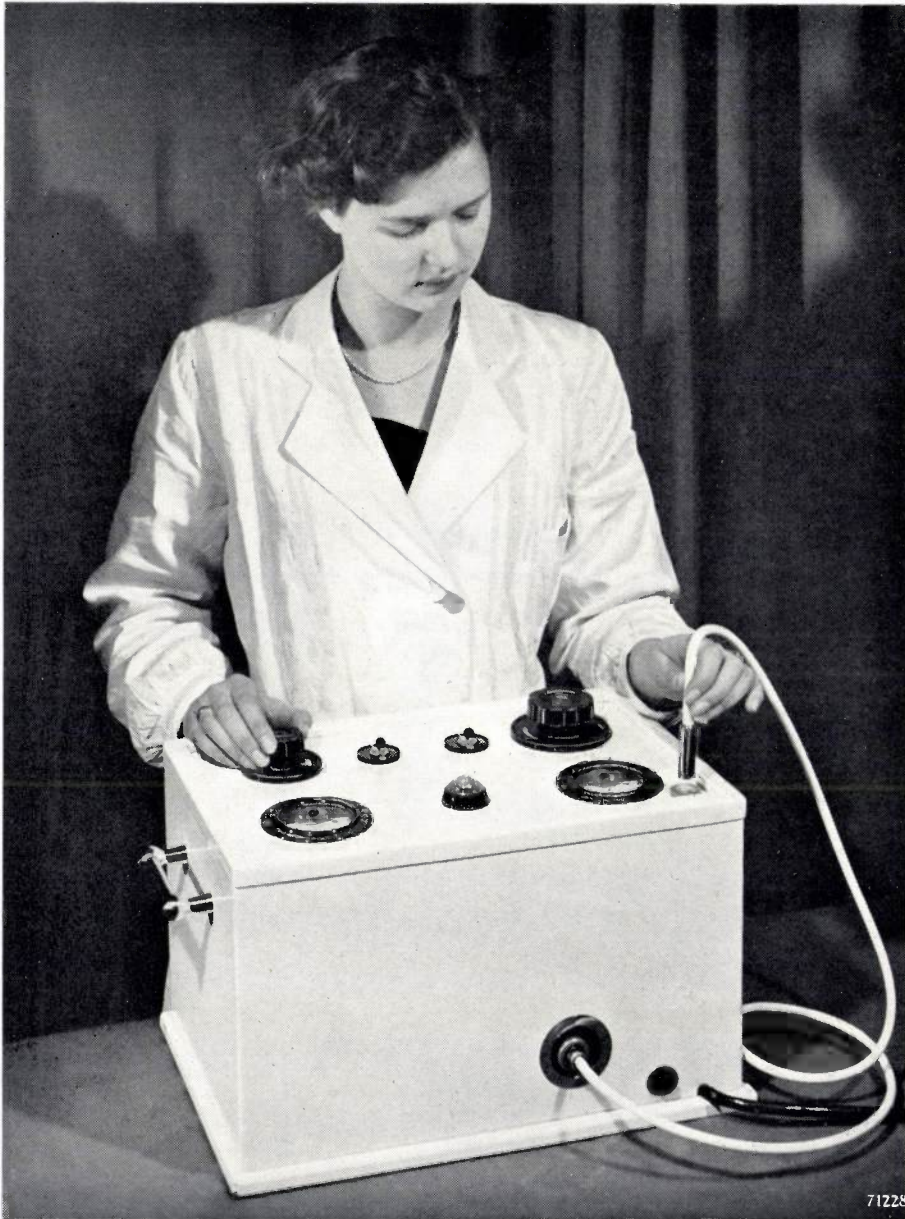
Fig. 10. The KT apparatus, ready for use. The tube current and the tube voltage are adjusted by means of the control knobs and meters. Note the connection of the "Podur" cable, with the midget KT tube at its end, to the apparatus. When not in use, this tube is housed in an opening in the apparatus.
