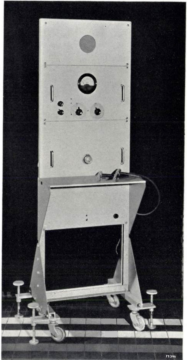
Fig. 4. View of the complete instrument. From top to bottom: loudspeaker panel, I.F. panel, H.F. panel, table (with the two probes) and supply panel.
