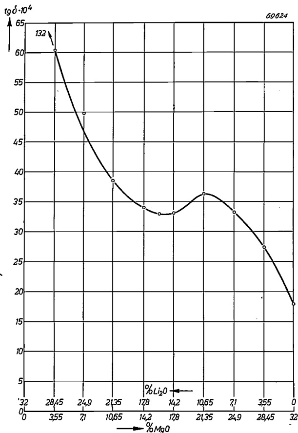
Fig. 13. Variation of \tan \delta at the frequency 1.5 \times 10^8 c/s and at room temperature for a series of glasses of the composition 53.3% SiO_2 , 10.2% PbO , 4.5% CaF_2 and 32% (Li_2O + MgO) , as a function of the MgO percentage. As described under fig. 4, when some of the Li^+ ions are replaced by Mg^{2+} ions, \tan \delta at first decreases, because the structure of the network is then more rigid. A further increase of the Mg^{2+} content reduces the rigidity of the structure and \tan \delta increases. This does not continue along the same line, in contrast to fig. 4, since the higher the Mg^{2+} concentration, the more Mg^{2+} ions begin to act as network formers. Then they no longer contribute to the relaxation losses, so that ultimately \tan \delta drops.
