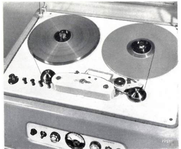
Fig. 7. Close-up of the top panel of the magnetic recorder depicted in fig. 6 . The components of the driving mechanism sketched in fig. 4 are easily recognized. At the front of this panel, on the left, will be seen the push-buttons for the control. The first of these (left to right) is for the rewind; rotation of the knob on the extreme left controls the speed, both forward and reverse. The second button starts the recorder at normal speed forward; this is the "playback" setting, seeing that the playback head is permanently connected to the amplifier (all amplifiers are of course previously switched on). The third push-button brings in the erasing head and recording head. To avoid the possibility of erasing part of a recording by depressing the button accidentally, this button is interlocked in such a way that it functions only when depressed together with the second button (which merely starts the machine). The fourth button returns all the others to neutral and stops the instrument by braking the motors.
