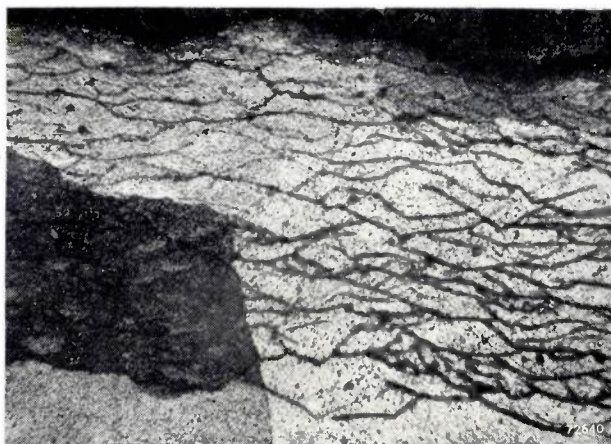
Fig. 7. Inner oxide films formed in copper with 5 at. % beryllium. The films run roughly parallel to the metal surface, the arrow indicates the direction of the oxygen diffusion.
