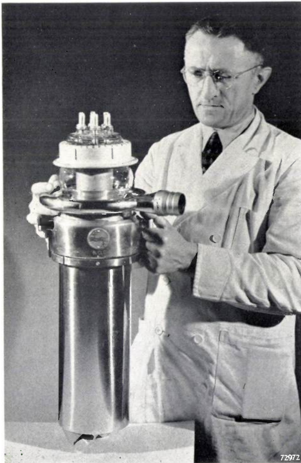
Fig. 3. a) The TBW 12/100 with "Grip-o-matic" water jacket. b) The same in cross-section. 1 filament connecting pins. 2 ring-shaped grid lead-in with upper anti-corona ring 3. 4 lower anti-corona ring, at the same time serving as handle and distributor of the air applied to inlet 5 for cooling the seals. 6 outlet holes for cooling air. 7 anode. 8 water jacket with water inlet 9 and outlet 10. 11 helical ribs. 12 self-sealing packing ring. 13 ring for locking the valve in the cooler.
