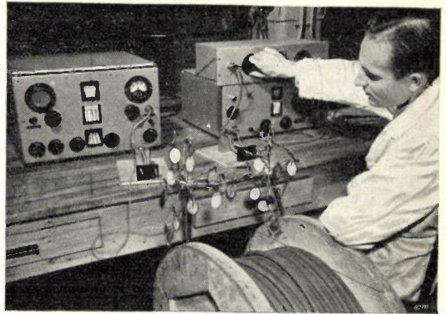
Fig. 12. Measuring the cross-talk damping between the pairs of conductors in a telephone cable. A certain voltage supplied by the generator (left) is applied to one pair of conductors. The resulting voltage on other pairs is measured (right) and must not exceed a certain value. Measurements are taken at different frequencies (100 to 500 kc/s).
