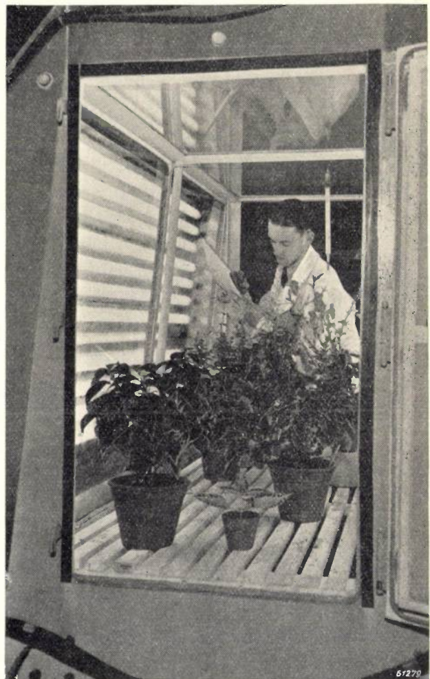
Fig. 3. A greenhouse with Coleus and Petunias. A TUV lamp ( d ) is to be seen between the TL lamps. The ultra-violet rays from this mercury lamp kill the algae which otherwise form a deposit on the glass panes along which the cooling water flows.
