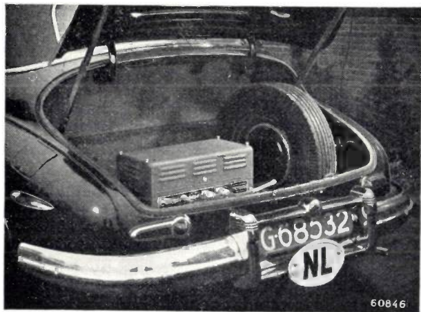
Fig. 9. Mobile transmitter and receiver, type SRR 192, in the boot of a motorcar.
