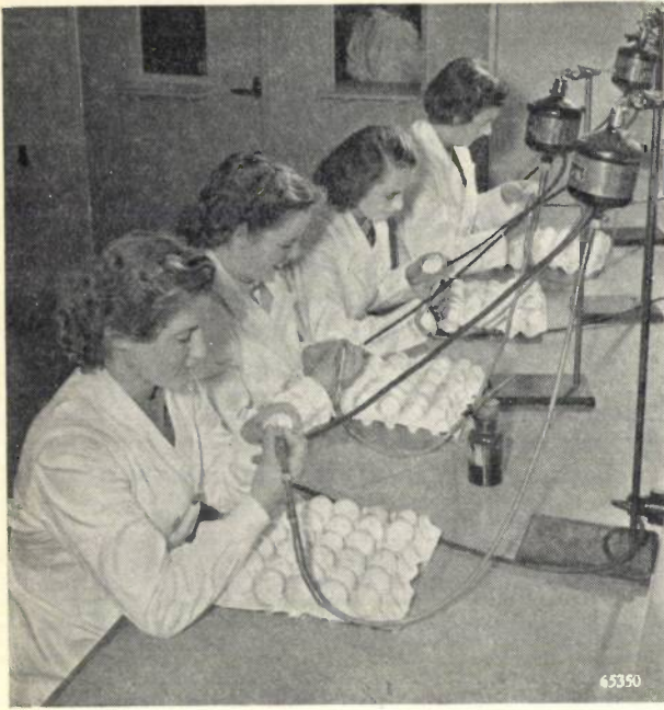
Fig. 5. The necessary holes are drilled in the eggs with a kind of dentist's drill.
