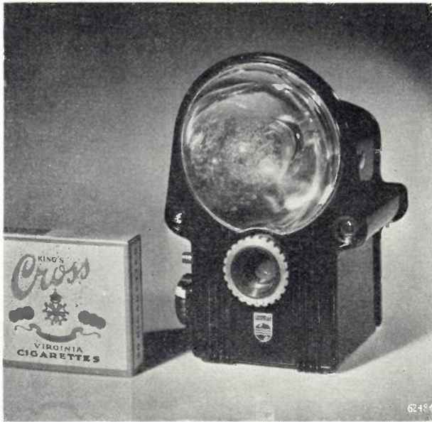
Fig. 5. Philips flash camera, type No. 5210. It contains a built-in reflector for a flashbulb. The camera is also fitted with a synchronizer, a pilot lamp for the lamp circuit, a plug socket for connecting additional flashbulb, and a compartment to take the battery for the ignition.
