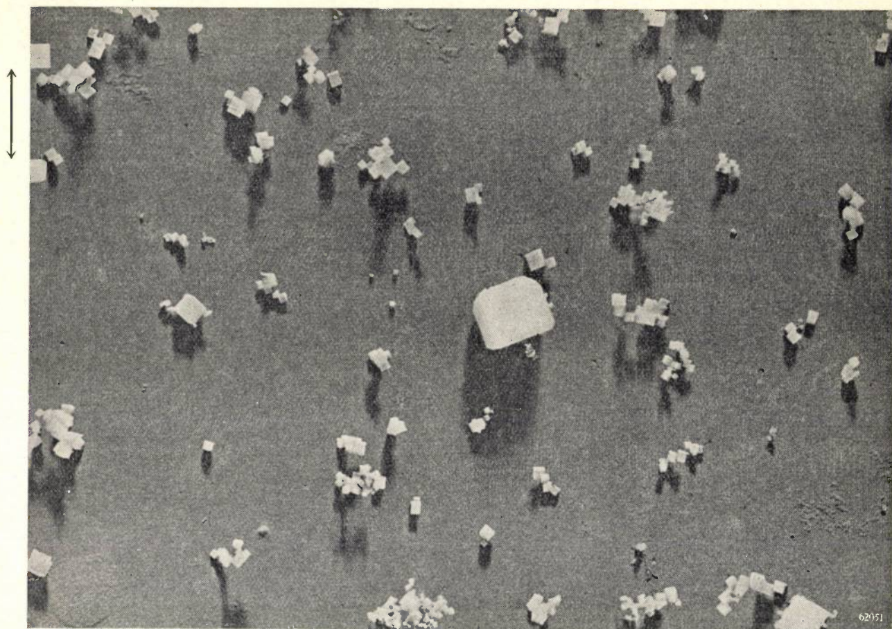
Fig. 17. Micrograph of magnesium oxide taken with the Philips electron microscope at a magnification of 18,000 times. The cube-shaped crystals lie on a film of "Formvar" and the whole is "shadowed" with a stream of uranium vapour. At the top on the left-hand side of the photograph are the two scale markings, the distance between which represents a length of 1 \mu . Photo b shows a detail of a at a magnification of 60,000 times.
