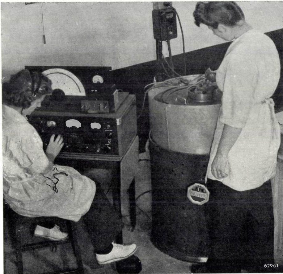
Fig. 7. Set-up of a planetary lap machine with apparatus for controlling the stopping point of the lap.
