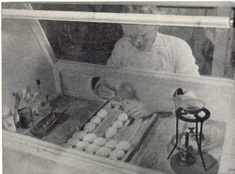
Fig. 12. Inoculating eggs with a highly infectious material, as carried out in the Institute for Tropical Hygiene at Amsterdam. The germicidal lamp is of particular importance here for safeguarding the laboratory workers.
