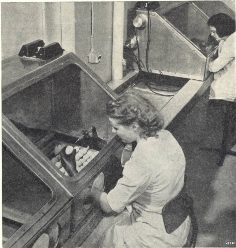
Fig. 6. The case, kept sterile with TUV lamps, in which the incubated eggs are inoculated with the virus to be cultivated. The glass top does not allow the rays of the 2537\text{ \AA} wavelength to pass through. The arm holes can be moved a little to the side to provide a comfortable position for the assistant's arms.
