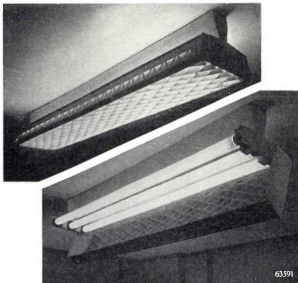
Fig. 10. Top: Fitting for four "TL" lamps of 40 W provided with rhombic louvres with screening angles according to fig. 9 . This type of fitting was employed on a large scale for the lighting of the new head offices of the Rotterdam Bank at Rotterdam. Bottom: The same lamp fitting opened.
