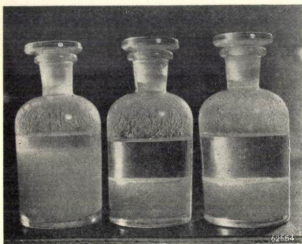
Fig. 3. The settling of a suspension of quartz in toluene. From left to right: after 5 seconds, 10 hours and 2 weeks respectively. In this unstable suspension the particles flocculate immediately and the liquid clears after a short time. Note the "buttermilk effect" on the inside of the flask.
