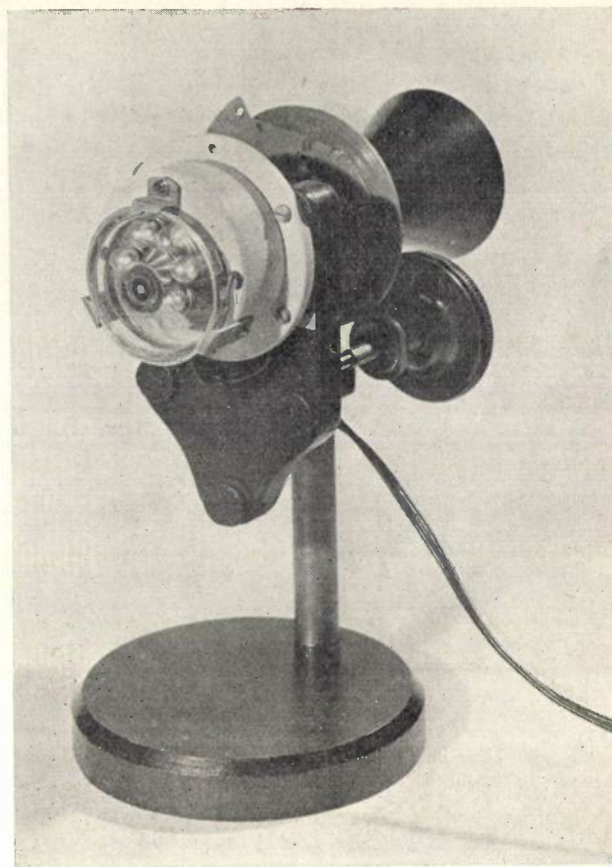
Fig. 7. Microscope set-up used for measuring the extent to which the skin bulges out when shaving with a dry-shaver. The shaving cap is centred in the round glass cap at the front of the apparatus, and is illuminated from the inside by a number of small lamps placed in a circle round the objective. The microscope eye-piece is inside the cone on the right-hand side of the apparatus. The observer focuses the microscope onto the inner face of the shaving cap along which the cutters run, and then onto the skin; the displacement gives a measure for the bulging of the skin.
