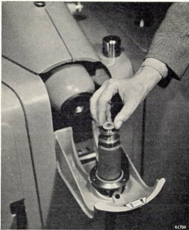
Fig. 7. Replacement of the filament. The removed cathode cap is seen standing on the desk above the man's hand.
