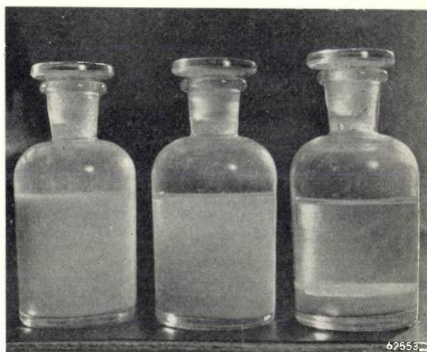
Fig. 2. The settling of a suspension of quartz in water. From left to right: after 5 seconds, 10 hours and 2 weeks respectively.
