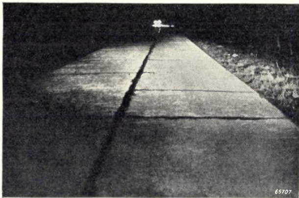
Fig. 10. When two cars are about to pass, a tall object on the right-hand side of the lane can sometimes be observed from a great distance owing to it standing out as a silhouette against the patch of light thrown on the road by the oncoming car. (Taken from V. J. Roper, Ill. Eng. 34, 1073, 1939.)
