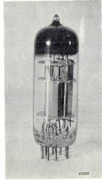
Fig. 2 Combined pentode and triode for television reception, type ECL 80.
