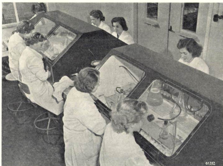
Fig. 8. Case, sterilized with TUV lamps, in which the cultivated virus is extracted from the eggs. Each of the assistants working at the case uses a pipette, connected to a suction pump, with which the liquid is drawn out of the allantoic cavity of the "decapitated" egg into the flask standing in the middle of the case. This flask can hold the culture taken from 300 eggs. In each suction line is a small intermediate flask which has to be inverted after every fourth egg for its contents to be transferred to the big flask. If one of the eggs happens to be a failure (for instance through a blood vessel bursting) the intermediate flask is replaced by a clean one, so that the contents of the big flask are not spoiled.
