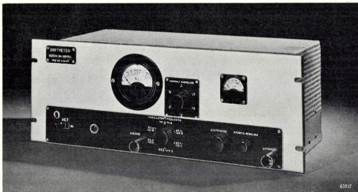
Fig. 7. Frequency-drift meter, in a form suitable for mounting in a rack. The left-hand meter, calibrated in kc/s, is used for preparatory adjustments; the recording meter is not shown in the illustration. The right-hand meter is used to check the various grid currents selected by the knob in between them. Underneath is the knob for selecting the desired reference frequency ( n = 19 \dots 28 ), cf. fig. 4.
