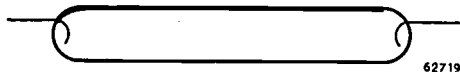
Fig. 3. Schematic cross section of the new "TL" lamp ("TL" S lamp) with conducting strip on the inside of the glass tube making contact with one of the electrodes.
