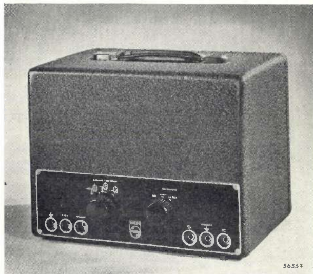
Fig. 8. The pre-amplifier GM 4570, which is suitable for the arrangement according to fig. 7. Gain 4 times or 20 times.
