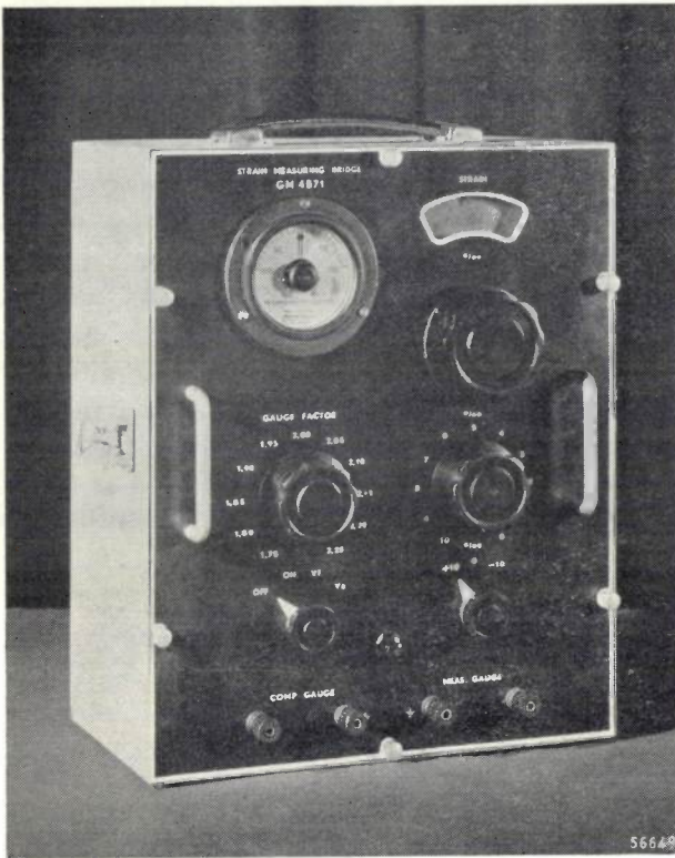
Fig. 5. Measuring bridge (GM 4571) using the zero method for measuring static loads. To the right, one above the other, three knobs for balancing the bridge; to the left, from top to bottom, the indicator, the correcting knob for the gauge factor of the strain gauge, and the knob for switching on and off, acting at the same time as the switch by means of which the indicator can be used for checking the batteries.
