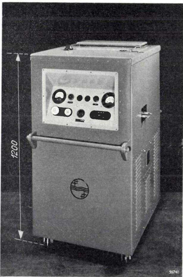
Fig. 9. Generator for high-frequency induction heating, type SFG 136/00. On the right the connections for the work coil. Maximum power in the workpiece 2 kW, frequency 1.2 Mc/s. The apparatus is equipped with one transmitting valve TB 3/2000 and two rectifying valves DCG 5/5000. Height indicated in mm.
