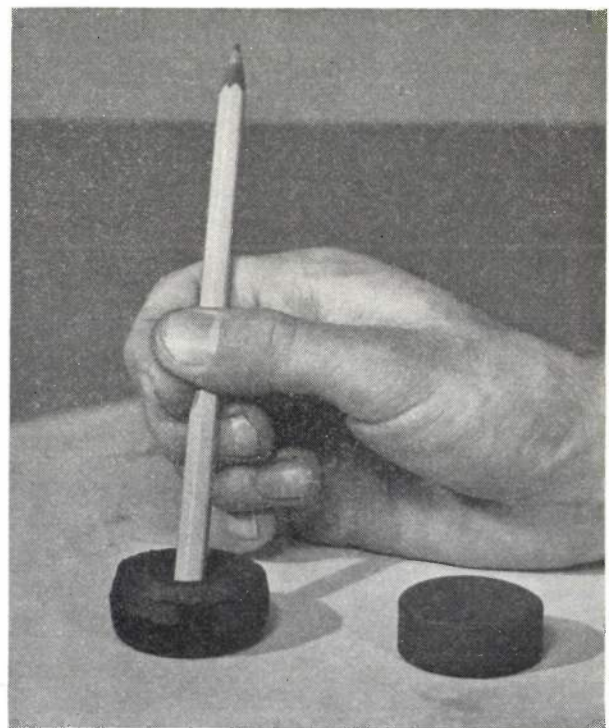
Fig. 8. Two thermosetting plastic pellets. The left-hand one has been made plastic by preheating and is ready for moulding.
