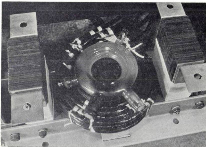
Fig. 6. a) The betatron illustrated in fig. 5 with the upper part of the yoke and the upper coil and pole piece removed. (For practical reasons each coil was composed of four parallel-connected parts; this explains the large number of cables seen at the back.) b) Here the accelerating tube has also been removed, showing the peculiar shape and construction of the pole piece.
