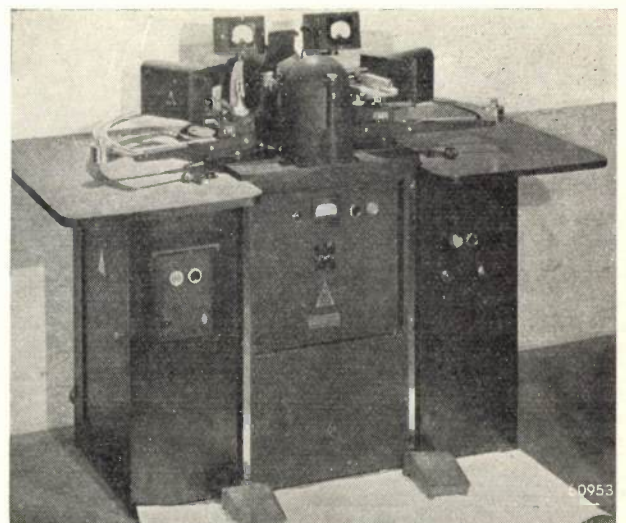
Fig. 8. The complete X-ray diffraction apparatus of the North American Philips Co. for quartz-plate manufacture. The instrument is provided with two independent measuring tables which can be seen here to the left and right of the X-ray tube. Under each measuring table is the supply apparatus for the counter tube, in the middle cabinet the supply and controls for the X-ray tube.
