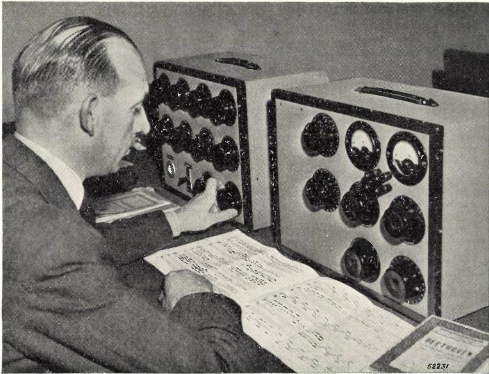
Fig. 7. The "music pilot" at work. He regulates the compression guided by the music score in front of him. By means of the other controls seen in the photograph the signals from the microphones set up in the hall can be mixed in the right proportions.
