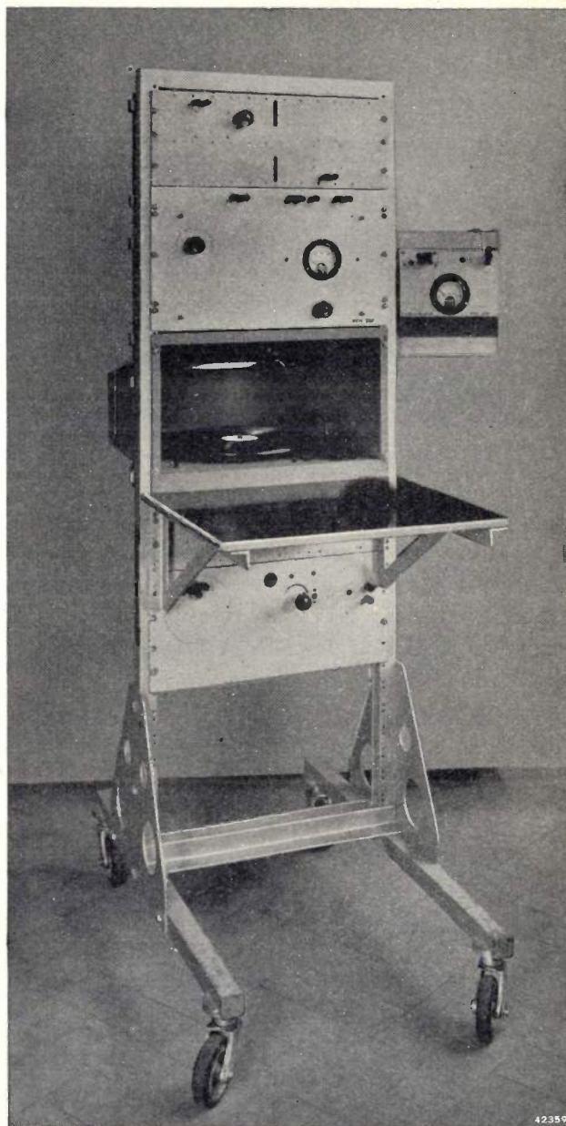
Fig. 8. Transportable equipment for cross-talk measurement. Top: the psophometer 6) ; below: the play-back apparatus for the speech records. On the right: the volume-meter.
