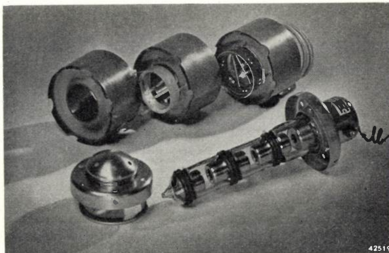
Fig. 4. A Philips three-stage gas-filled rectifier valve for 125 kV; a) assembled and b) taken apart. The glass tube is surrounded by ring-shaped "Philite" condensers (see C in fig. 3). The tube is calculated for oil immersion of the rectifier. The length is more than 20 cm, the diameter of the condensers is almost 9 cm. When used in air, in order to avoid flashover along the outside of the glass wall, a greater insulation distance between the electrodes would be necessary, thus in general a longer length of tube.
