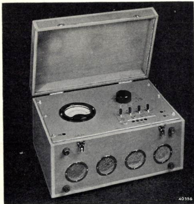
Fig. 7. Level indicator, mounted in a robust wooden box. The construction, as indeed that of all the equipment described, must be extremely rigid to avoid distortion of the chassis, buckling of the front panel etc. and thus exclude any possibility of consequent changes in the electrical properties.
