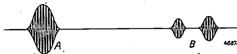
Fig. 3. The transmitted signal A and the reflected signals B in the determination of the effective altitude of the ionosphere according to the method of Breit and Tuve.
