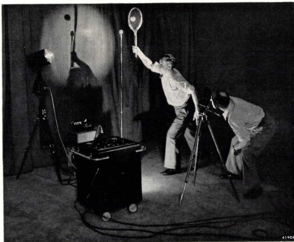
Fig. 5. Arrangement for photographing the collision between tennis ball and racket with the help of the stroboscope. The illumination is synchronized by means of a microphone.
