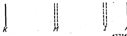
Fig. 1. Diagram showing the principle of a velocity modulated tube. K cathode, M grids of the modulator between which the electrons are modulated in velocity by an A.C. voltage. Between M and I is a field-free space for overtaking, in which velocity-modulation is converted into density-modulation; I inductor to which density-modulated electrons give off their high-frequency energy.
