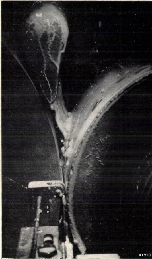
Fig. 13. Cooling of a centreless grinding machine. The lubricant is blown aside by the wind from the rotating grindstone.
