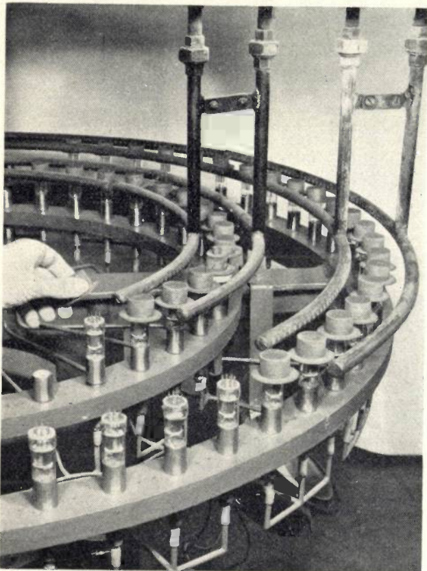
Fig. 3. Detail of the sealing machine on which bulb and base plate are joined. A metal cap is placed on the base plate (left). The whole passes between two rows of gas flames, the layer of glaze being heated to about 450° C, necessary for fusing.
