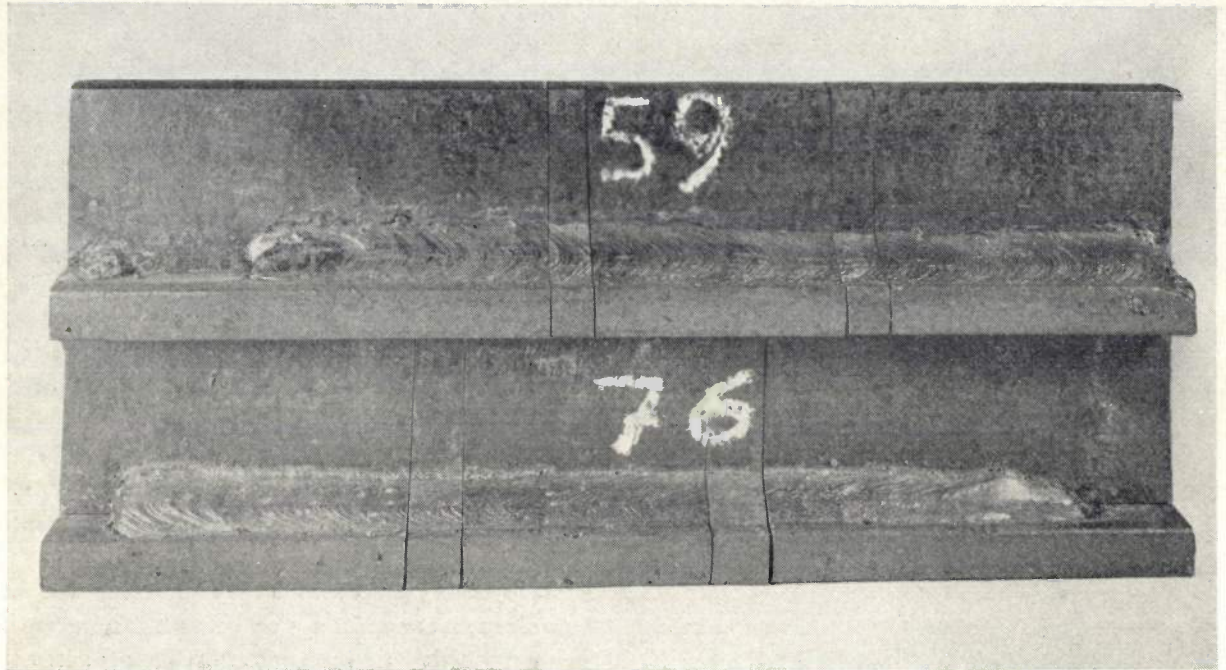
Fig. 6. Photographs of fillet welds made in the flat position with Ph 55-7 (No. 59) and with Contact 15-5 (No. 76). In No. 59 the undercut can be seen under the figure 9, while No. 76 shows no faults at all.
