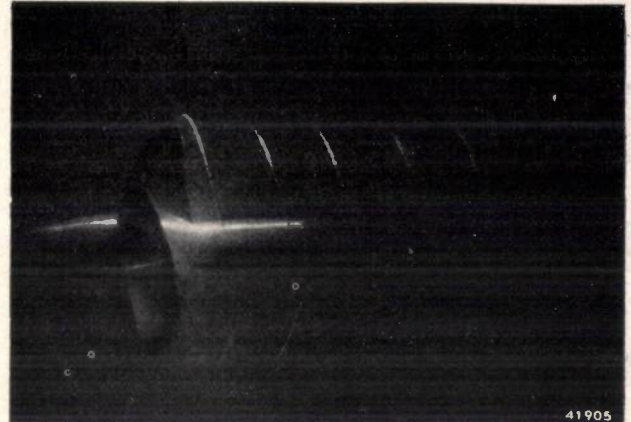
Fig. 8. Ship's screw in cavitation tank. a) Strong cavitation, b) no cavitation. The bright line in b) indicates the top spiral of the screw. The photographs were taken in the Naval Shipbuilding Testing Station in Wageningen.
