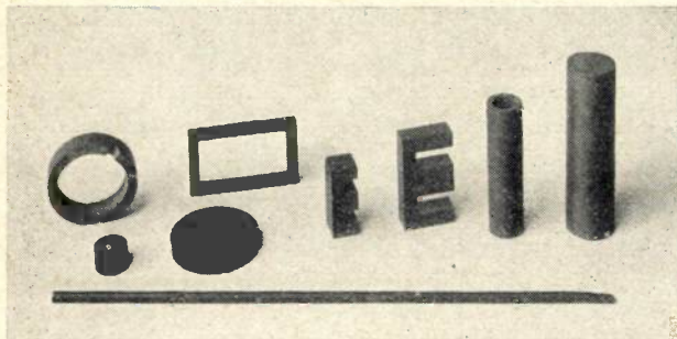
Fig. 2. Some specimens showing the shapes in which component parts of "Ferroxcube" can be made. The disc, ring and E-shaped pieces are moulded by dry compression of the basic material in powder form; the rod and tube-shaped pieces are formed by adding a binder to the powder and pressing the mass through a circular opening.
