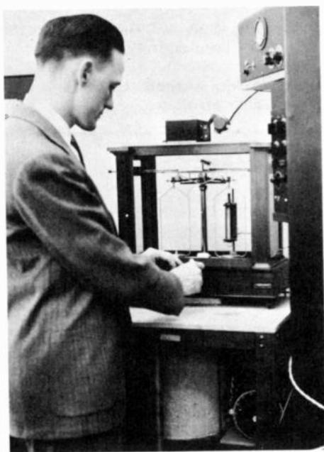
Figure 1. Adjusting the Recording Analytical Balance Recently Developed at the National Bureau of Standards
