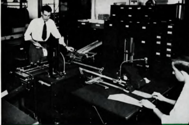
▲ ADDRESSOGRAPH EQUIPMENT—Time cards, payroll sheets and pay checks are printed by Paul Graefe (left) and Anthony Jagielski.
