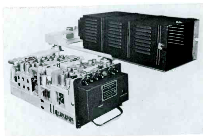
Figure 5 — DIA DME without dust cover showing upper portion.
