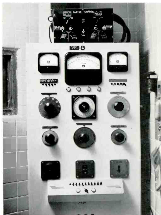
Figure 4 — Control Booth. An arrangement satisfying manual requirements of the circuitry. Presetting areas of dynapulse controls, program selector and power supply for the second tube are not illustrated.
