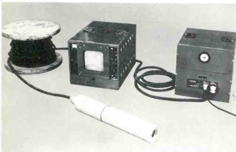
Figure 4 — Diamond Underwater Television System uses Vidicon camera pickup tube in a watertight housing for relatively shallow water work. This system is used effectively at depths up to 500 feet. Other Diamond cameras using the Image Orthicon camera pickup tube in a pressurized waterproof housing work effectively at depths of 1000 feet.
