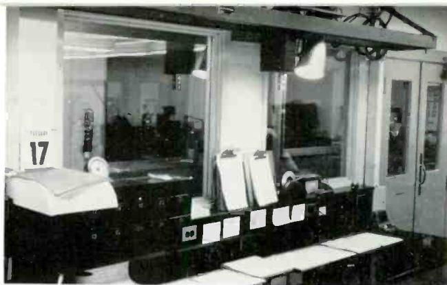
Figure 1 — Remote operated television camera scans Laboratory Reports, on table, to provide Paper Machine Superintendent with in-process quality control data.
