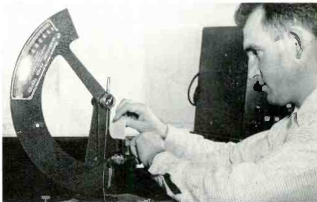
Figure 2 — Information feed-back cycle begins with paper testing. Elmendorf Paper Tester provides tear strength data as shown on scale. Via closed-circuit camera this information is relayed to Paper Machine Superintendent who directs adjustment of a Jordan Pulper.
