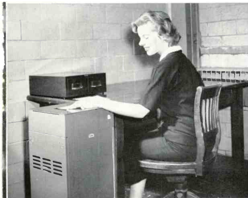
Figure 6 — A television camera inside the Dumont camera stand views a signature card placed face down on its glass top, at the Denver U. S. National Bank.
