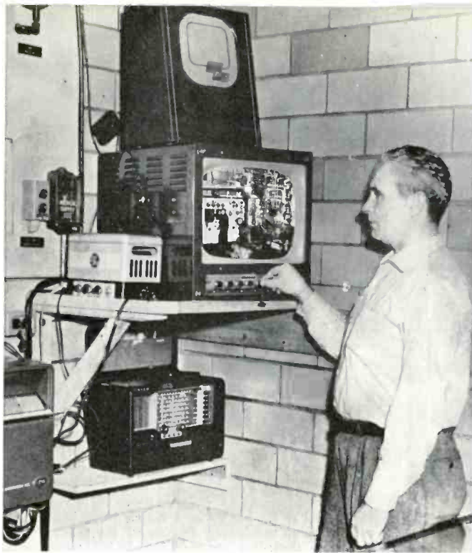
Figure 5 — Shift foreman at Esso Research and Engineering Company pilot plant at Bayway, New Jersey, checks safety of workmen on job at unit 300 feet away via GPL closed-circuit television system.
