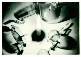
Early Machlett tubes—of the Jackson type. The anode is directly in line with the cathode and bears a target set to receive the full stream of electrons and angled to direct the shower of x-rays to one side. Other protuberances from the tube are incidental to creating or maintaining a vacuum.
