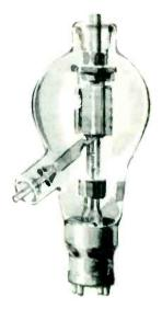
The 6C21 pulse modulator tube, heart of the transmitter in early-warning and gunlaying radar systems, was Machlett's first big assignment in defense production work. In the modern form of the straight-line exhaust system, tubes are mounted on moving dollies equipped with mechanical and diffu-
