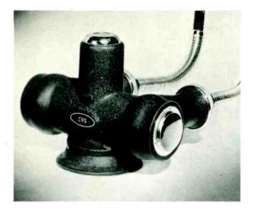
The CYS tube was an innovation in design —half the size of previous ray- and shockproof tubes. It had the added advantage that the insert could be readily changed.
