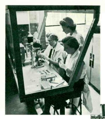
All-but-automatic exhaust apparatus for the 2C39A tube requires only general supervision —but it has to be very intelligent supervision.
