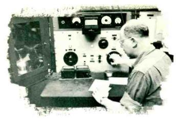
A power tube, at left, glows behind safety glass as it is put through gruelling, instrument-recorded tests.
