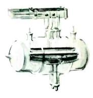
sion pumps which keep the tubes under continuous high vacuum as they progress through the final stages of exhaust and seal-off.
