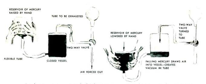
It took a strong man to operate the Geissler mercury vacuum pump, here shown in schematic diagram.
