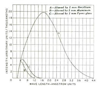
Beryllium transmits a far greater intensity of xradiation at longer wave-lengths than other practicable materials. Curve A shows intensity transmitted by 1 mm. thickness of Beryllium. Curve B, 1 mm. of Aluminum; Curve C, 1 mm. of Pyrex Glass.
