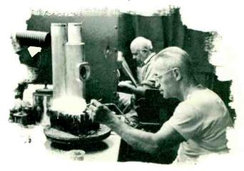
In the fabrication of aluminum housings for high-voltage x-ray tubes, shown here, operators take unremitting care to achieve an absolutely sound bond between aluminum components and shockproof housings.
