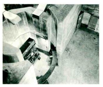
A Betatron in position, surrounded by great shielding walls of concrete to guard against uncontrolled radiation. The Donut is between the two curved-edge parts at left center of the apparatus. Patients are wheeled into position right by the Betatron, for deep x-ray treatments made possible by the accurately localized dosage produced by this remarkable apparatus.
