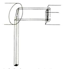
In the line-focus principle, the filament (right) emits a stream of electrons which is focused by the shaped walls surrounding it into a beam that is broad yet thin, like a board standing on its edge. This thin beam strikes a target set at an angle of about 20°. So the spot on the target is foreshortened, as seen from outside the tube, into a very small square. This square is the "focal spot" of the x-rays that emerge from the tube. The smaller it can be made, the sharper the x-ray picture.
