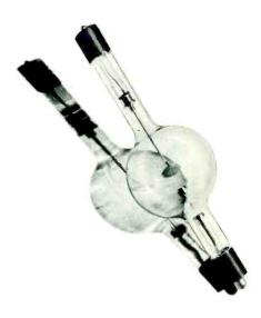
A therapy x-ray tube of the Coolidge type made by Machlett in the early 1930's. Note the light target, supported on a slender stem. Heavy copper anodes were yet to come.
