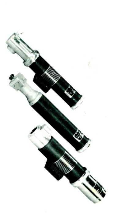
Typical beryllium-window x-ray tubes of the present day. Upper and lower tubes (Types OE6-50 and OE6-60) are oil-immersed, hermetically sealed, shockproof tubes for medical, research, and industrial uses. Middle tube (Type A-2) is a type expressly made for crystal analysis and other applications of x-ray diffraction phenomena.
