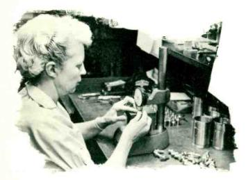
Purchased parts are inspected on receipt and tested with micrometers and other precision measuring equipment before being put into stock.
