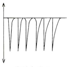
Effect of valve tubes on Ruhmkorff coil current.
