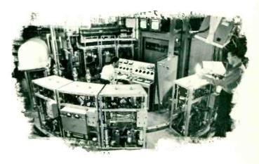
Newest version of the mobile exhaust system is an endless-track circuit. Tubes being sealed into pump—bearing dollies at right, progress through outgassing stages accurately controlled from the instrument board at center.
