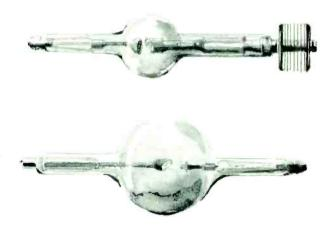
Coolidge tubes handled by Machlett as distributor about the time of World War I. Upper, a diagnostic tube "recommended for fluoroscopy and radiography only. It should never be used for therapy." Lower, "For treatment and general picture work." the recognizably greater power, penetration, speed and simplicity of the Coolidge tube were undoubted advantages, many radiological authorities held that for certain uses the gas tube was superior.
