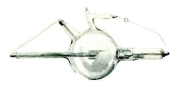
The Bellevue tube for interrupterless transformer current in the form made by Machlett from about 1912—the small spear-point projecting from the face of the anode produced, in some degree, the effect of a valve or rectifier, to suppress some of the inverse impulses necessarily inherent in the alternating current then necessary to produce high voltages in x-ray equipment.
