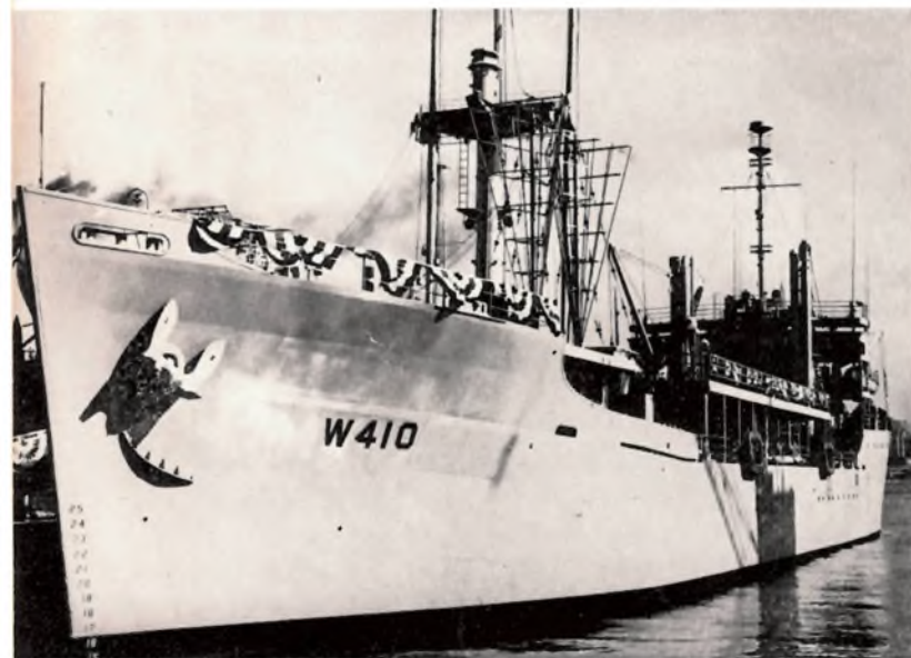
Figure 6 — The Voice of America's floating radio station "Courier." Some of the special antennae can be seen in this view. From the raised platform amidships captive barrage balloons may be released to carry antennae hundreds of feet above the ship.
