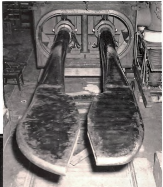
Figure 4 — The two semi-circular hollow electrodes called "dees" because of their shape. Radio-frequency voltage between the dees accelerates the ions into the interior of the dee which at that moment is negative.
