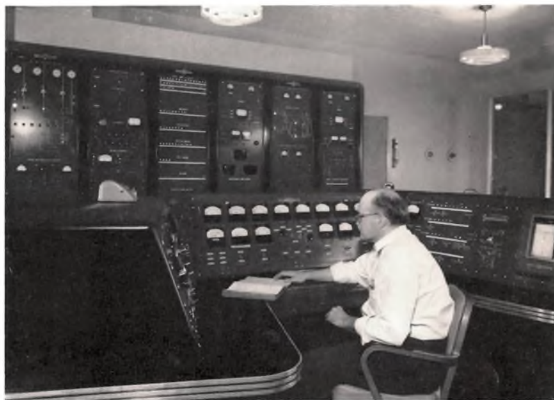
Figure 7—Control room from which the cyclotron is operated. The cyclotron is housed in a vault with concrete walls seven feet thick to protect the operators from lethal quantities of nuclear particles.
