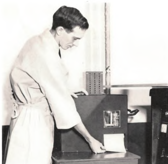
Figure 9 — Counts are accumulated for 30 sec. in three decade circuits and then transferred through stepping relays at the end of the count time to three printing wheels and recorded on tape.
