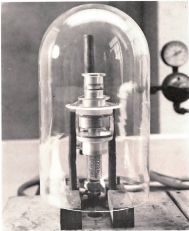
Figure 4—ML-6256 final seal-in operation by induction heating.
