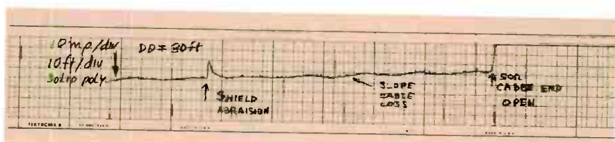
Figure 12. 1502 strip chart showing cable discontinuities at points "A" and "B" (see figure 11).
