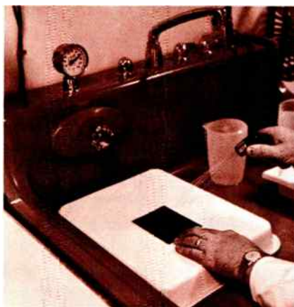
Figure 2. The resistor pattern can be seen emerging from the stencil film as the unexposed area is rinsed away. Using the temperature blender in the background, a steady water temperature of 110° is maintained.
