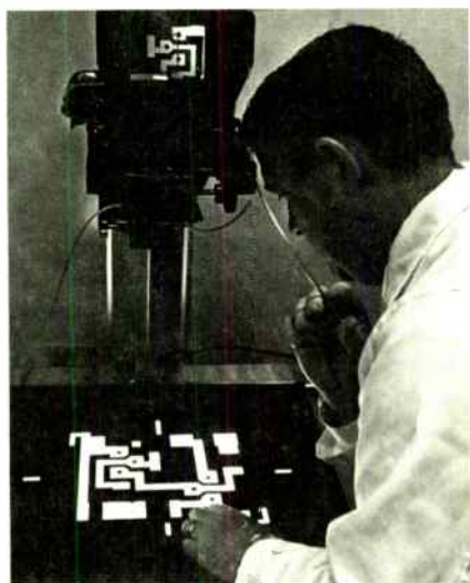
Figure 3. Photographic reduction of the circuit design is an indispensable part of any microelectronic technique.
