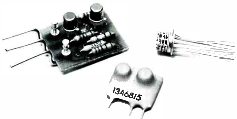
Figure 7. Lenkurt-built negative resistance (left) for channel filter studies compared to Centralab package and Sylvania IC version. About actual size.
