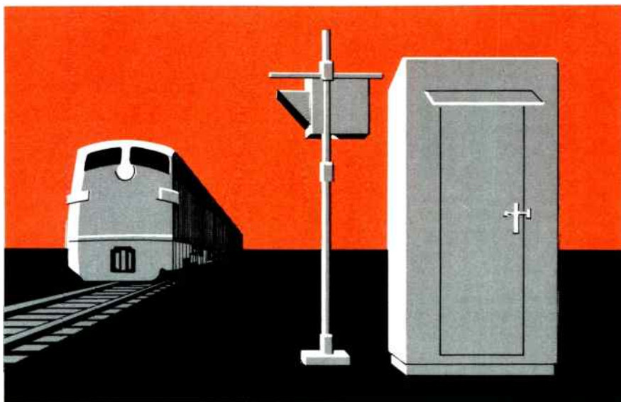
Figure 4. Mounted at trackside so as to provide maximum view of the passing trains, the scanner covers a vertical area of just under nine feet. Its protective housing allows the scanner to operate at temperatures ranging from -50^{\circ} to 150^{\circ} Fahrenheit.
