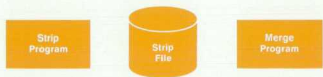
Fig. 3. Using available compiler information, two programs and a data file were developed to provide useful symbolic debugging capability to driver writers who do not have HP-UX source licenses.
