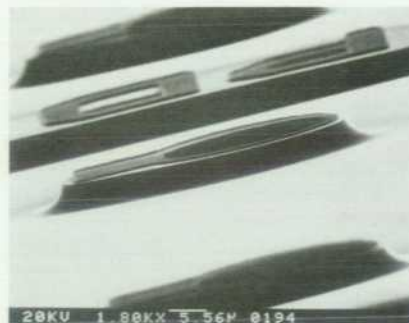
Photodiode Mesa Surface 1:1:1 (1N)K_2Cr_2O_7:CH_3COOH:HBr
