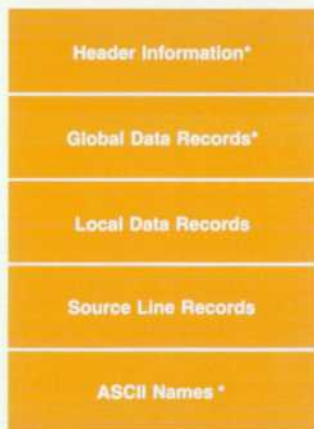
Fig. 1. Debug section of an HP-UX object module.
