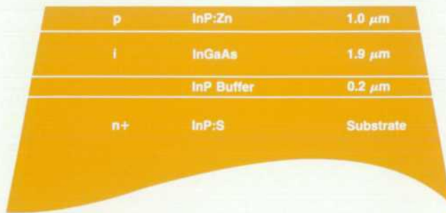
Fig. 2. Photodetector epitaxial structure (not to scale).
