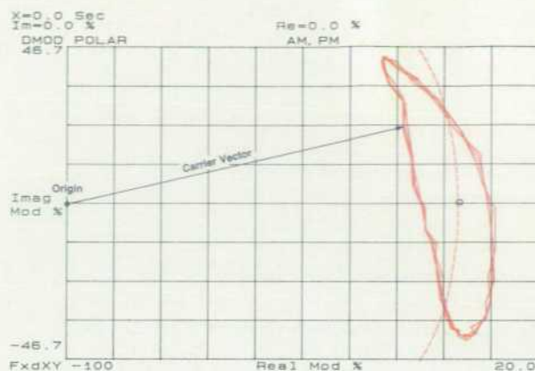
Fig. 4. Demod-polar plot. Approximately three cycles of the locus of the tip of the modulated carrier vector are shown after ten demodulated time record averages. The dashed line shows the locus of constant carrier amplitude. The marker on this line shows the zero phase point, corresponding to an unmodulated carrier.
