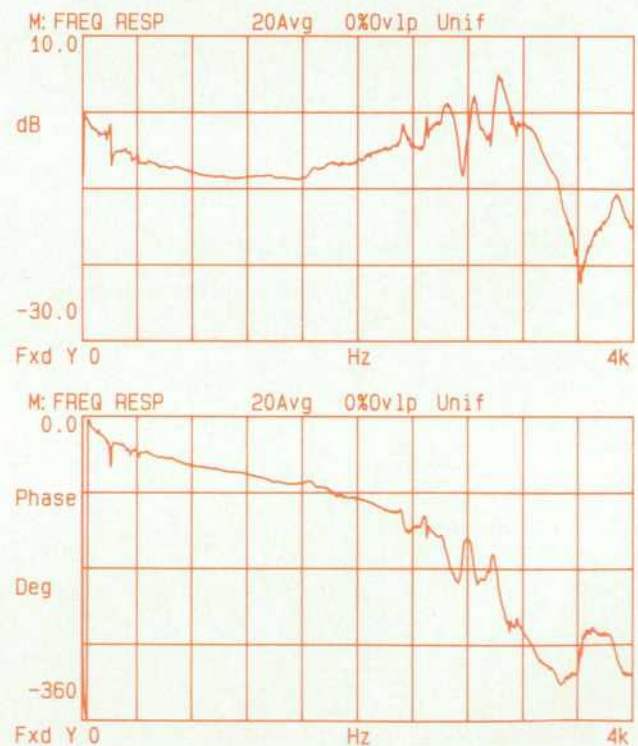
Fig. 12. Compensated open loop system response.
