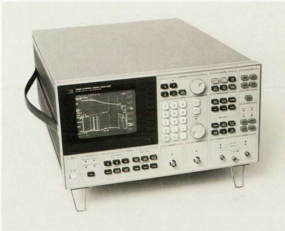
Fig. 1. The HP 3562A Dynamic Signal Analyzer performs fast, accurate network, spectrum, and waveform measurements from dc to 100 kHz. Measurements include power spectrum, histogram, frequency response, and cross-correlation. These can be performed in real time or on stored data. Built-in analysis and modeling capabilities can derive poles and zeros from measured frequency responses or construct phase and magnitude responses from user-supplied models. Direct control of external digital plotters and disc drives allows easy generation of hard copy and storage of measurement setups and data.
