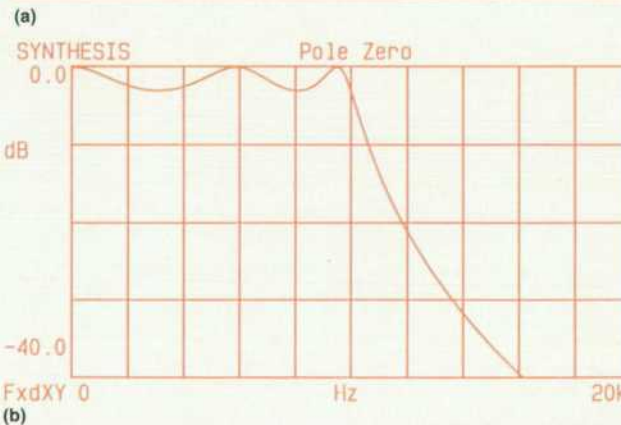
Fig. 4. (a) Table of ten poles obtained by curve fitting equation 5. (b) Response obtained by discarding right-hand poles listed in (a) and resynthesizing the resulting pole-zero function.
