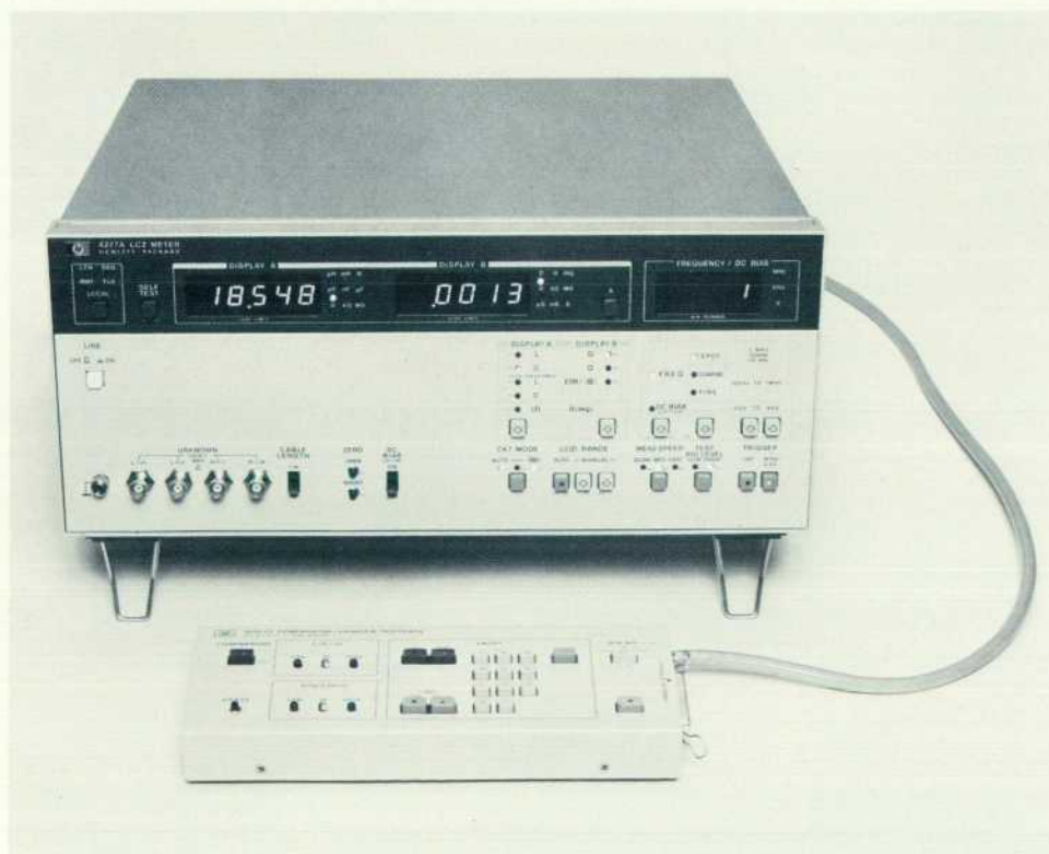
Fig. 1. The HP 4277A (shown here) and 4276A (Fig. 2) LCZ Meters perform accurate high-speed measurements of impedance parameters of components and materials at frequencies from 100 Hz to 20 kHz (4276A) or 10 kHz to 1 MHz (4277A). By adding an optional comparator/component-handler interface (shown in the foreground), they can be operated in a stand-alone configuration for low-cost, high-speed production-line testing or incoming inspection.
