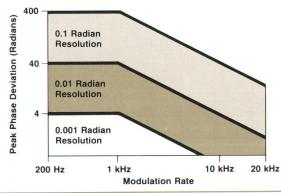
ACCURACY:<sup>2</sup> +3% of reading ±1 digit. DEMODULATED OUTPUT DISTORTION: <0.1% THD. AM REJECTION (for 50% AM at 1 kHz rate):<sup>2</sup> <0.03 radian peak in a 50-Hz-to-3-kHz BW.
