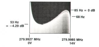
**Fig. 5.** Oscilloscope display from the setup of Fig. 4. Ac input to the VCXO was adjusted to give 100-Hz deviation at the low end of the VCXO's tuning range. The display shows how the actual deviation varies as the VCXO is tuned across its band.
