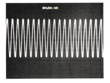
**Fig. 2.** AM recovered by the 8901A modulation analyzer from the signal of Fig. 1 is a single-frequency sine wave.
