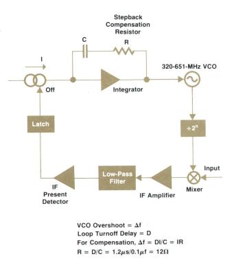
**Fig. 8.** Sweep loop, controlled by the microprocessor, tunes the octave oscillator rapidly across its band, looking for an input signal. When an IF signal is detected, the sweep stops. The stepback resistor compensates for the oscillator's overshooting the input frequency during the time it takes to stop.
