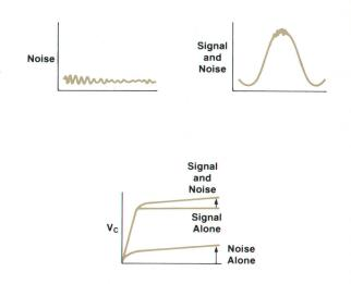
Fig. 3. Effective noise during peak detection.
