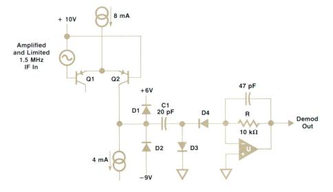
in the pulse duration that limits noise performance. In contrast, the charge-count circuit requires only that a dc voltage be accurate and stable.
