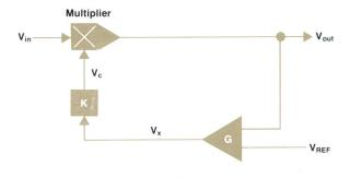
Fig. 12. AGC loop can be modeled as a feedback loop around a multiplier.
