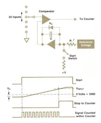
**Fig. 15.** Analog-to-digital converter is used to measure many voltages in the modulation analyzer. It is a single-slope converter, counting a clock signal while a constant-slope ramp voltage rises to the level of the unknown voltage.
