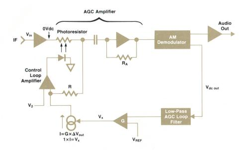
**Fig. 11.** Automatic gain control (AGC) circuit provides a constantlevel IF, signal to the AM demodulator. A low-distortion photoresistor is the gain control element.
