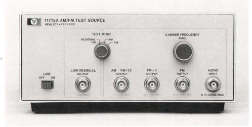
**Fig. 1.** Model 11715A AM/FM Test Source provides AM and FM signals of sufficient flatness and linearity to characterize the 8901A Modulation Analyzer. test source contains two oscillators. A crystal oscillator generates the low-residual-FM output. This oscillator is followed by a full-wave frequency doubler and appropriate filtering. The output residual FM is much less than 0.1 Hz in a 50-Hz-to-3-kHz bandwidth.
