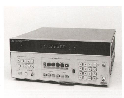
Fig. 1. Model 8901A Modulation Analyzer measures a signal's frequency, drift, power, AM, FM, and residual noise. It also recovers the modulating signal. Its carrier frequency range is 150 kHz to 1300 MHz and its modulation depth or deviation measurements are generally accurate within one percent of reading.
