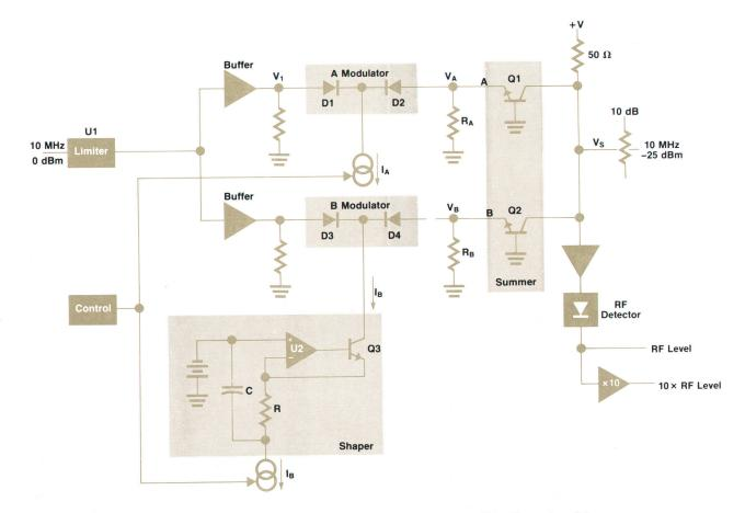
**Fig. 4.** AM calibrator circuit diagram. The 10.1-MHz signal from the FM calibrator is split into two identical paths. The signal in one path is switched on and off, and the two paths are then summed.
