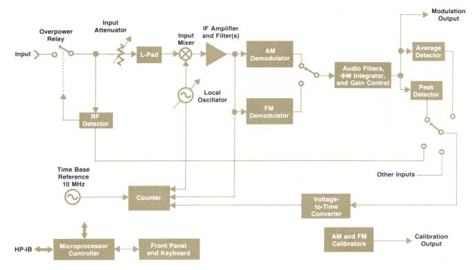
**Fig. 3.** Simplified block diagram of Model 8901A Modulation Analyzer. Basically a calibrated receiver, the analyzer down-converts the input signal and then recovers either the amplitude or frequency modulation regardless of which is the dominant type.
