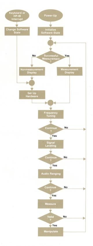
**Fig. 1.** 8901A software supervisory loop is continuously traversed by the microprocessor-based controller. A measurement is made near the bottom only if all preceding tests are passed in immediate succession.
