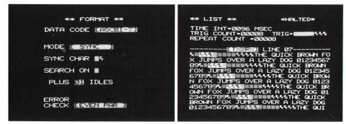
**Fig. 2.** (Left) Typical menu shows the selections to be made, in this case the format for configuring the instrument to match the format of the data in the RS-232C bus. The blinking cursor is positioned here in the DATA CODE field. **Fig. 3.** (Right) In the LIST mode, the contents of the data-acquisition memory are displayed with RX data (inverse video) interleaved with TX data (normal video).
