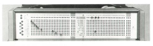
memory can be displayed at one time but the rest can be brought on display by using the up-down CURSOR keys to scroll the data past the display.
