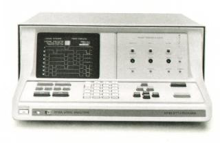
**Fig. 2.** Model 1615A Logic Analyzer can function as a 24-bit state analyzer, an 8-bit timing analyzer with glitch triggering capability, or as a combination 16-bit state and 8-bit timing analyzer that captures time and state activity simultaneously. Cross triggering between timing and state modes enables study of the interaction between timing problems and particular states, especially useful where the system under test has both synchronous and asynchronous elements.
