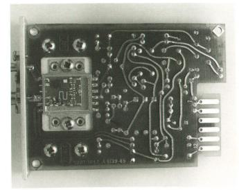
**Fig. 8.** Thin-film sampler is housed in a low-cost stripline package mounted to the printed-circuit board containing the preamplifier circuits.
