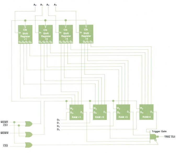
Fig. 8. Scaled-down representation of the trigger recognition circuitry.
