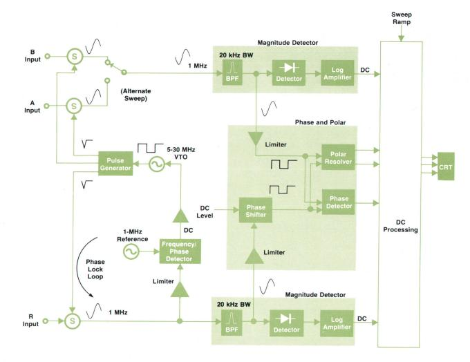
**Fig. 9.** Three-input receiver has a reference channel (*R*) for phase and magnitude-ratio measurements and a time-shared channel. The alternate sweep switch allows two quantities, applied through the A and B inputs, to be displayed simultaneously. All three inputs are down-converted by samplers serving as mixers.
