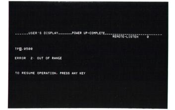
**Fig. 5.** When an illegal command is sent over the HP-IB to Model 1610A/B, the analyzer displays an error message. In the one shown here, number 3 is the highest value that can follow the mnemonic TP (trace point).
