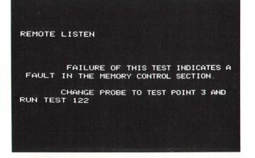
**Fig. 7.** Automatic test programs for controlling a logic analyzer over the HP-IB can include messages that are displayed on the analyzer's CRT for the test technician.
