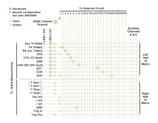
Fig. 5. Organization of the pin matrix. The 24 leads of the RS-232C bus form the vertical columns and the 1640A inputs/ outputs form the horizontal rows. For clarity, the left half of the matrix is shown stacked on the right half.
