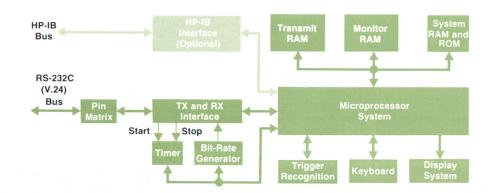
Fig. 7. Simplified block diagram of Model 1640A. It is microprocessor-based (8080-4), which enables it to perform a wide variety of measurements without a lot of software.
