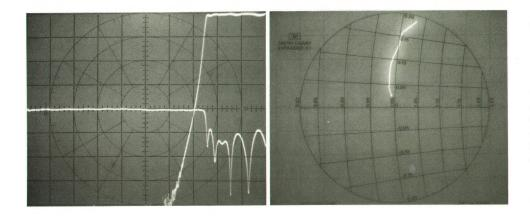
**Fig. 3.** Display at left shows the transmission characteristics of a 1-GHz high-pass filter measured over a frequency range of 4 to 1300 MHz by Model 8754A. The vertical scale is 10 dB/div. The display at right was made in the polar mode with a Smith chart overlay installed on the CRT. This shows the input impedance of a transistor amplifier to be near  $50\Omega$  at low frequencies, becoming increasingly inductive at the higher end of the 4-to-1300-MHz measurement range.
