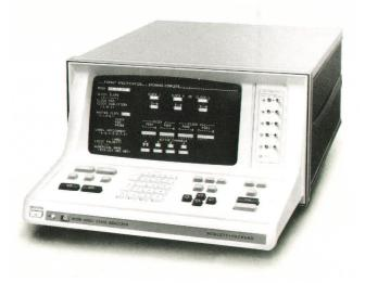
**Fig. 1.** Model 1610A/B Logic State Analyzer traces the flow of simultaneous digital events in as many as 32 bus lines in digital systems at clock rates up to 10 MHz. Its selective triggering capabilities enable it to restrict data capture to specific loops or branches in complex programs. Keyboard control and an interactive display that uses menus enable rapid set up of complex measurement parameters. The Model 1610B shown here can have data strobed in by three different clocks.
