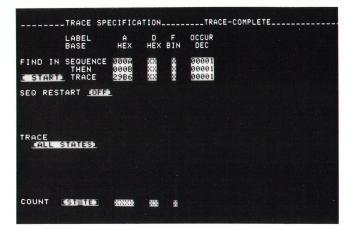
**Fig. 3.** Menus display fields (highlighted by inverse video) that may be changed by the keyboard in setting up instrument controls. The menu shown here tells the analyzer it must first find state 000A and then 000B in that order before allowing state 29B6 to start data capture.
