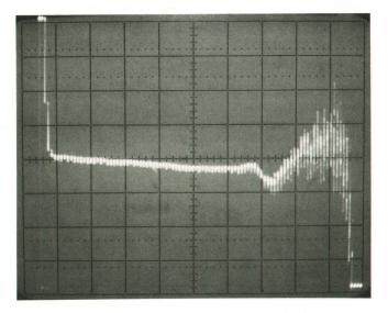
**Fig. 13.** Oscilloscope display of magnitude detector error versus signal level over a range of +10 dBm (left) to -90 dBm (right). The error voltage is derived by comparing the detector output to a reference. This measurement, which shows the accuracy of the magnitude detectors, was made on a sweeping-attenuator test system developed for the 8754A production line. (Vertical scale: 0.25 dB/div.)
