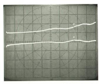
**Fig. 10.** Wide 4-to-1300-MHz-sweep display of magnitude (upper trace, 0.25 dB/div) and phase (lower trace, 2.5°/div) shows no transients where the four frequency relock points occur. The tunable marker is positioned at 1 GHz.
