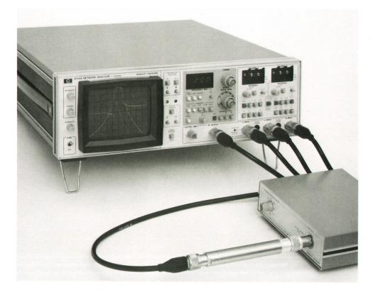
**Fig. 1.** Model 8754A Network Analyzer makes swept measurements of absolute power, gain/ loss, phase, and reflection coefficient over a frequency range of 4 to 1300 MHz. Dual-channel operation permits display of two parameters simultaneously in the rectilinear display mode, or magnitude and phase angle in the polar display mode.
