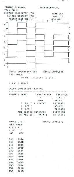
**Fig. 6.** Timing plots and labels can be sent from Model 1615A over the HP-IB to a digital plotter.
