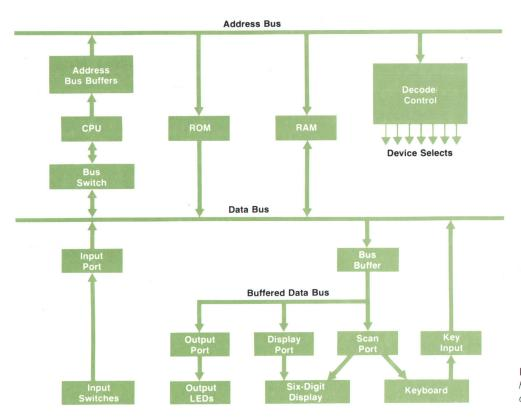
Shorted address bus lines Bad ROM output line Stuck ALE control signal Bad RAM decoding Bad address decoder Bad memory protect circuit Stuck Ready line Stuck Hold line Broken buffered data bus line Shorted buffered data bus line Open keyboard scan line Shorted keyboard/display lines.
