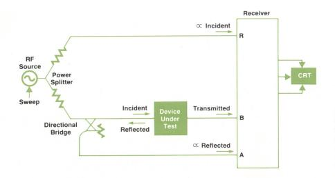
**Fig. 2.** Basic network analyzer measures device characteristics by comparing the signal entering the device (incident) with the signals leaving the device (reflected or transmitted) and displaying the difference in dB or degrees.
