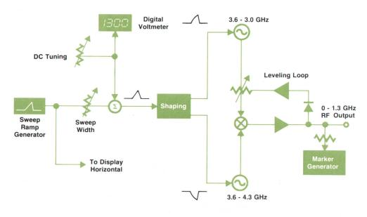
**Fig. 6.** The RF output is a difference frequency derived from the two varactor-tuned microwave oscillators.
