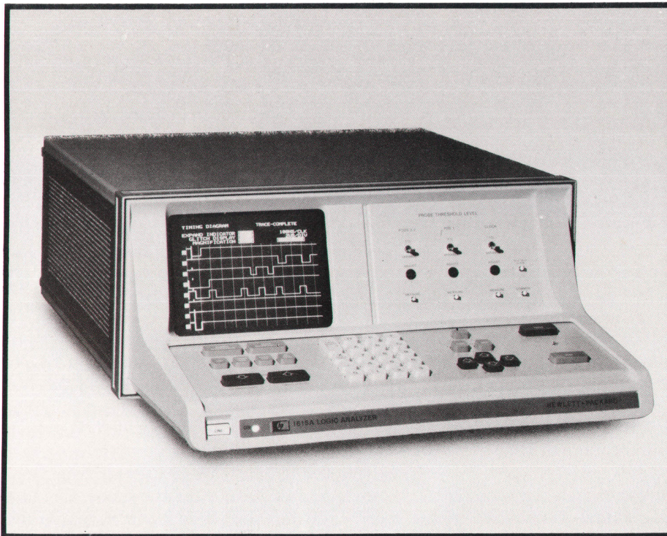
Fig. 2. Model 1615A Logic Analyzer functions as both a logic state analyzer and a logic timing analyzer. The state analyzer part of the instrument can trigger the timing analyzer so timing problems related to a particular part of a program can be located. Conversely, the timing analyzer can trigger the state analyzer so state information related to a timing event can be observed.
