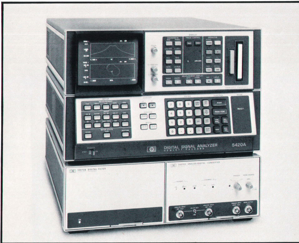
Fig. 1. Model 5420A Digital Signal Analyzer is a dual-channel instrument that analyzes signals in the dc-to-25-kHz frequency range. It makes many powerful time and frequency domain measurements, including spectrum, transfer function, and impulse response. Results are displayed on a fully annotated dual-trace CRT in any of three graphic formats and 14 choices of coordinates.
