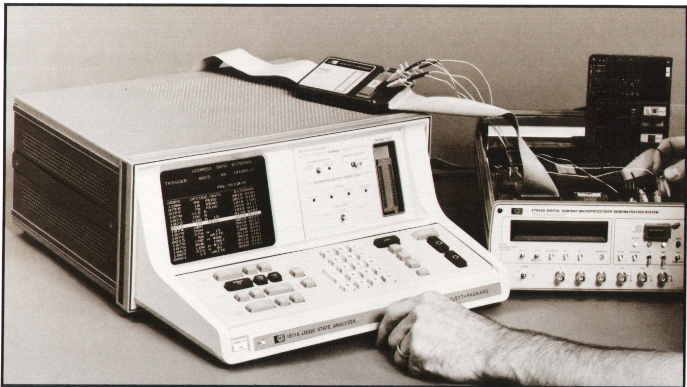
Fig. 1. Model 1611A Logic State Analyzer, designed to test systems using popular microprocessors, captures and displays the sequential flow of states on a microprocessor's DATA and ADDRESS busses and at up to eight other nodes selected by the user.
