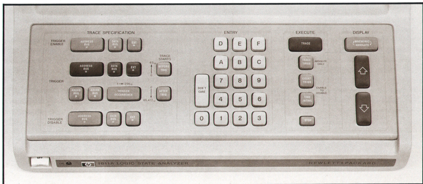
Fig. 1. Keys are grouped into four functional areas on the keyboard of the Model 1611A Logic State Analyzer. The keys that are most basic to instrument operation are in a darker shade.
