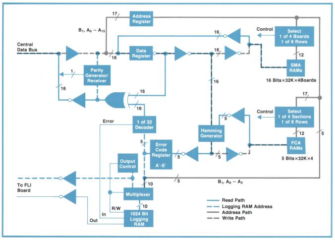
**Fig. 4.** Check bit field generation takes place in three memory-module boards: MCL, FCA, and the accessed SMA board. The Hamming generator on the FCA board does the calculations. Four check bits are stored on the FCA board and one on the SMA.
