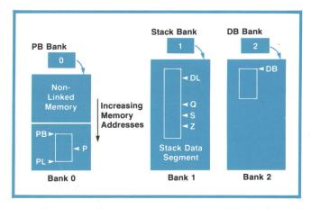
**Fig. 3.** Modified register structure of the HP 3000 Series II. Memory is divided into four banks of up to 64K words each. Three bank registers (shown at top) allow code and data segments in different banks to be used simultaneously.
