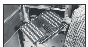
**Fig. 1.** 136 18-pin 4K RAMs on each HP 3000 Series II memory board provide 32,768 17-bit words of semiconductor memory capacity, four times the capacity of the same-size board with core memory. Series II memory is 50% faster and less than one-third as costly as the older core memory.
