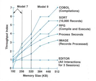
**Fig. 1.** Relative throughput of HP 3000 Series II models 7 and 9 using several measures of throughput. The base is a model 5 system with 128K-byte memory. magnetic tape that is later processed by data reduction programs.
