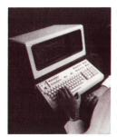
**Cover:** Model 2640A Interactive display terminal uses its optional line-drawing character set to display a form to be filled in by the operator. Microprocessor control gives this new terminal a high degree of flexibility at a relatively low cost.
