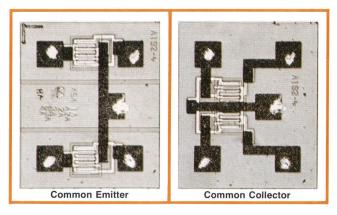
**Fig. 6.** Special dual-transistor chips, made by a new 5-GHz transistor process, are used in the high-speed binary in the 1100-MHz front end.
