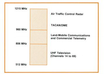
**Fig. 2.** Frequency spectrum allocations within the range of the 1100-MHz counter.
