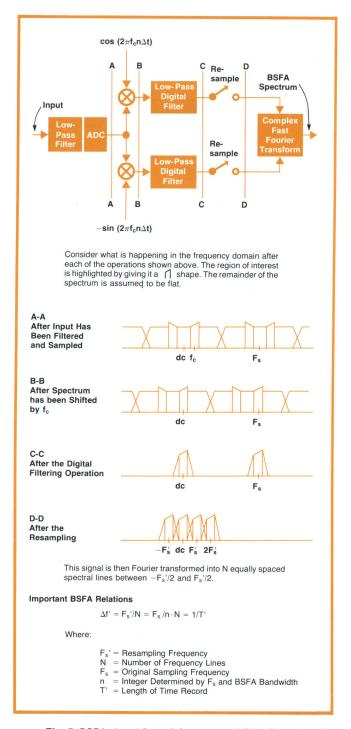
**Fig. 5.** BSFA signal flow. A frequency shift by f<sub>c</sub> centers the analysis band on the frequency of interest and digital filtering removes information outside the band of interest.
