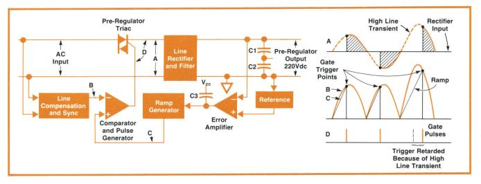
**Fig. 5.** Block diagram of the preregulator section. Operation is explained by the waveforms, which also show how the preregulator responds immediately to a change in line voltage.
