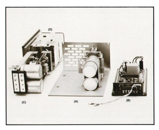
**Fig. 4.** Modular construction simplifies assembly and disassembly.
