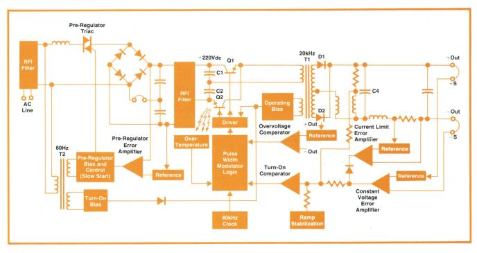
**Fig. 2.** Block diagram of the Model 62605M modular power supply. It operates directly from a 220V power line when the shorting strap is in place. With the strap removed (and some other minor changes), the input rectifiers no longer function as a bridge but become a voltage doubler that enables use on a 120V line.
