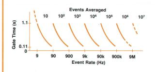
clocked on the next log pulse. The log time base produces pulses when 10 events have occurred, and when 10<sup>2</sup>, 10<sup>3</sup>,..., 10<sup>7</sup>, 10<sup>8</sup> events have occurred. The first of these pulses to occur after 0.11 s has elapsed will close the gate. Because the pulses represent powers of ten of the event rate, some pulse will close the gate after it has been open for a time between 0.11 and 1.1 s.
