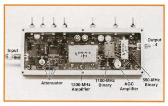
**Fig. 3.** Completely enclosed high-frequency front end contains an attenuator, a broadband amplifier, a high-speed binary, and a second binary.
