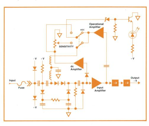
**Fig. 5.** Input attenuator may be controlled manually or automatically. Usually automatic sensitivity control is better for noisy signals; manual control is better for amplitude-modulated signals.
