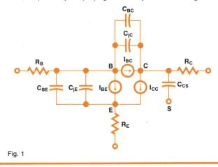
C<sub>iC</sub>, C<sub>iE</sub>, and C<sub>CS</sub> reduced propagation delay by 5% or less.
