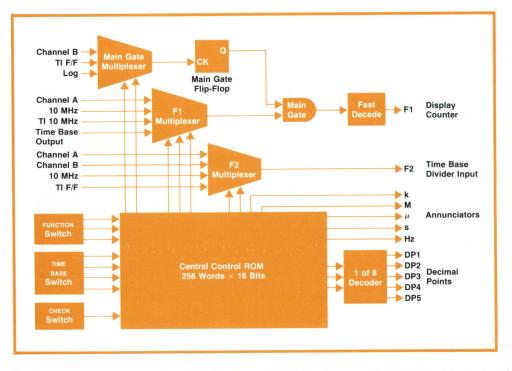
**Fig. 2.** 5308A function control circuit. Central control ROM made possible much of the new capability of the 5308A, including autoranging and time interval averaging.
