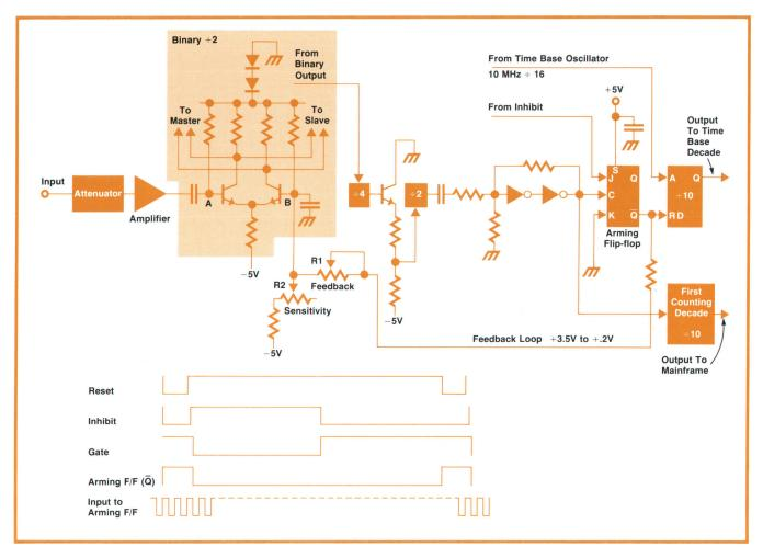
**Fig. 8.** Feedback loop reduces input sensitivity until a large enough input signal is present, then increases sensitivity during counting.
