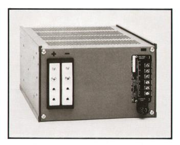
**Fig. 1.** Model 62605M Power Supply, designed for permanent installation, supplies current in a range from 0 to 100 A at 5 V. The switching regulator achieves 70% efficiency at full output.
