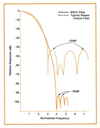
**Fig. 6.** BSFA digital filters have high out-of-band rejection, a primary requirement for BSFA. Here the BSFA filter frequency response is compared with a commonly used raised cosine filter. Note the 50 dB greater out-of-band rejection of the BSFA filter.
