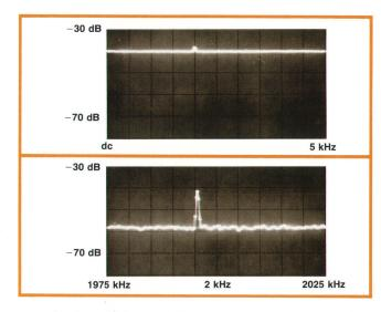
**Fig. 2.** In the baseband spectrum of a sine wave buried in white noise the sine wave appears only 2 dB above the noise after 10 000 averages. In the BSFA spectrum after only 100 averages, the sine wave is 17 dB above the noise and consequently is much more detectable. BSFA's 100 × improvement in resolution results in a reduced mean value for the white noise; however, the noise variance is greater because fewer measurements were averaged. The two measurements required the same total time.
