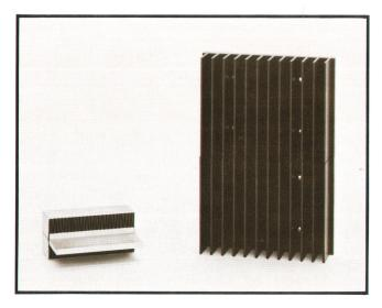
**Fig. 3.** Heat is removed from the power mesh through a heat exchanger (left) that rises in temperature only 0.5°C/W with an air flow of 10 ft<sup>3</sup>/s. An equivalent convection-cooled heat sink is shown on the right.
