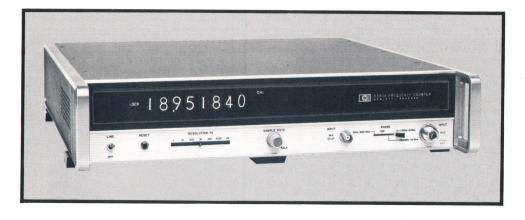
Fig. 1. Model 5340A Microwave Frequency Counter can measure 10 Hz to 18 GHz automatically, using only a single input. Eight digits are displayed. Resolution is selectable from 1 Hz to 1 MHz.
