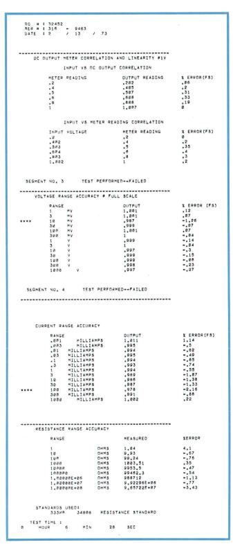
**Fig. 3.** Typical 9550 test report shows failure points (\*\*\*\*) and running time.
