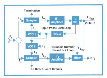
**Fig. 5.** Wideband thin-film samplers are used as harmonic mixers in the automatic transfer oscillator phase-lock loops. The input loop mixes the signal with a harmonic of the sampling frequency. The second loop determines the harmonic number.
