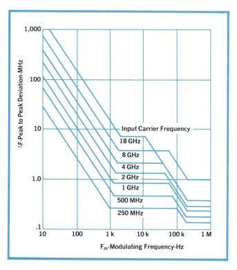
**Fig. 6.** Typical 5340A frequency modulation tolerance characteristics for single-tone FM on input signal. Input level is -20 dBm. Carrier frequency will be correctly measured if modulation frequency and peak-to-peak deviation are below curves.
