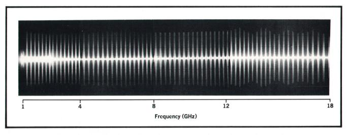
**Fig. 5.** In swept tests, the sampler produces a response whenever its output frequency is in the passband of the IF amplifier shown in Fig. 3. Note uniformity of responses.
