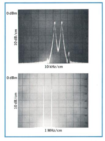
**Fig. 9.** Model 5340A is designed to measure only the largest signal in its passband. Top spectrum is of signals 10 kHz apart and differing in amplitude by 1 dB. In bottom spectrum, signals are 1 MHz apart and differ by 3 dB. The larger signal in each case was measured.
