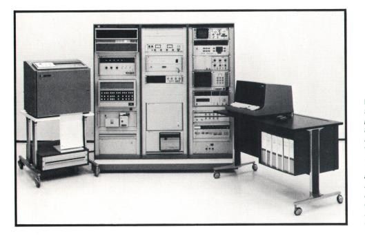
Fig. 1. 9550 Instrument Calibration Systems are modular computer-controlled dedicated systems designed to help solve calibration laboratory problems of work overload, personnel training, and laboratory management. Large and small systems are available. Calibration-quality stimulus and measuring instruments, plus computer-applied corrections, assure that automated calibrations equal or exceed manual methods.
