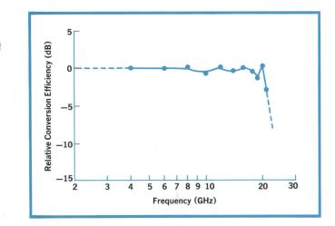
Fig. 4. Relative conversion efficiency of thin-film sampler.
