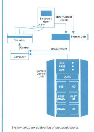
Watching the needle deflection, he presses the appropriate button to provide more or less stimulus voltage and quickly adjusts the stimulus so the needle deflection is exactly over the 0.1 cardinal point. He then presses the "DONE" button on the remote controller. The system measures and records the voltage at the 412A meter output jack (proportional to meter deflection).\* The system also records the true dc voltage required at the input of the instrument to deflect the needle to the 0.1 point.
