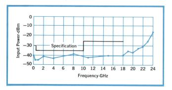
Fig. 2. Typical 5340A sensitivity.
