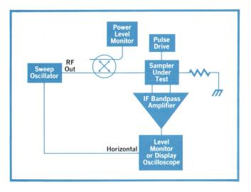
Fig. 3. Typical circuit used for testing sampler operation (conversion efficiency, IF response, etc.).
