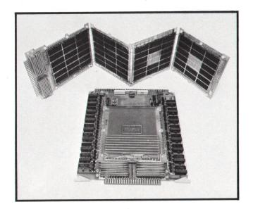
Fig. 2. 8K folded-planar corestack with sense amplifiers and diode decoding matrix occupy only one printedcircuit board. Cores are 20-mil wide-temperature-range type.
