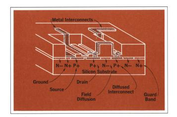
**Fig. 5.** Extra N + diffusion next to P + source, and extra N + guard band, are elements of a unique 'ground riveting' scheme that was used to eliminate much ground metallization. This reduced the sizes of the MOS chips and allowed 10 MHz speeds.
