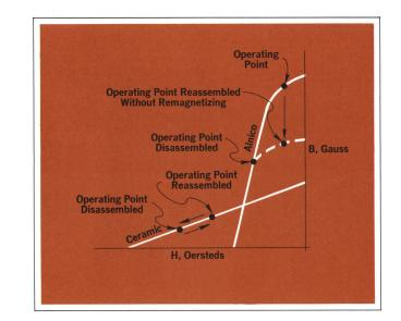
**Fig. 5.** What happens when a magnetic assembly is disassembled then reassembled. Operating point of alnico drops, while the operating point of a ceramic magnet assembly is the same when reassembled; remagnetizing is unnecessary.
