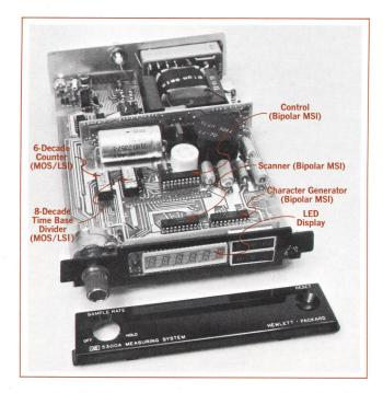
**Fig. 3.** Mainframe contains a complete six-digit 10 MHz electronic counter except for an input amplifier and trigger. Large-scale and medium-scale integration and a solid-state display reduce the six major blocks in Fig. 2 to just six components. Benefits are reliability, service-ability, and low power consumption.
