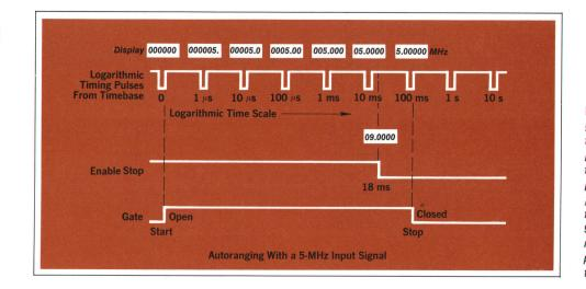
**Fig. 6.** Autoranging selects the gate time for maximum resolution without overflowing the display. A logarithmic output from the time-base chip produces pulses at decade multiples of 1  $\mu$ s. The counter counts until the fifth decade reaches a count of 9, then terminates the measurement on the next logarithmic pulse. Manually-selected gate times are also available.
