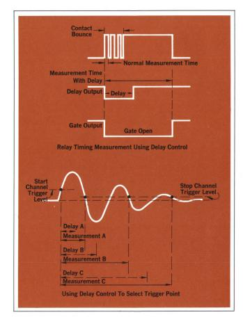
**Fig. 8.** Model 5304A Timer/Counter snap-on module is optimized for time-interval measurements. It has 100-ns resolution and an unusual delay feature which causes the counter to ignore extraneous events and measure the interval of interest. Delay is useful for relay timing and tone-burst measurements.
