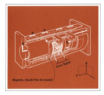
**Fig. 2.** Construction of the Hewlett-Packard linear motor. The linear motor positions a wiper on a potentiometer made of conductive epoxy film. The resulting position signal is compared to an applied input signal. The difference voltage between these signals is amplified and applied to drive the bobbin to reduce the error signal to a minimum.
