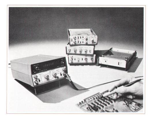
**Fig. 1.** Compact, low-cost 5300 Measuring System consists of a mainframe (top half of instrument at left), four snap-on functional modules, and a battery pack (right). Autoranging, serial BCD digital output, and a highstability crystal reference oscillator are standard.
