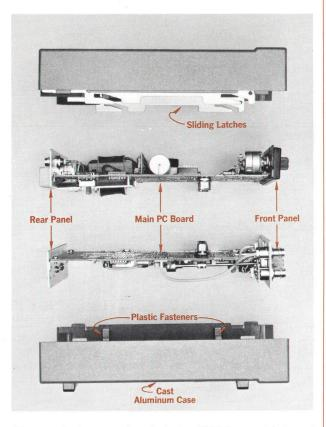
\*The cast aluminum case is a far better shield than most instrument cases. By itself, however, it isn't a complete RFI shield. Complete RFI shielding of the 5300A would require a metal screen behind the plastic front panel of the mainframe.
