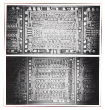
**Fig. 4.** 10 MHz MOS/LSI six-digit counter circuit and eight-decade time base chips. Counter chip (top) is 0.096 in by 0.118 in and contains 930 transistors. Time base is 0.109 in square and contains 980 transistors.
