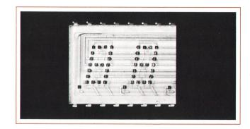
**Fig. 7.** Data comes out of the counter chip one digit at a time, so the solid-state display is scanned instead of continuously lighted. One-half digit is lighted at a time. A scan is completed every millisecond, so the display appears steady.
