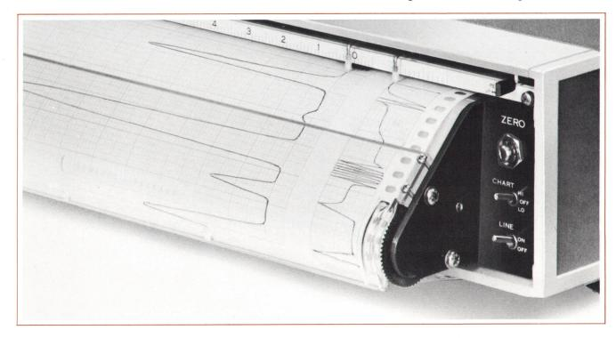
**Fig. 6.** An all-electronic integrator used for measuring the areas under the main trace is an option with the Model 7123A/B recorders. Its separate pen shares the slider rod and magnetic circuit of the linear motor with the main pen assembly.
