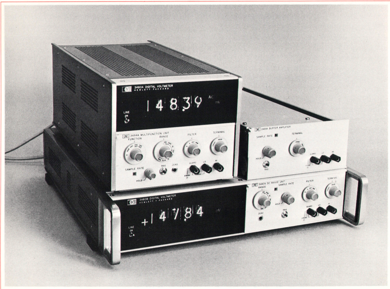
Fig. 1. This new Hewlett-Packard Model 3480A/B is a high speed multi-function DVM capable of making 1000 readings per second up to 1000 volts dc, and ohms down to 100 ohms full scale. It comes in both half module and rack versions. Also shown here are the Models 3481A Buffer Amplifier (with one 10 V dc range), 3482A DC Range Unit and the 3484A Multifunction Unit.
