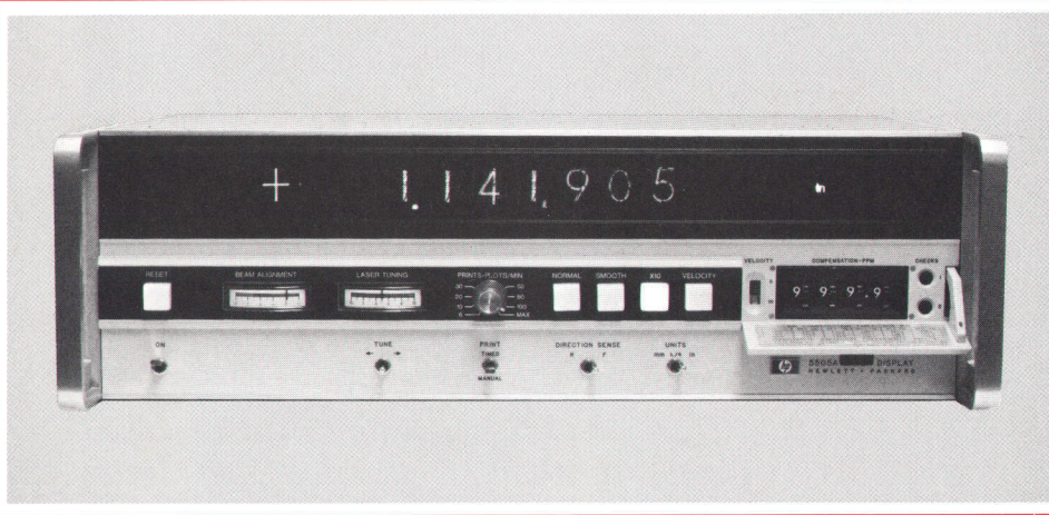
Fig. 2. Model 5525A Interferometer has 10 microinch resolution in NORMAL and SMOOTH modes, one microinch in X 10 mode. In the SMOOTH mode, successive readings are averaged to eliminate vibration-induced jitter in the display. The system can also display the moving reflector's velocity, up to 720 in/min. Behind the door at right are thumbswitches for setting in velocity-of-light corrections.
