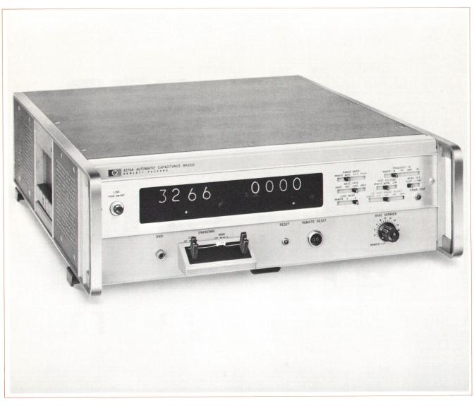
Fig. 1. The new HP Model 4270A Automatic Capacitance Bridge can measure grounded cables and input capacitance of amplifiers with the LOW terminal grounded. In L-GROUND operation, the instrument still retains the guarded feature.
