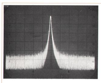
a  $I_{dc} = 55$  mA;  $P_o = 176$  mW  $f_o = 8.2$  GHz  $R_L = 1.0 \Omega$
