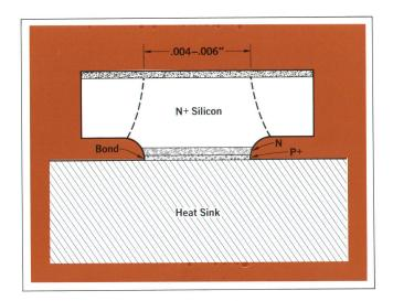
**Fig. 1.** IMPATT diode formed on silicon substrate and thermal-compression bonded to metal heat sink. Dotted lines show shape, mechanically more stable but harder to handle, obtained by etching from both sides of wafer. Dimensions apply to X-band diodes.
