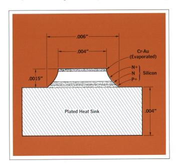
Fig. 2. Integral heat sink serves as water substrate during manufacture of new HP IMPATT diodes. Chips can be soldered into circuit or package without seriously degrading thermal properties.
