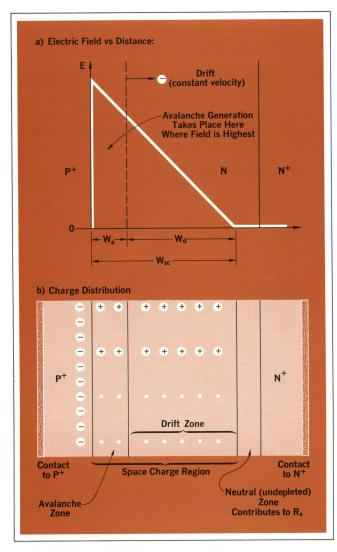
Fig. 4. Representation of diode with abrupt  $P^+NN^+$  junction reverse-biased in avalanche breakdown. Avalanche is generated in  $W_{\wedge}$  region where electric field is highest. Charge carriers move at constant velocity through drift region  $W_{d}$ .  $W_{sc}$  is total space charge region.
