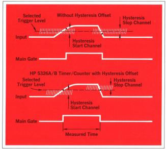
**Fig. 6.** Hysteresis keeps most counters from triggering exactly at the preset levels. Model 5326A/B's hysteresis offset has the same effect as reducing the hysteresis band by a factor of ten or more.
