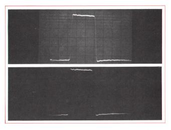
**Fig. 2.** Trace writing speed is increased by film and phosphor 'fogging' (upper trace) over speed obtained without fogging (lower trace), as shown by leading and trailing edges of fast pulse ( $t_r = 1.5$  ns). Internal flood gun in Model 183A Oscilloscope fogs film and phosphor automatically in synchronism with horizontal sweep.
