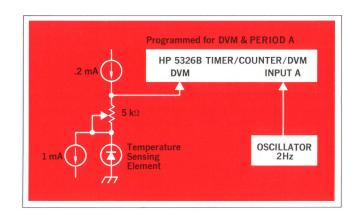
**Fig. 10.** Units conversion with Model 5326B. The temperature of the diode can be read directly in  $^{\circ}$ C with 0.1  $^{\circ}$ C resolution. The channel A input normalizes the reading.
