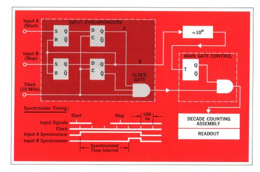
**Fig. 7.** Synchronizing circuit makes certain that a multipletime-interval average will tend towards the true value. In measuring 205 ns, for example, the counter will accumulate two counts 95% of the time and three counts 5% of the time, provided the repetition rate of the unknown intervals isn't synchronous with the 10 MHz clock.
