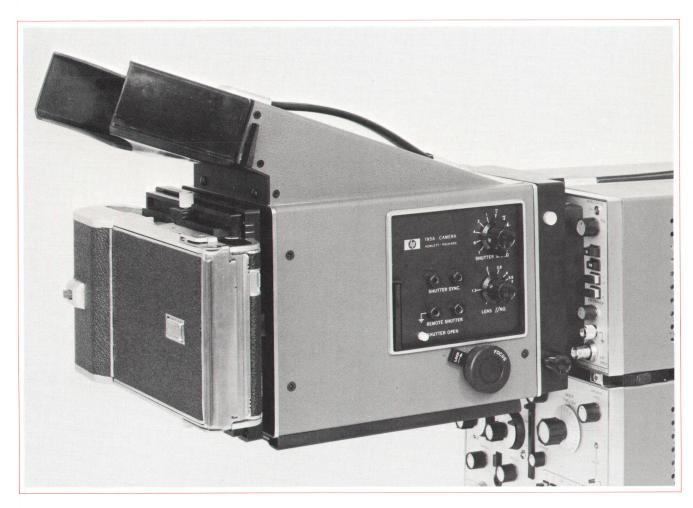
Fig. 1. Hewlett-Packard Model 195A Oscilloscope Camera mounts directly to HP 5-inch round and rectangular CRT bezels. Adapters, optionally available, fit Camera to most oscilloscopes of other manufacturers.
