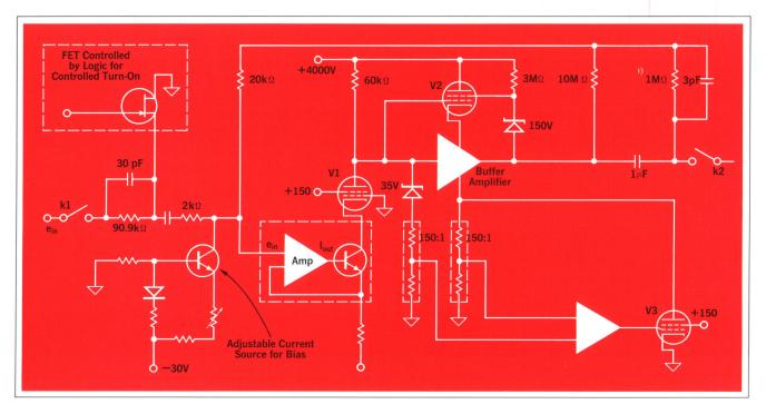
Fig. 3. Three vacuum tubes handle high voltage and power in the Model 746A. Logic circuitry controls the turn-on sequence.
