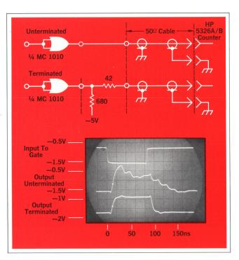
**Fig. 3.** Output of an ECL gate connected to Model 5326A Timer/Counter, first using only a  $50\Omega$  cable (middle trace) and then a  $50\Omega$  cable with the proper series termination. Reflections resulting from improper termination can cause double counts, incorrect readings.
